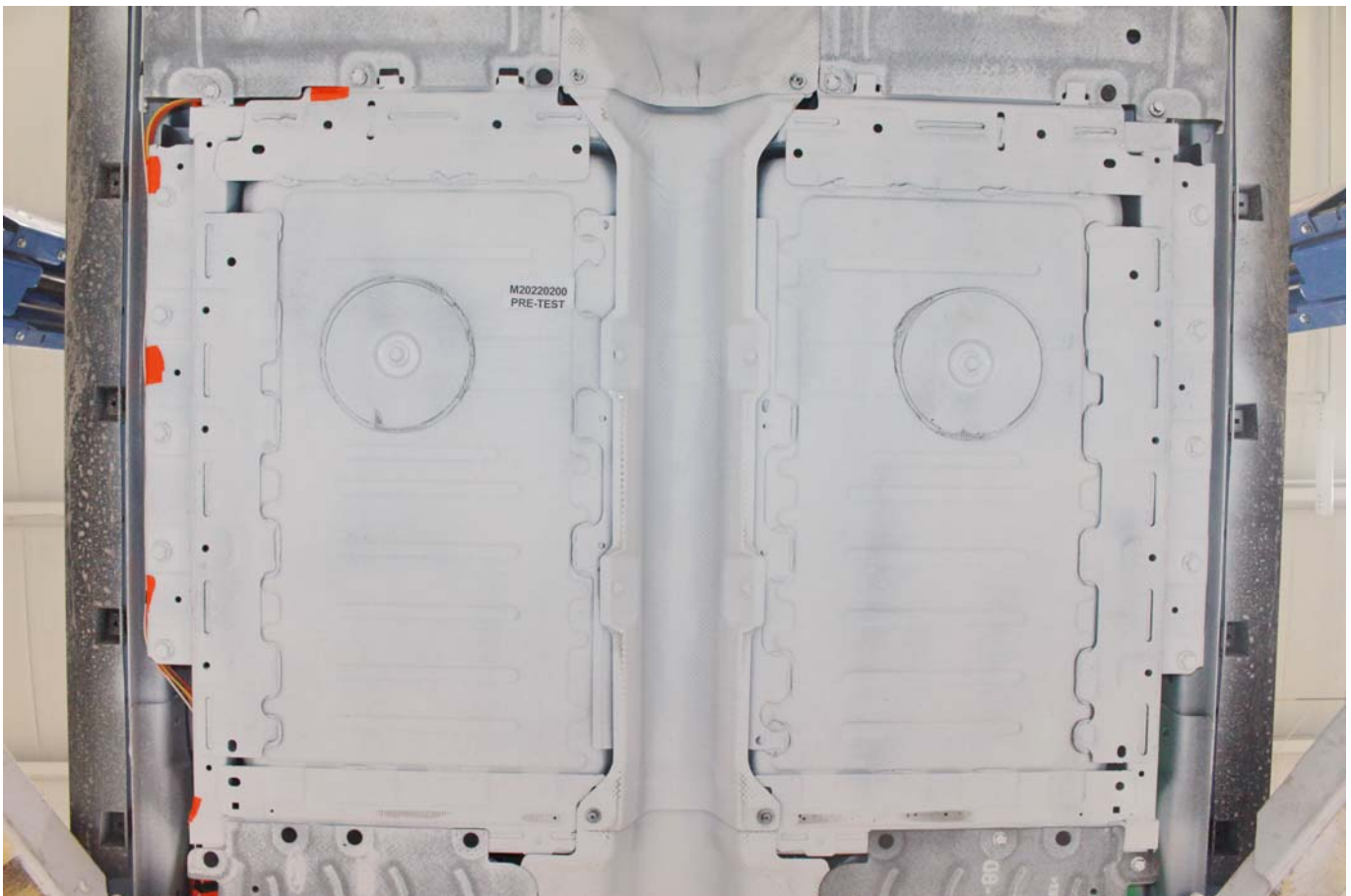
Photo No. 305-09 - Pre-Impact View of Propulsion Battery
