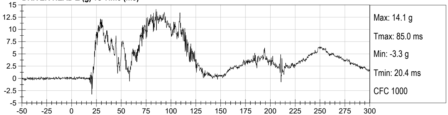
DRIVER HEAD Resultant (g) vs Time (ms)
