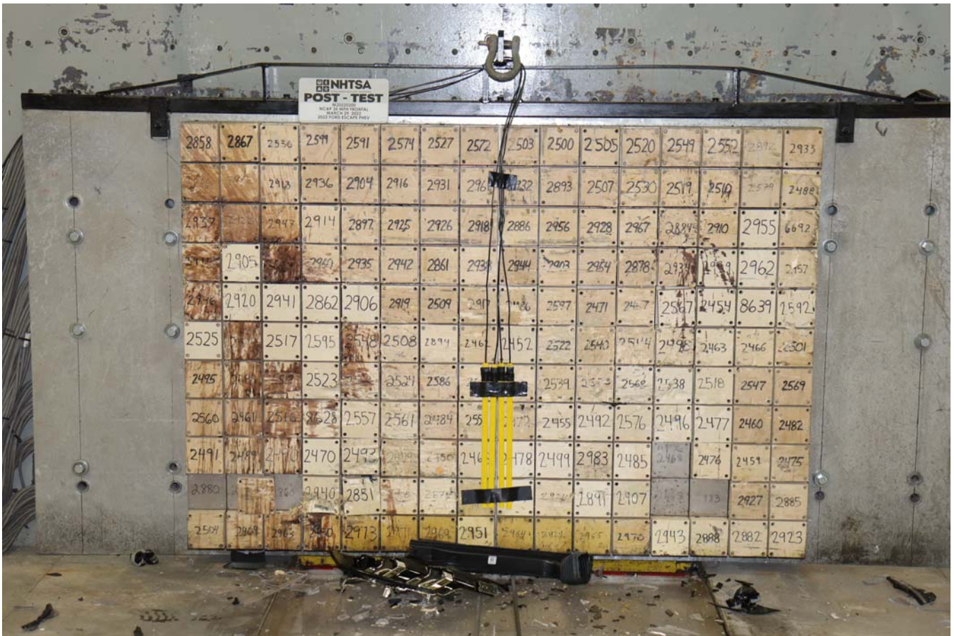
Photo No. 003 - Post-Test Load Cell Wall
