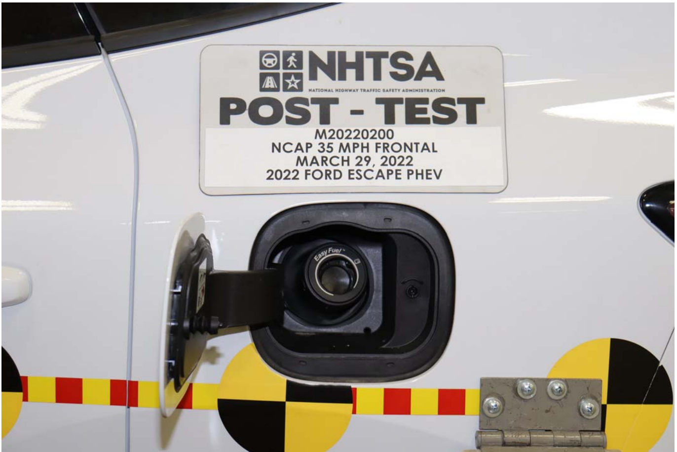
Photo No. 023 - Post-Test Fuel Filler Cap View
