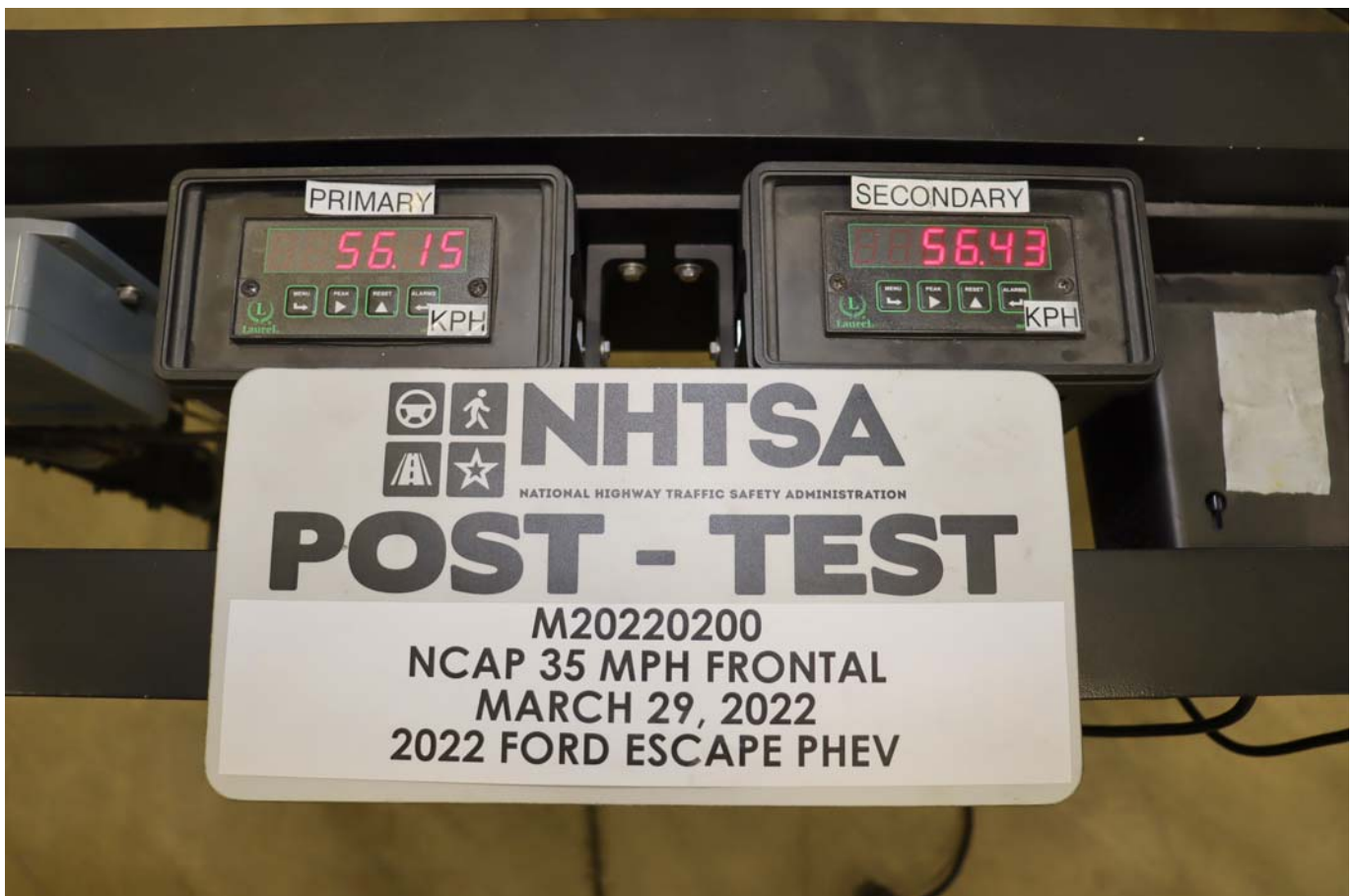
Photo No. 076 - Post-Test Speed Trap Read-Out
