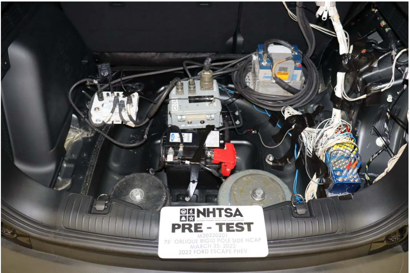
Photo No. 063 - Pre-Test Ballast View
