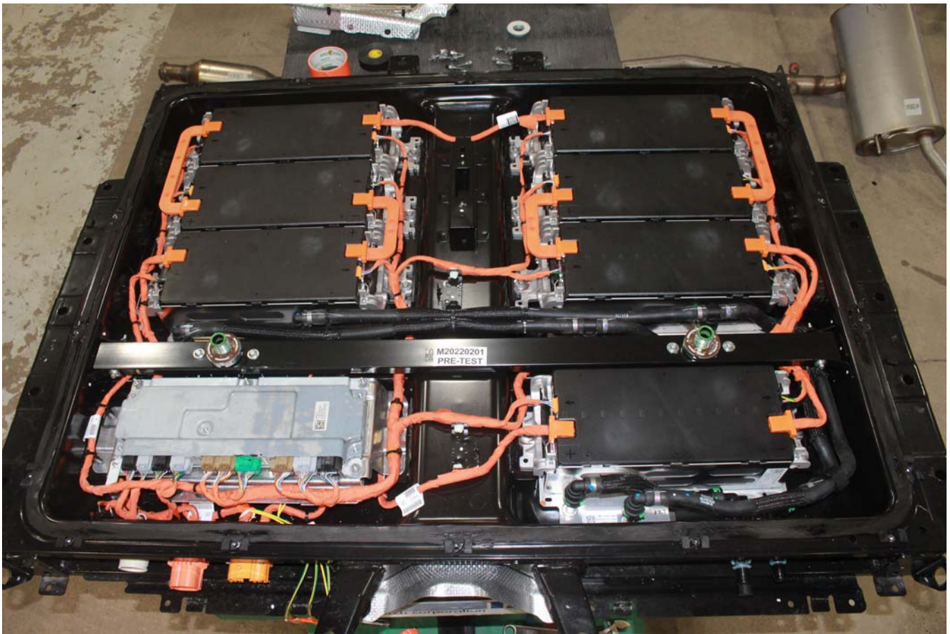
Photo No. 305-14 - Pre-Impact View of Propulsion Battery Module(s)
