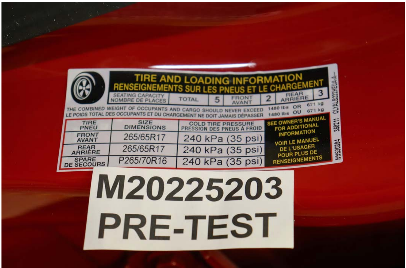
Photo No. 058 - Close-Up View of Vehicle's Tire Information Placard or Label
