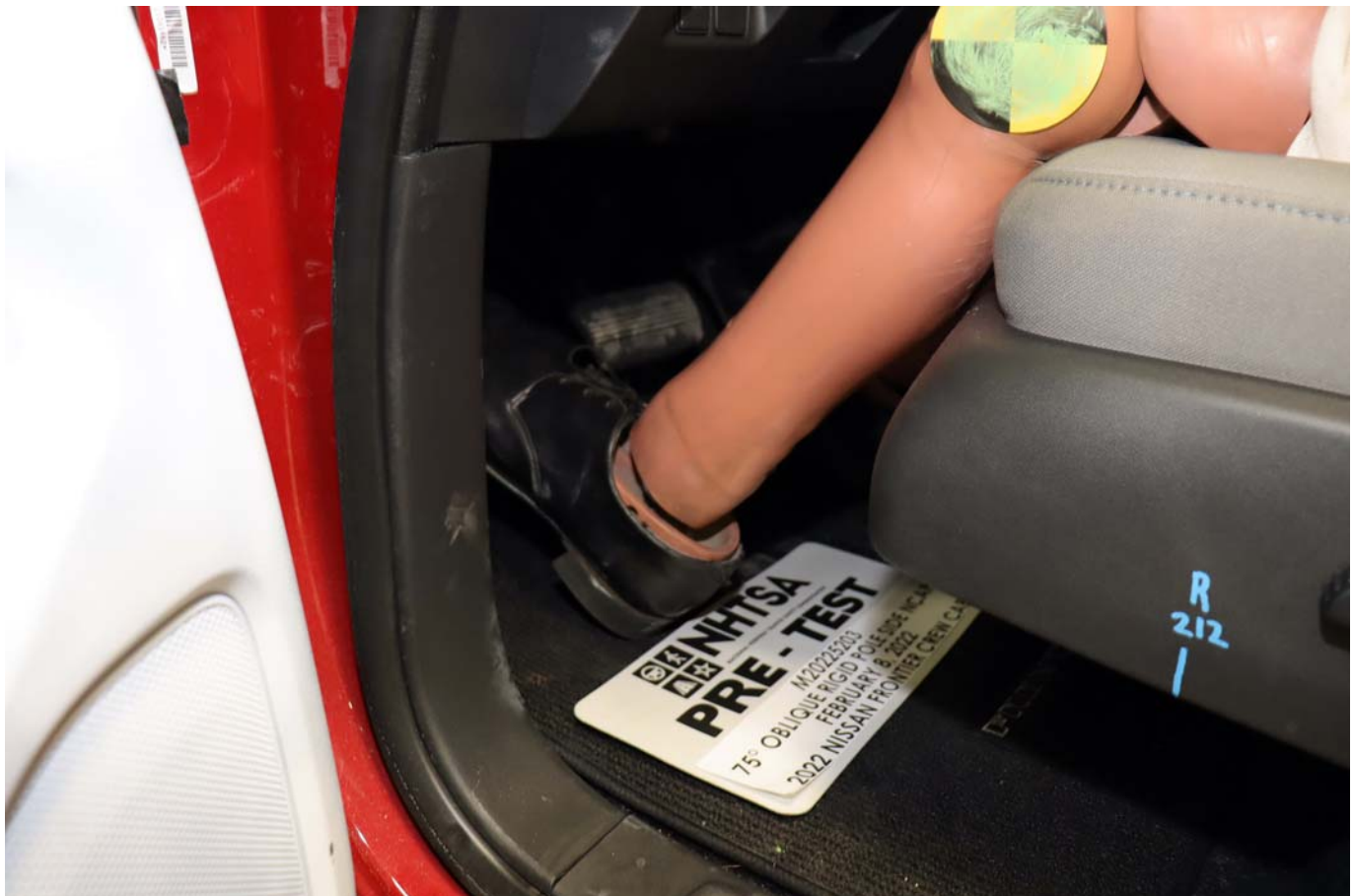
Photo No. 032 - Pre-Test Placement of Dummy's Feet
