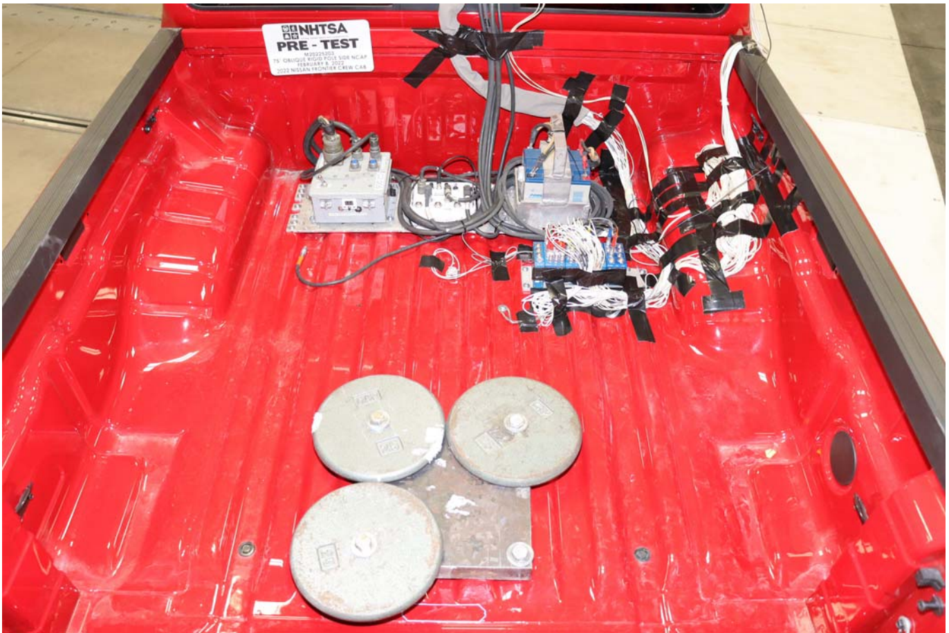
Photo No. 063 - Pre-Test Ballast View
