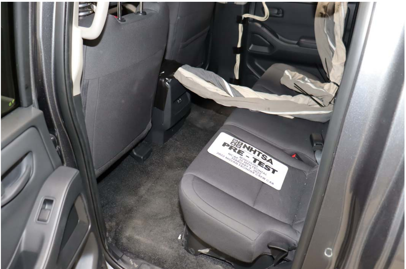
Photo No. 028 - Pre-Test Dummy Cable Routing
