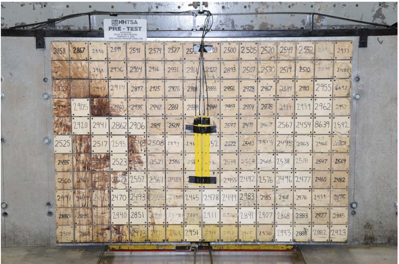
Photo No. 002 - Pre-Test Load Cell Wall
