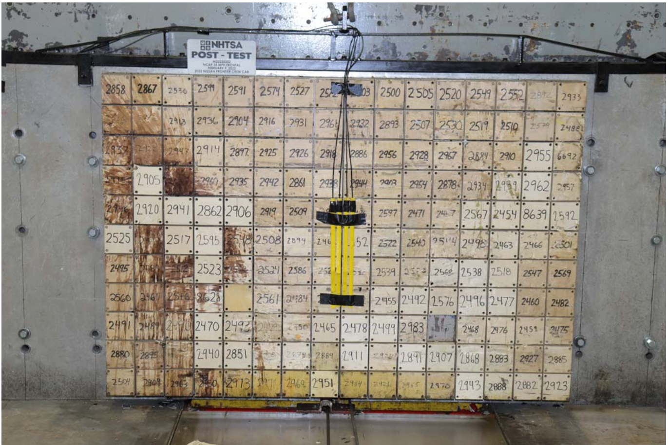
Photo No. 003 - Post-Test Load Cell Wall
