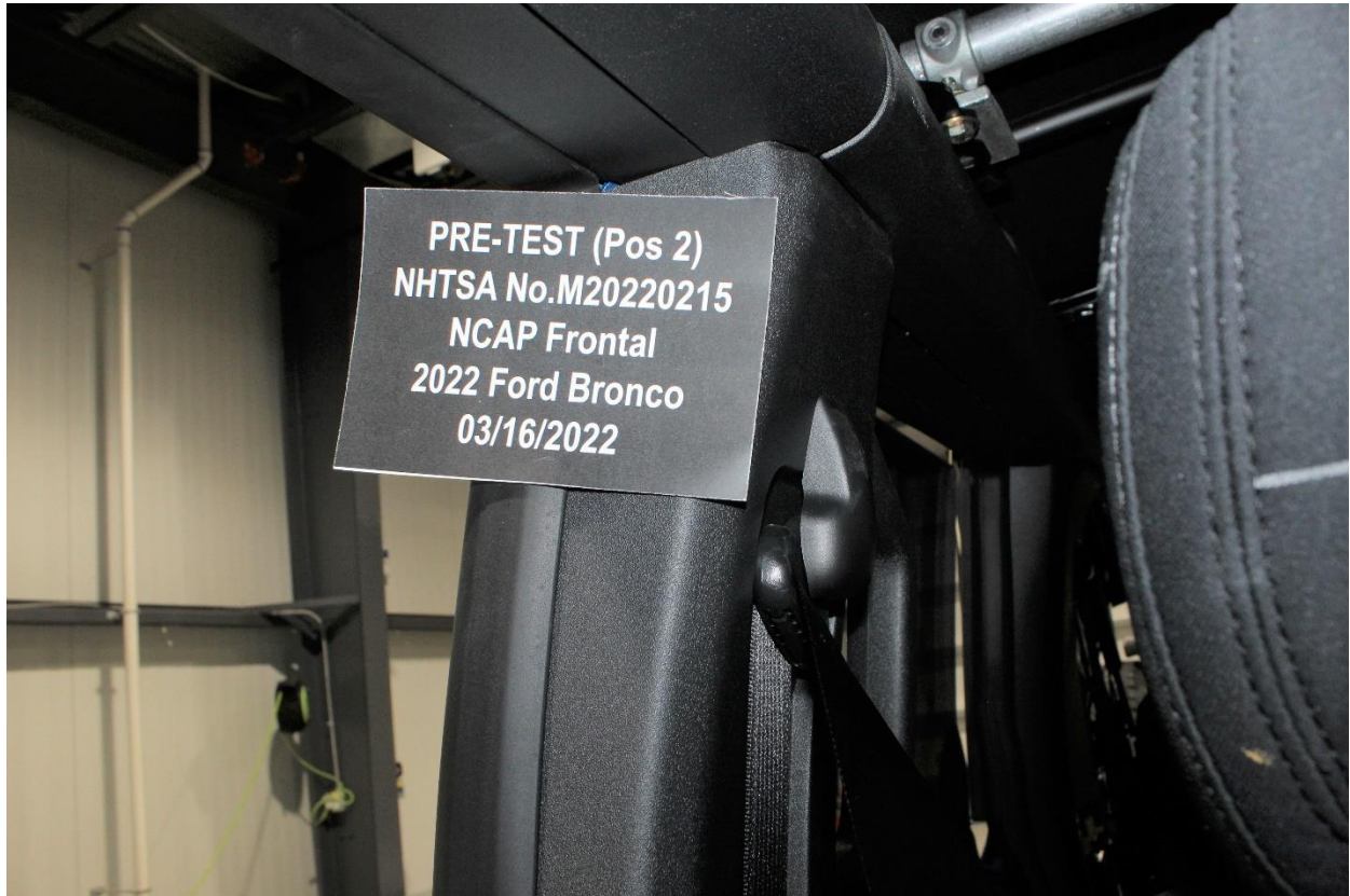
Figure A-61: Pre-Test View of Belt Anchorage for Passenger Dummy
