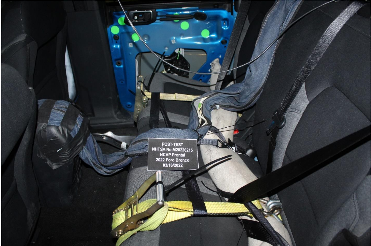
Figure A-29: Post-Test Dummy Cable Routing
