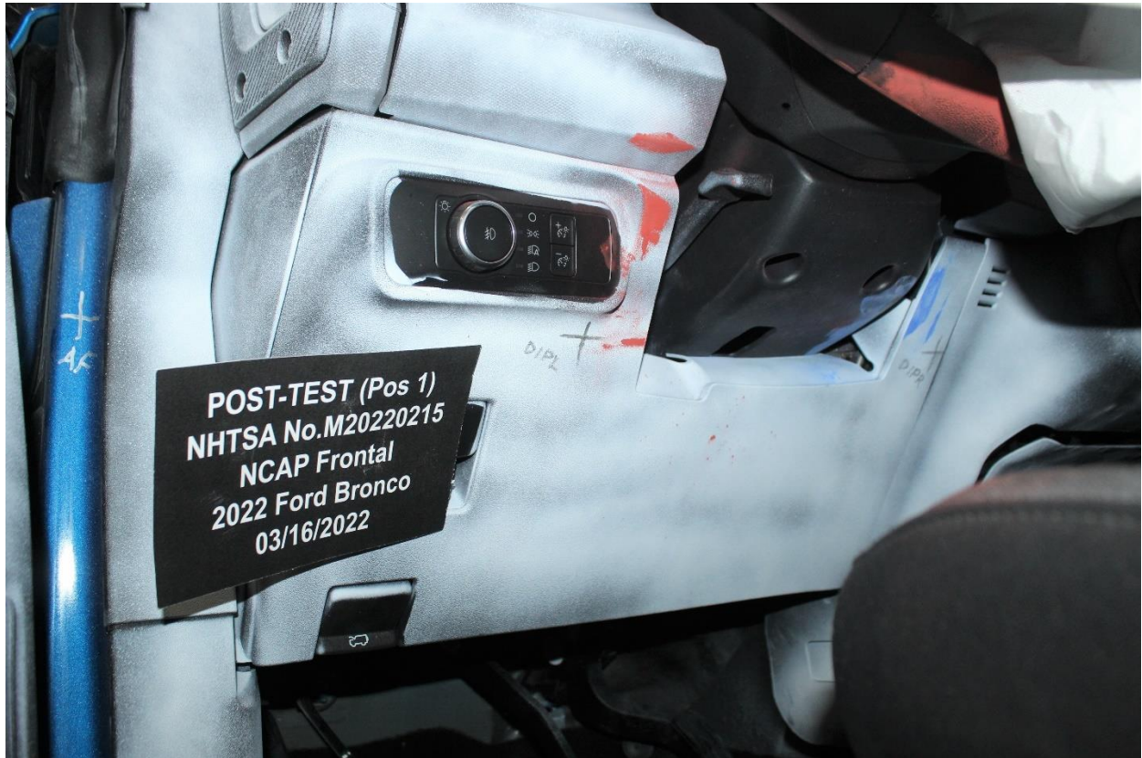
Figure A-45: Post-Test Driver's Side Knee Bolster
