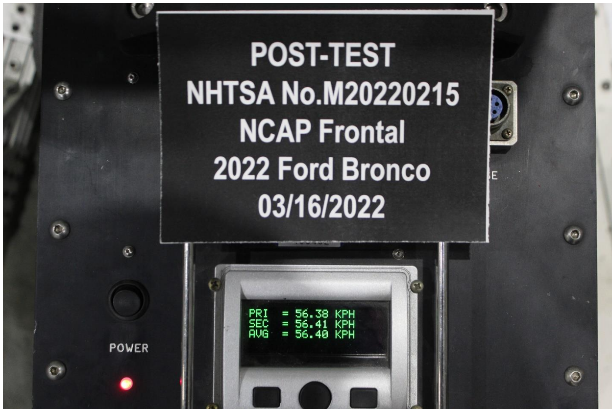
Figure A-76: Post-Test Speed Trap Read-Out
