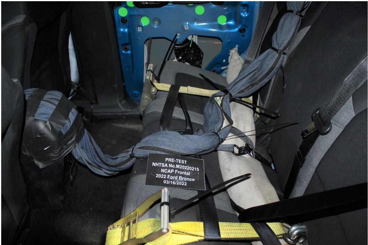
Figure A-28: Pre-Test Dummy Cable Routing
