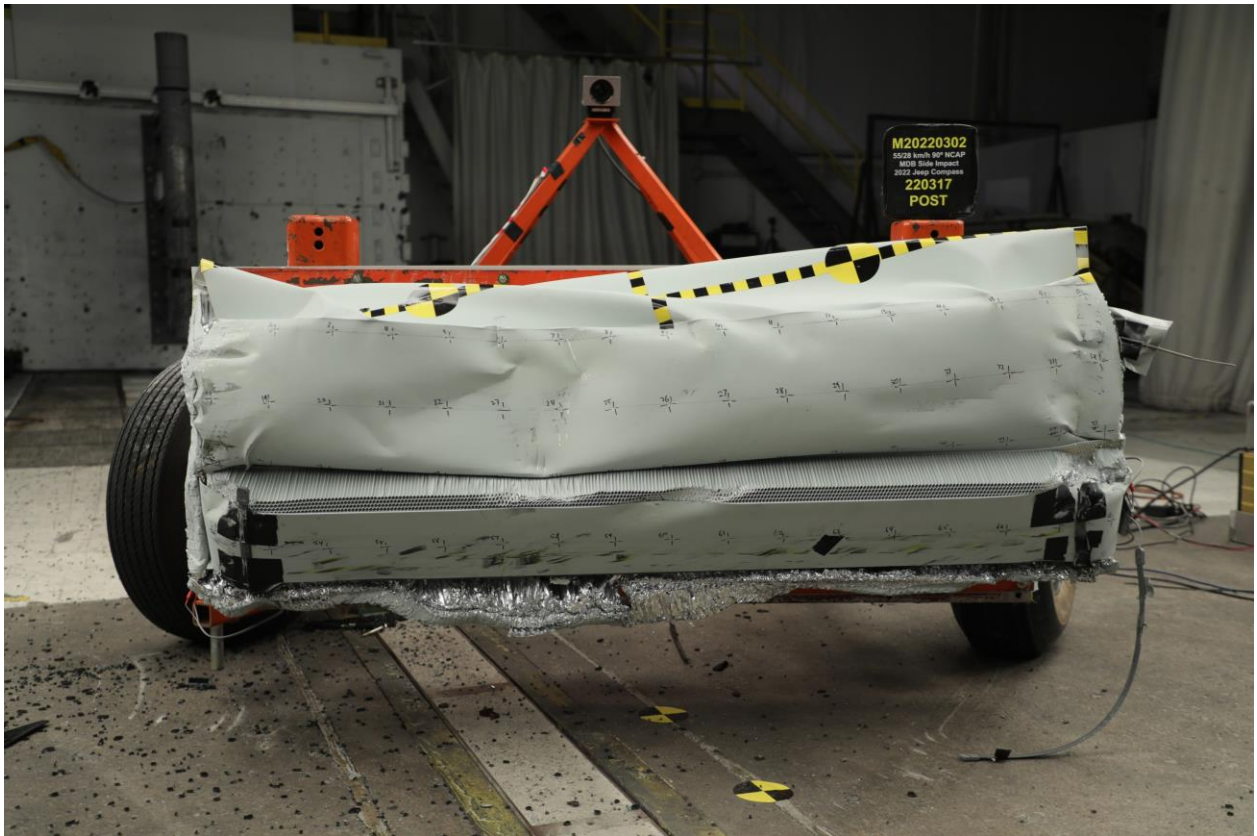
085 Post-Test Front View of MDB Impactor Face
