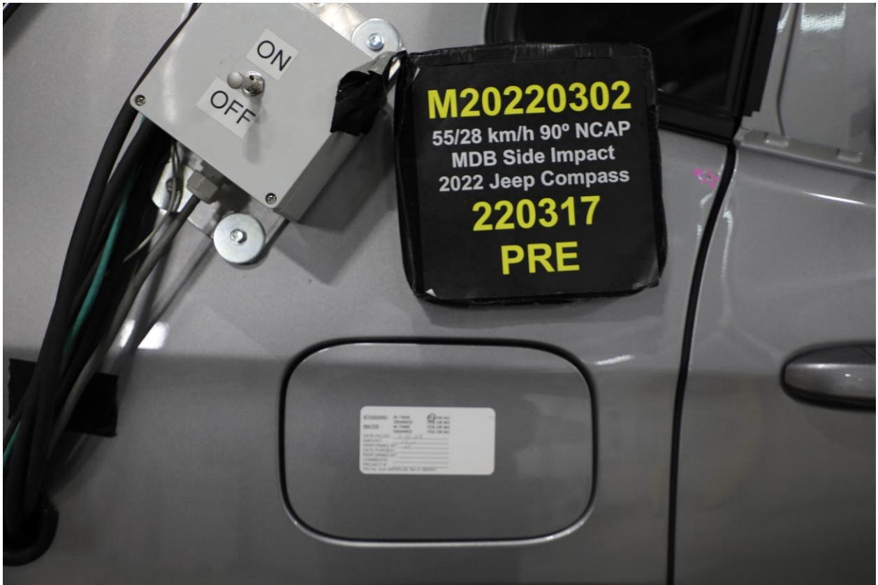
082 Pre-Test View of Fuel Filler Cap or Fuel Filler Neck
