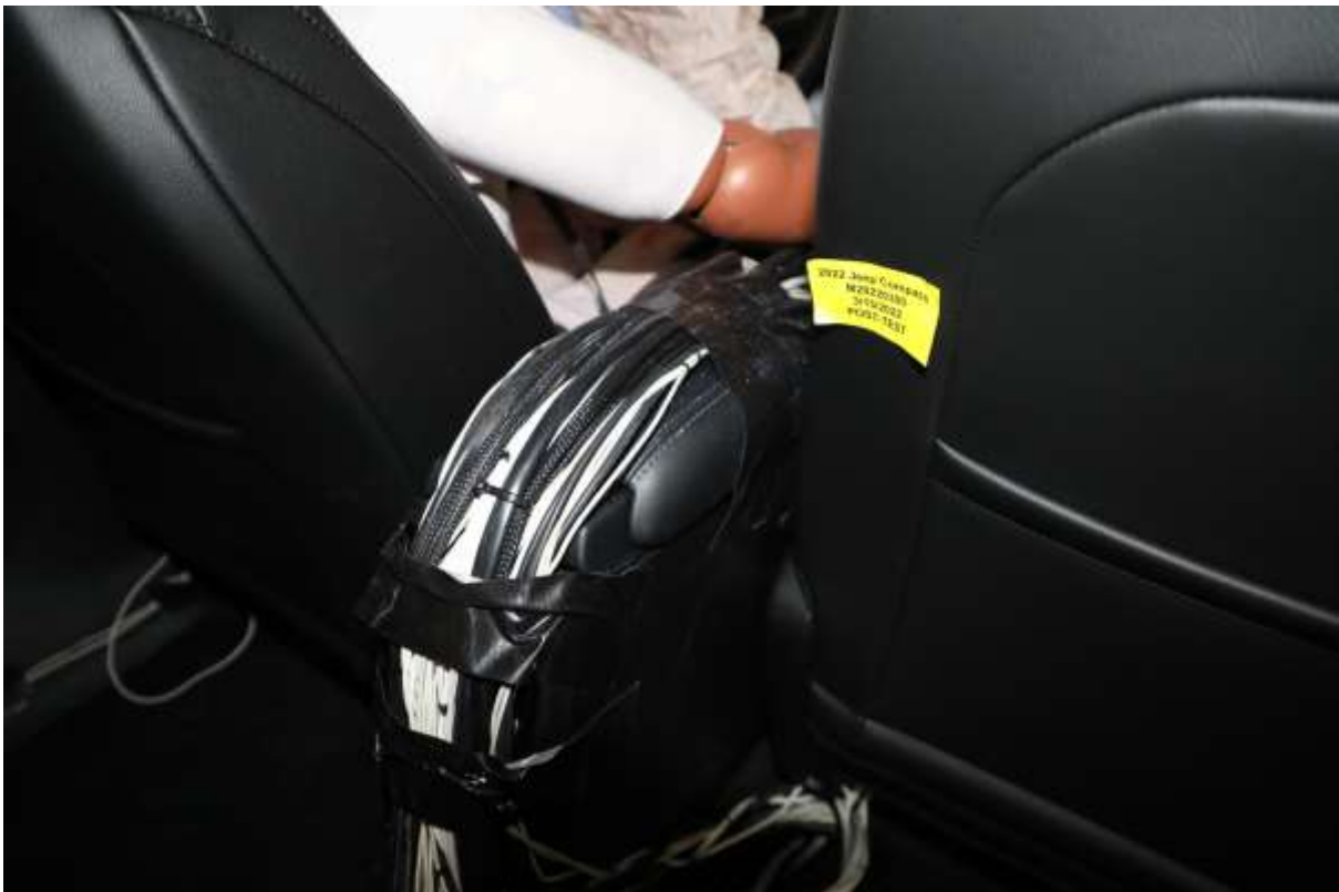
029 Post-Test Dummy Cable Routing
