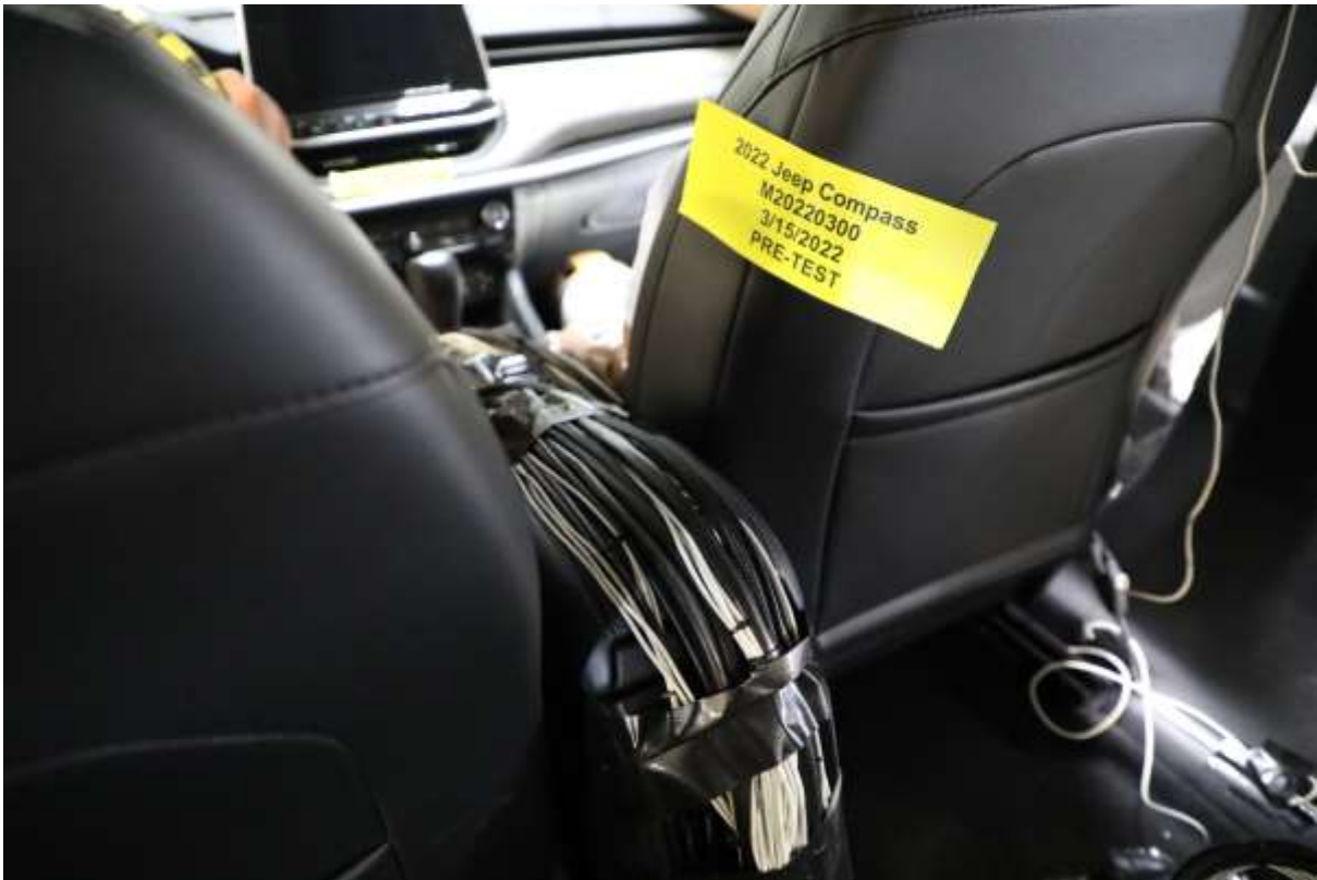
028 Pre-Test Dummy Cable Routing
