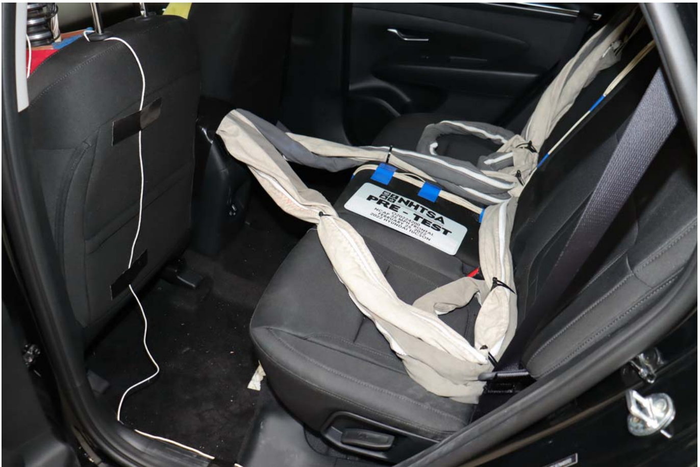
Photo No. 028 - Pre-Test Dummy Cable Routing
