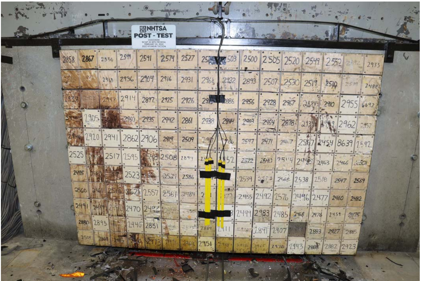
Photo No. 003 - Post-Test Load Cell Wall
