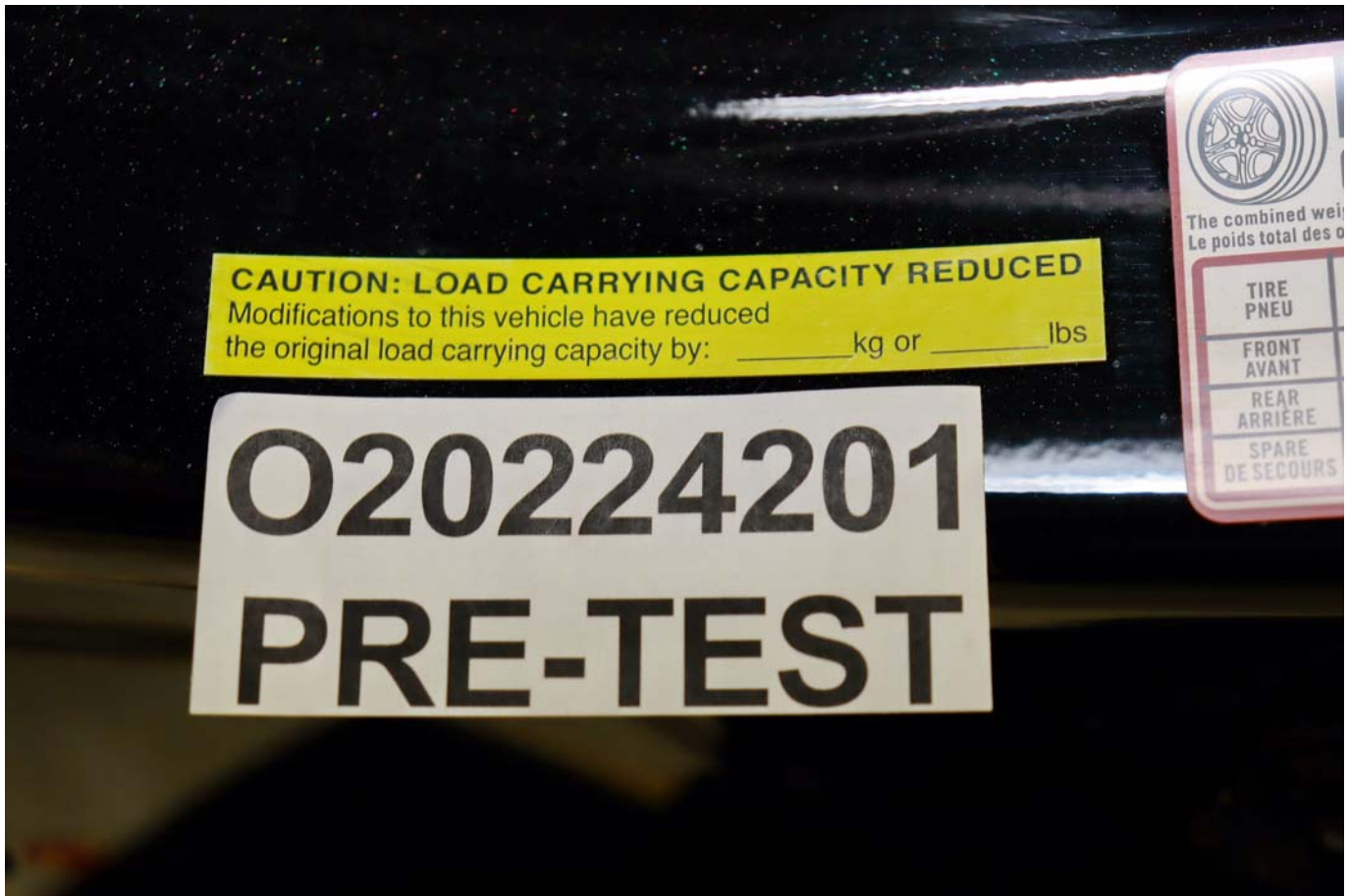
Photo No. 058a - Close-Up View of Vehicle Load Carrying Capacity Reduction Label
