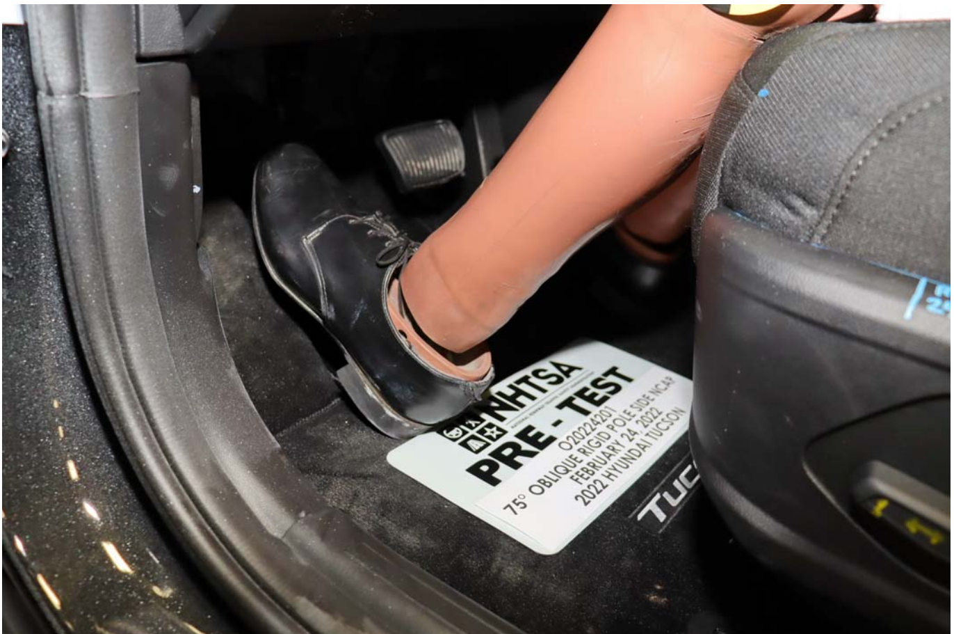
Photo No. 032 - Pre-Test Placement of Dummy's Feet
