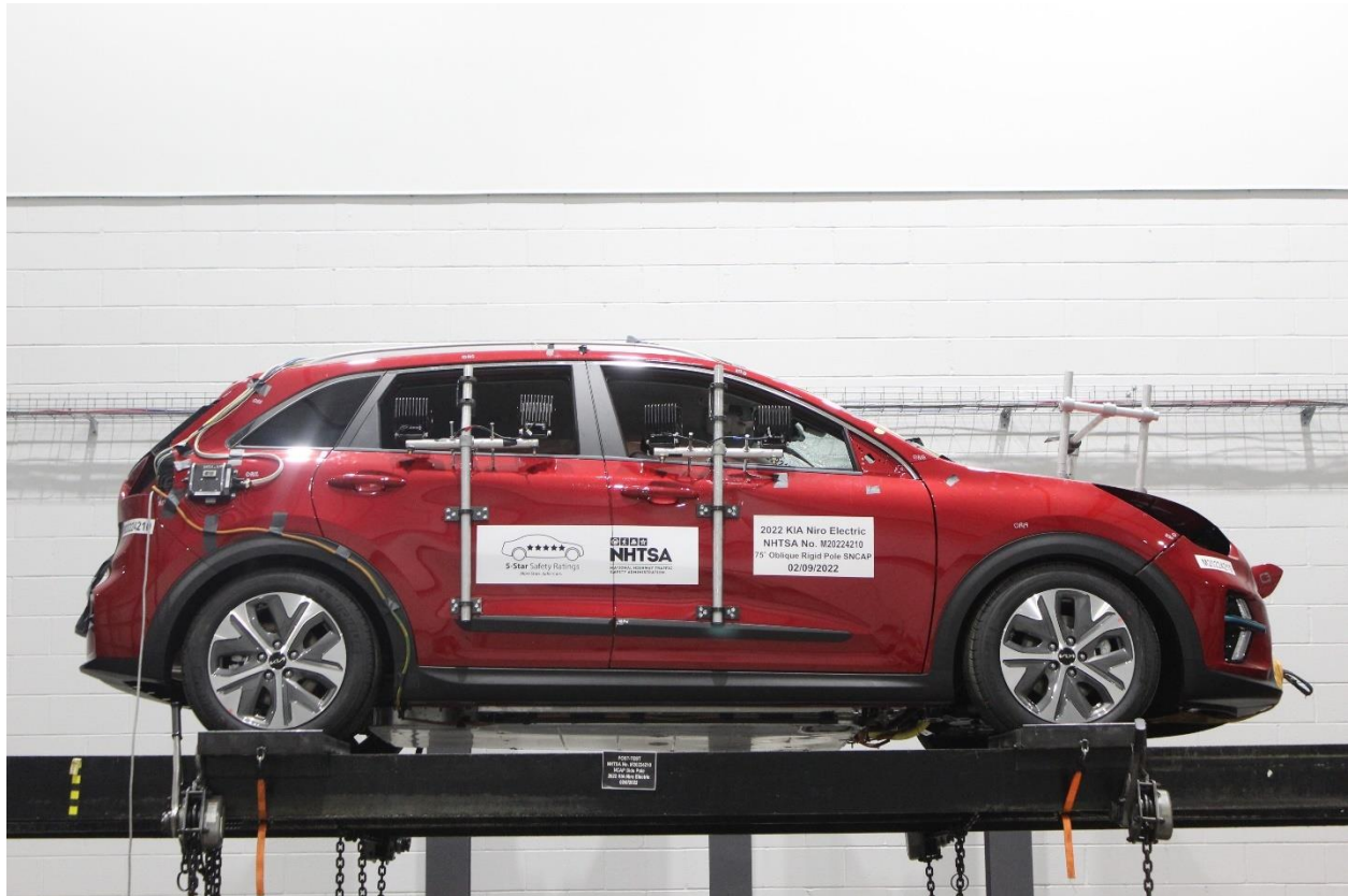
Figure 305-31: FMVSS No. 305 Static Rollover 360 Degrees
