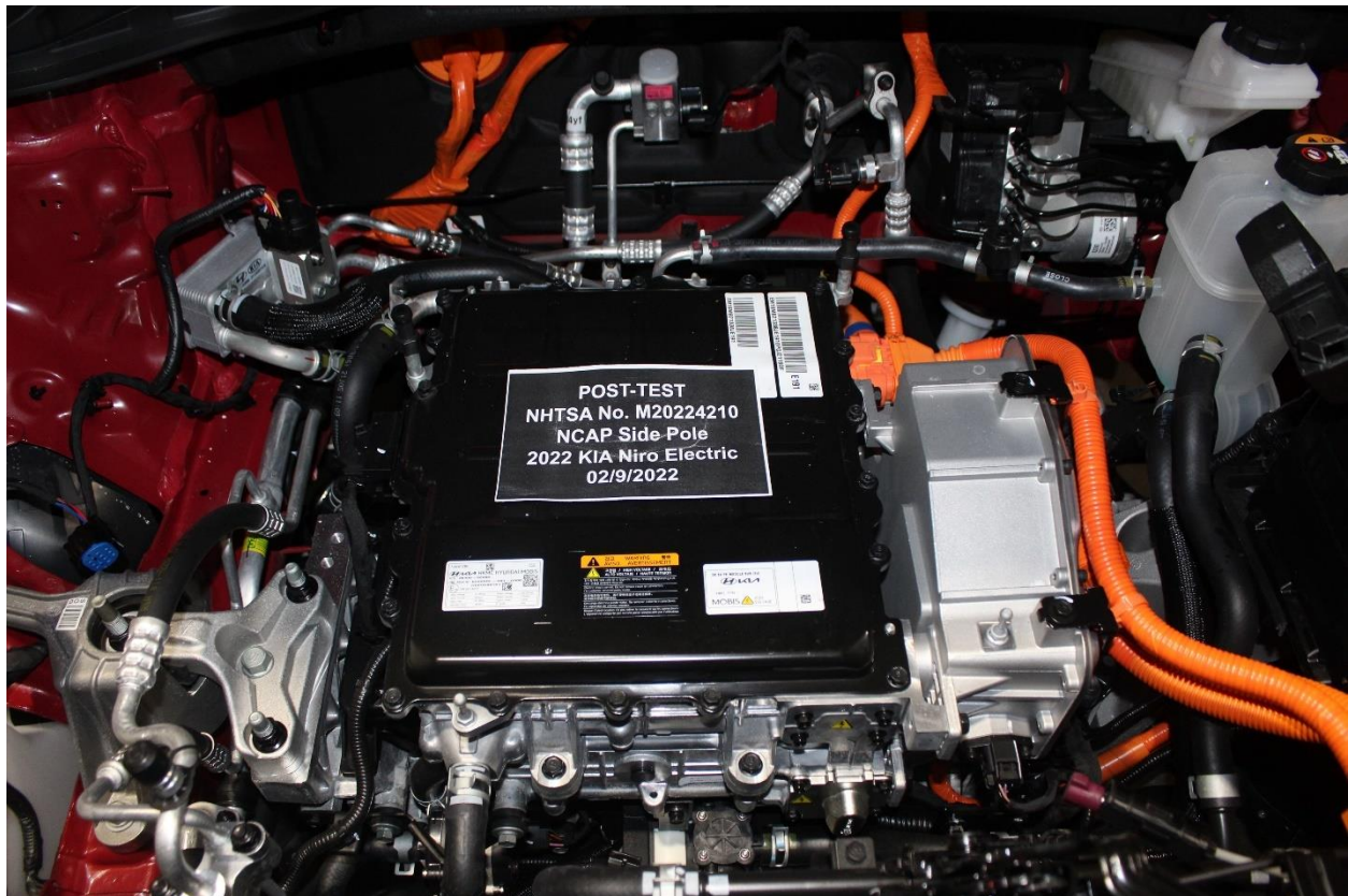
Figure 305-17: Post-Impact View of Electric Propulsion Drive
