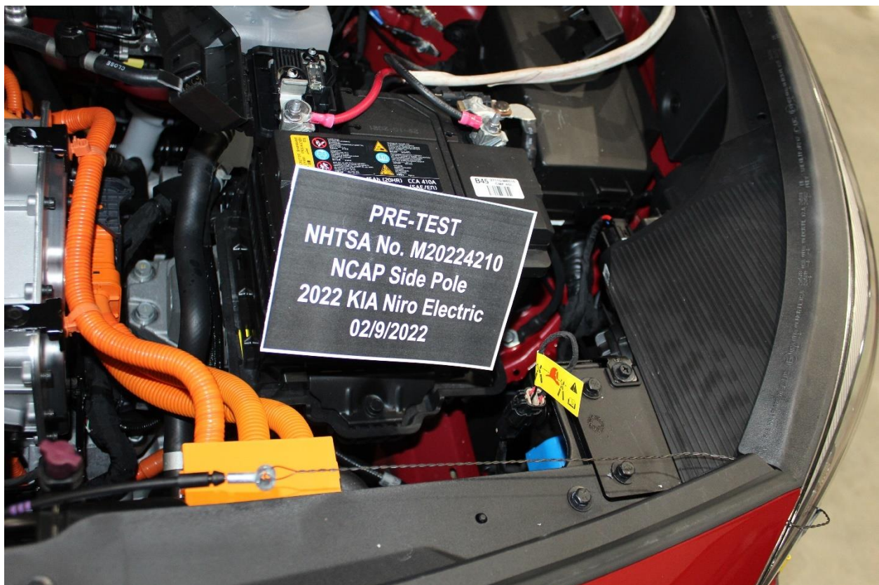
Figure 305-4: First Responder Warning Label Location
