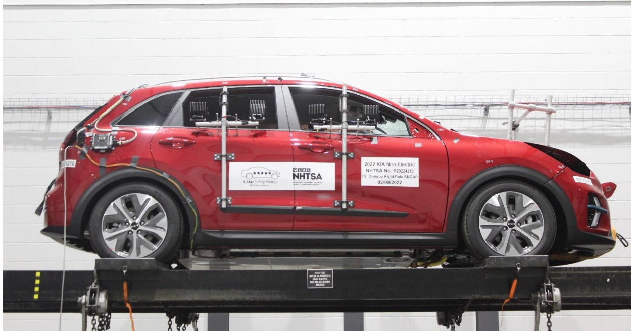
Figure A-65: FMVSS No. 301 Static Rollover 0 Degrees
