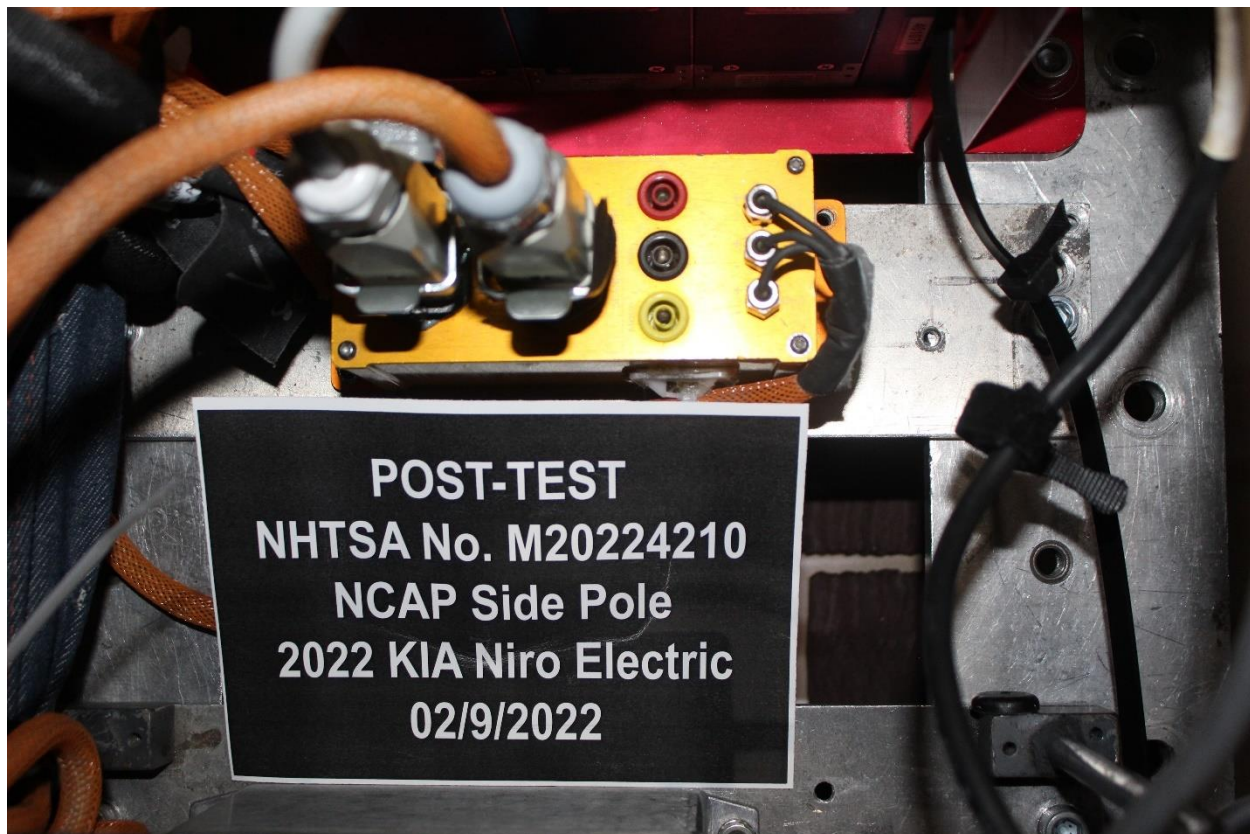
Figure 305-25: Post-Impact View of Installed Test Interface Port
