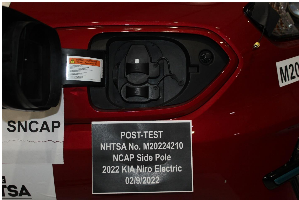
Figure A-56: Post-Test View of Charging Port
