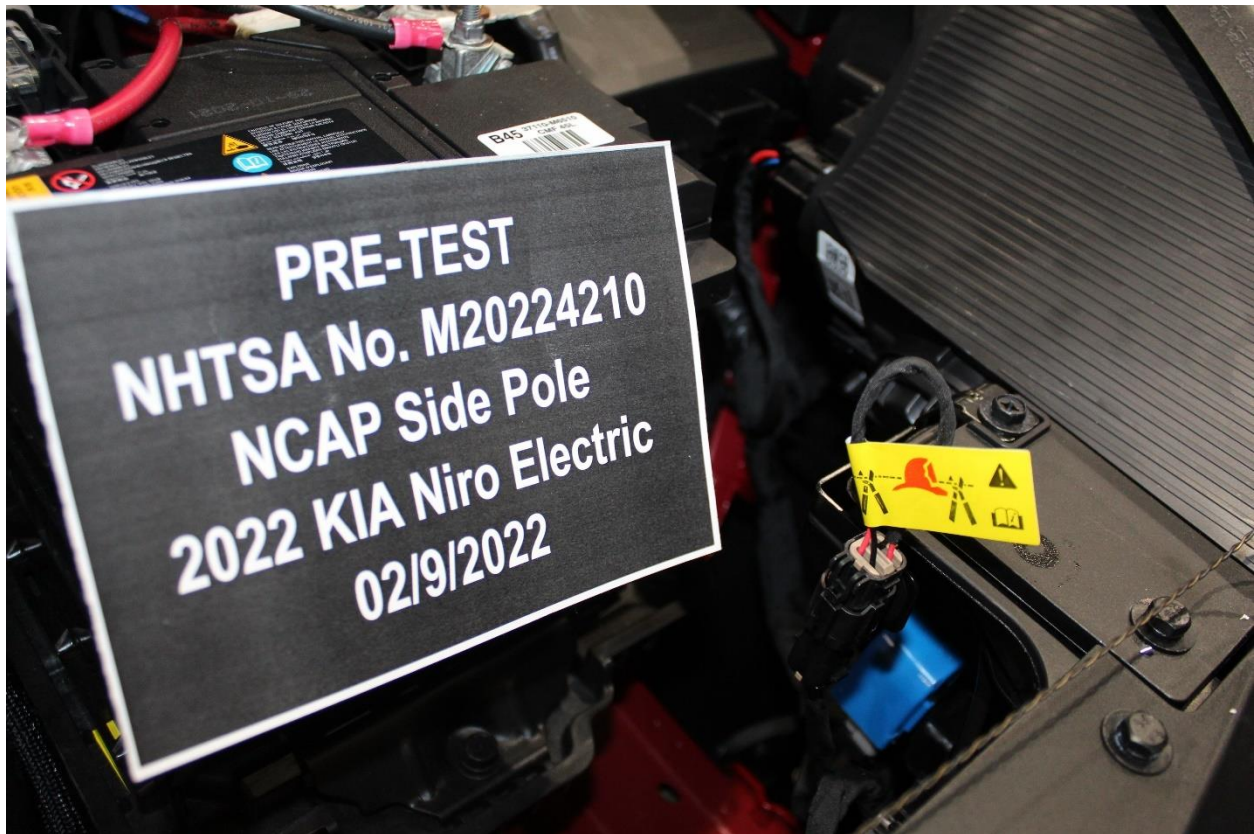
Figure 305-3 First Responder Warning Label
