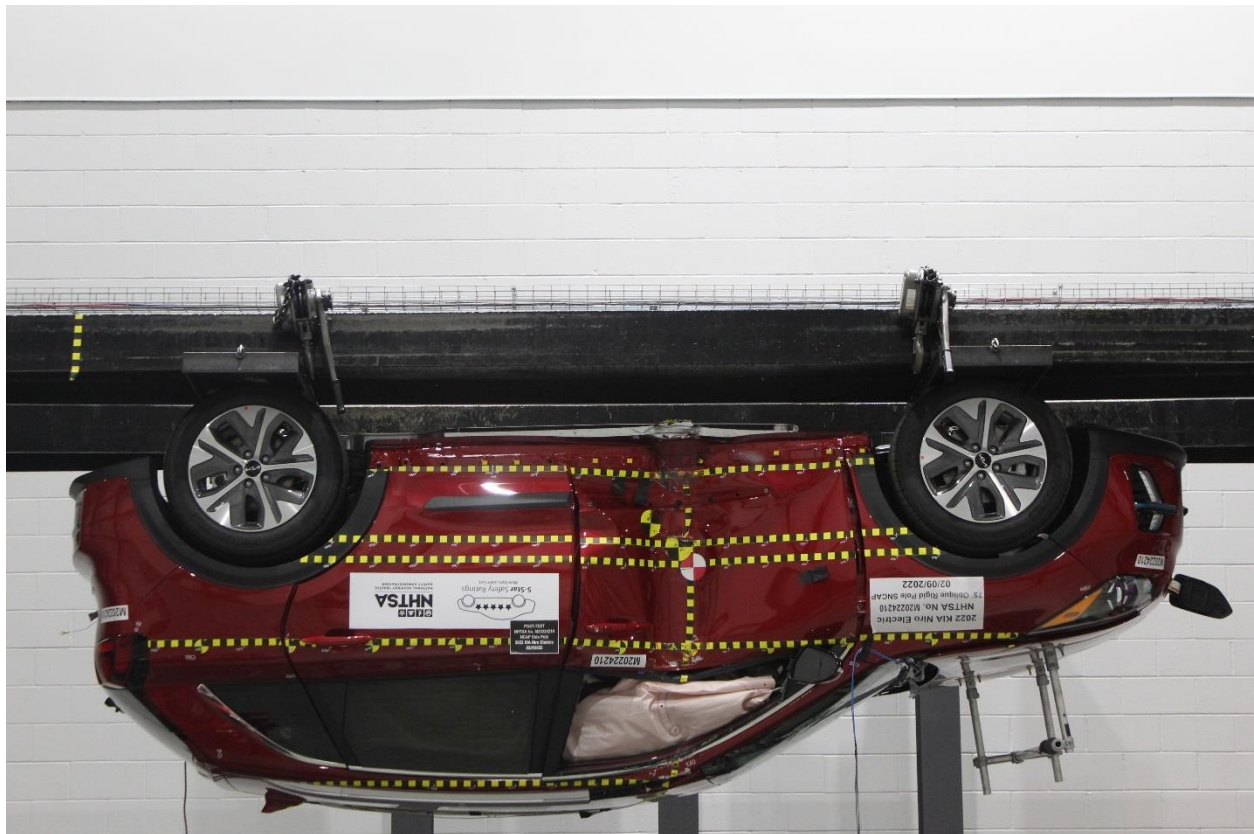
Figure 305-29: FMVSS No. 305 Static Rollover 180 Degrees
