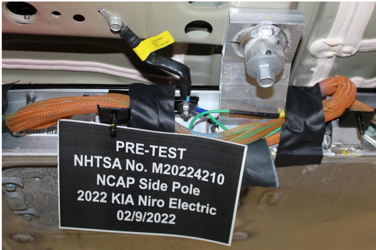
Figure 305-21: Pre-Impact View of Ground Lead Attached
