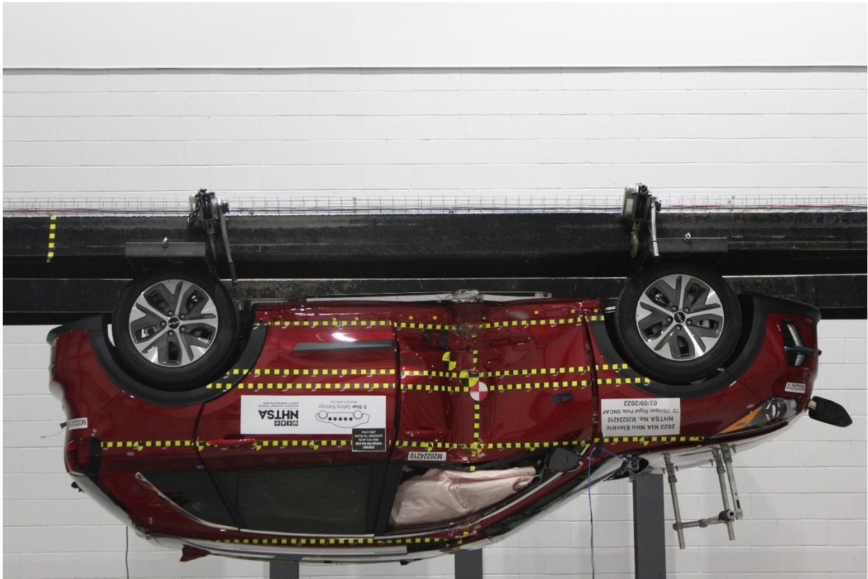
Figure A-67: FMVSS No. 301 Static Rollover 180 Degrees
