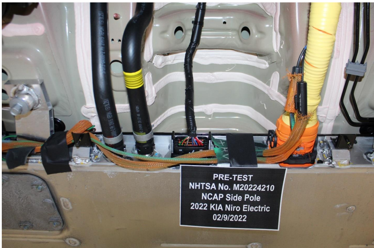
Figure 305-22: Pre-Impact View of High Voltage Leads Attached
