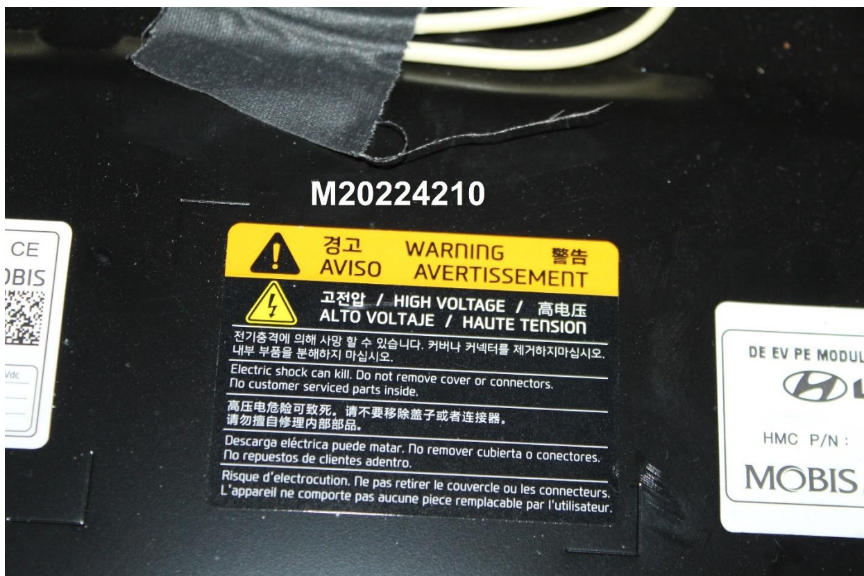
Figure 305-2: Power Inverter Warning Label
