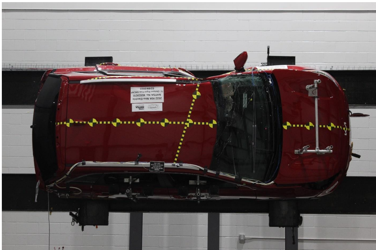
Figure 305-30: FMVSS No. 305 Static Rollover 270 Degrees
