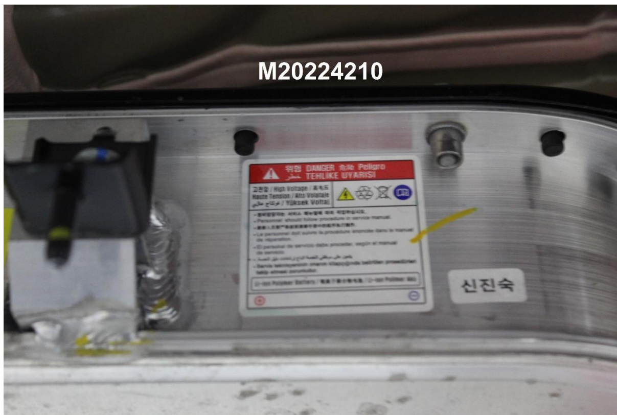
Figure 305-1: Auxiliary Power Module Warning Label
