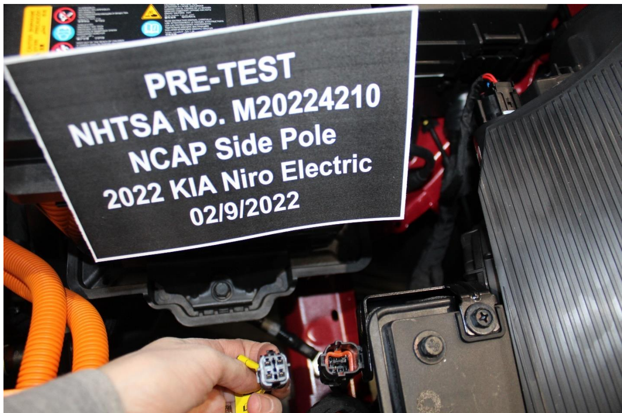
Figure 305-8: Manual High Voltage Service Disconnect Removed Location
