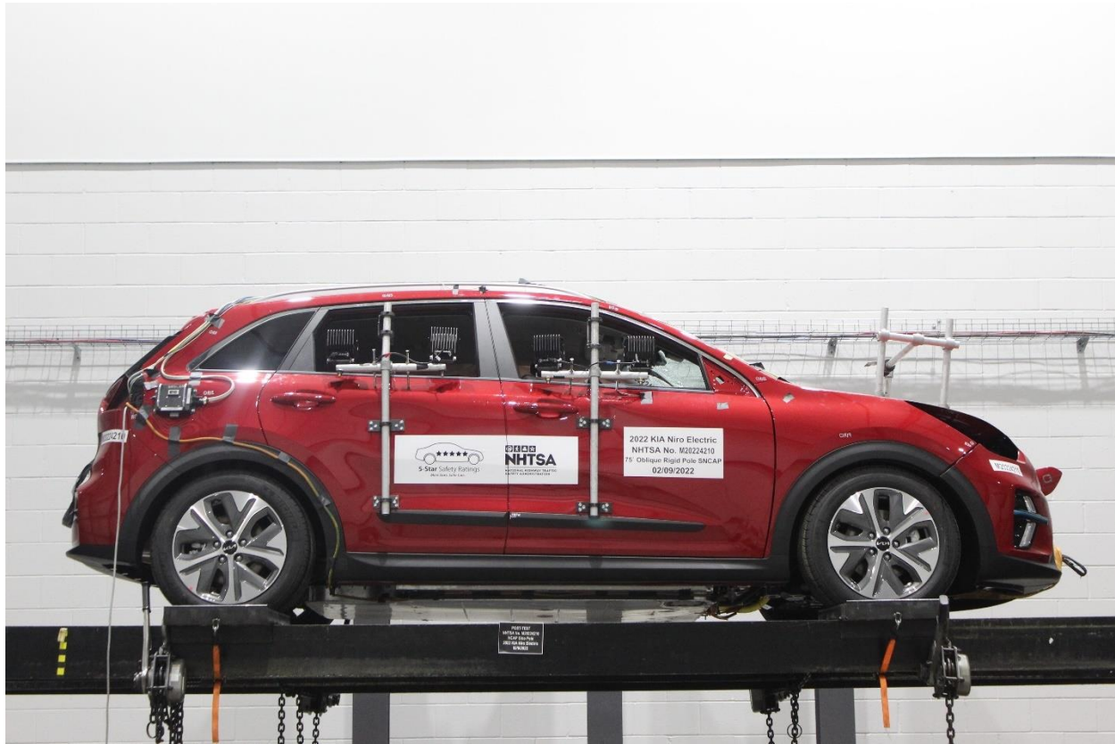
Figure A-69: FMVSS No. 301 Static Rollover 360 Degrees
