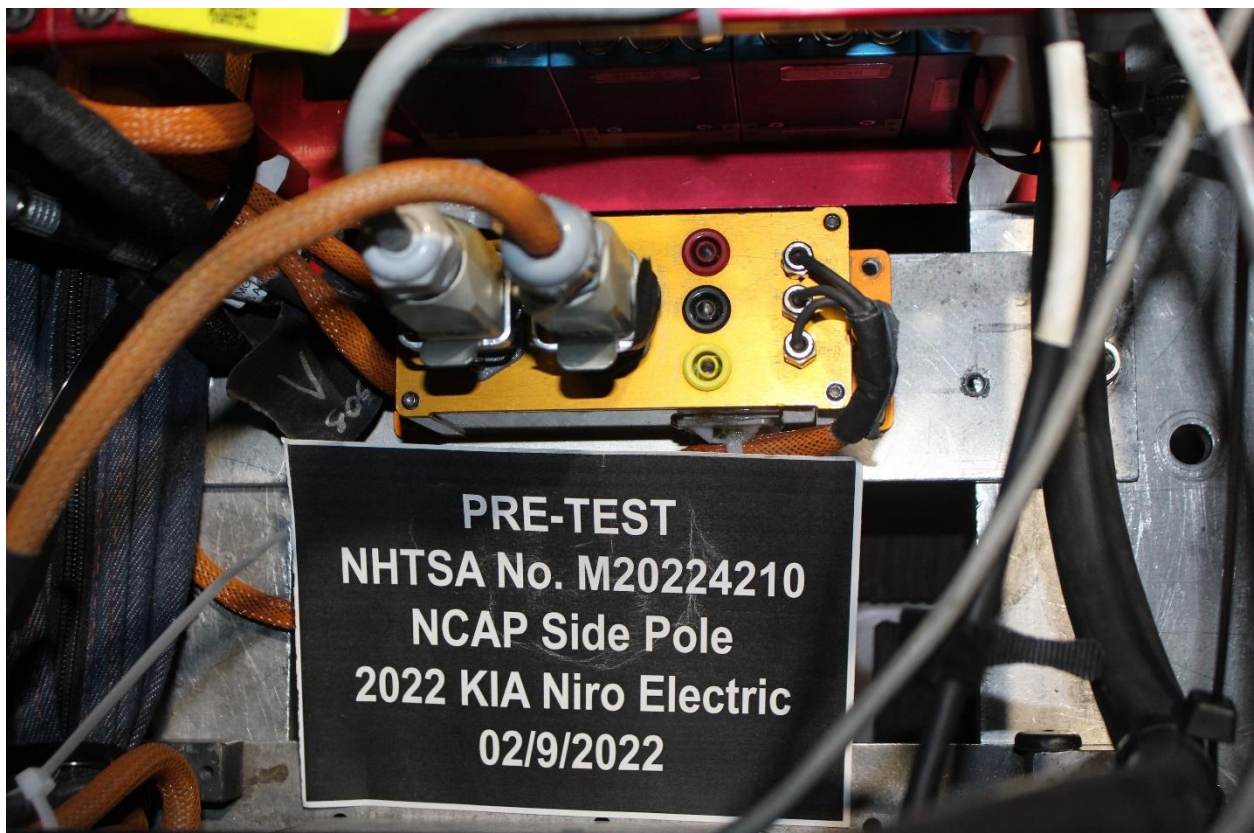
Figure 305-24: Pre-Impact View of Installed Test Interface Port
