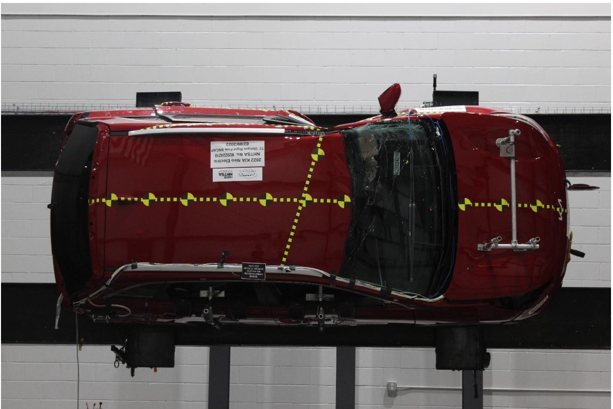
Figure A-68: FMVSS No. 301 Static Rollover 270 Degrees
