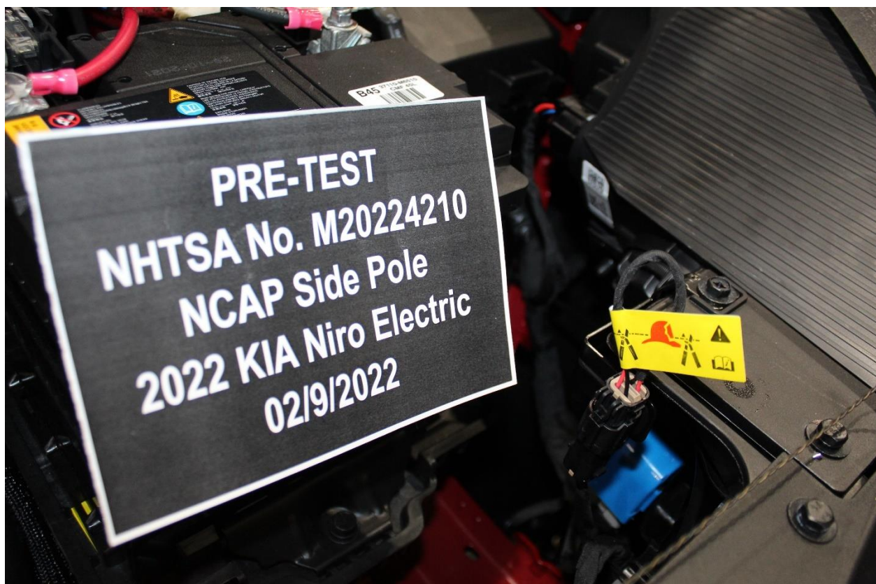
Figure 305-6: Manual High Voltage Service Disconnect in Place
