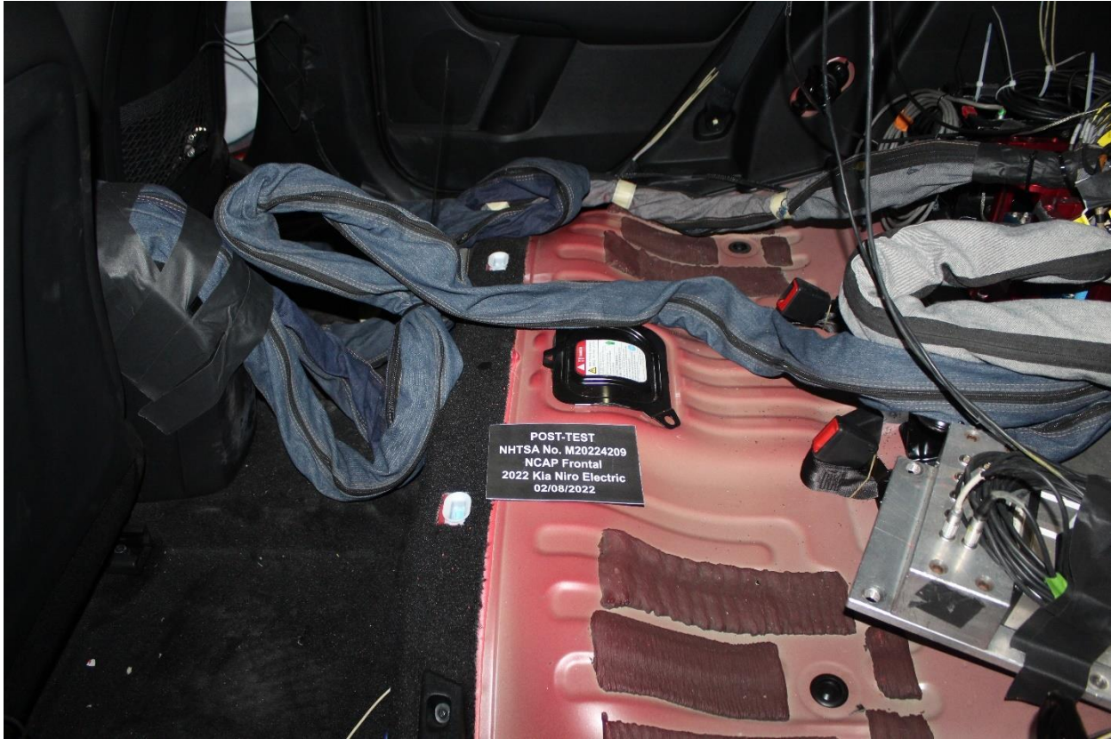
Figure A-29: Post-Test Dummy Cable Routing
