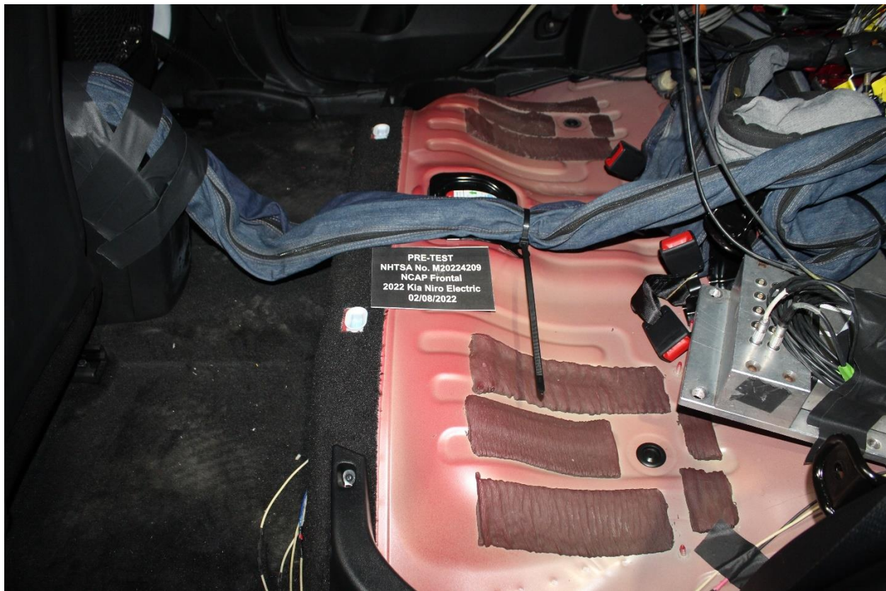
Figure A-28: Pre-Test Dummy Cable Routing
