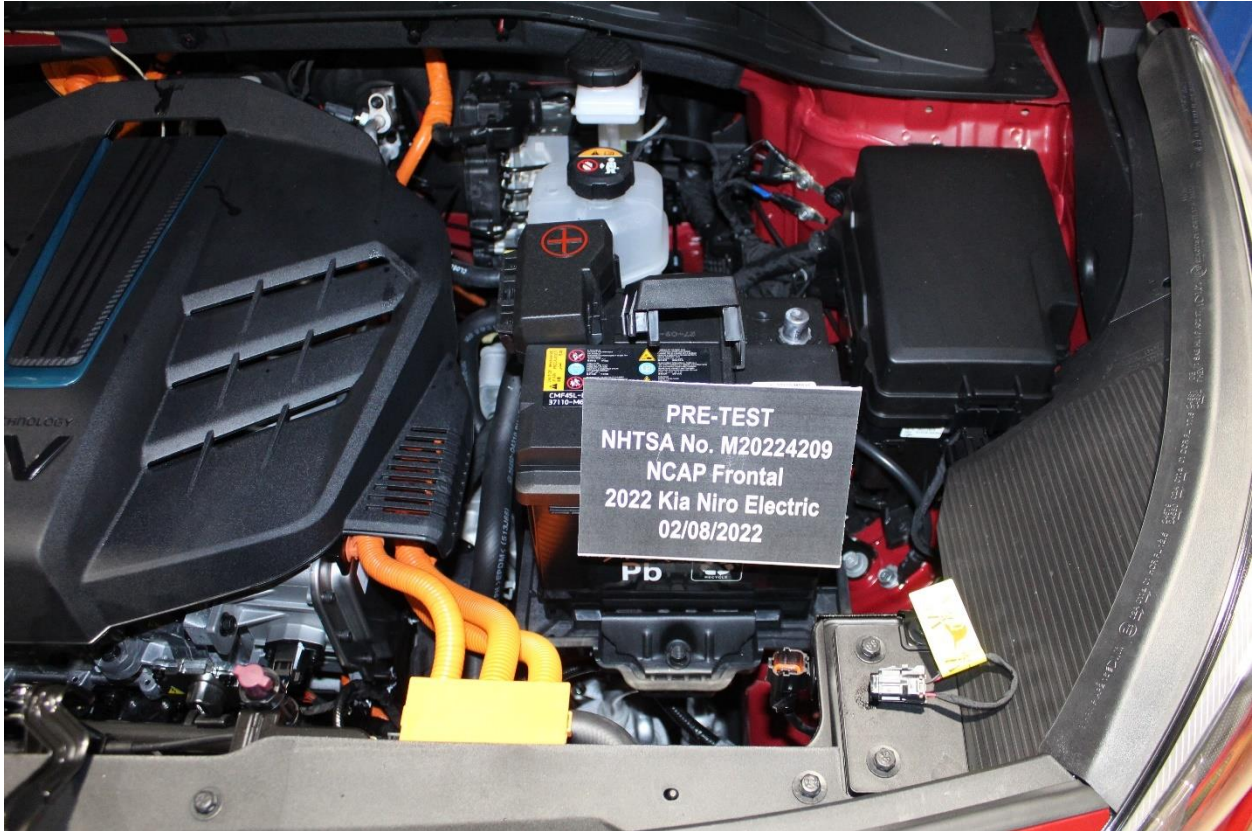
Figure 305-8: Manual High Voltage Service Disconnect Removed Location
