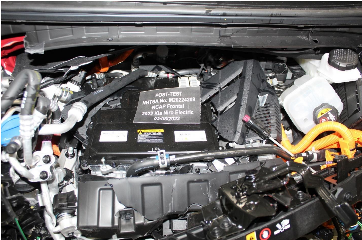
Figure 305-17: Post-Impact View of Electric Propulsion Drive
