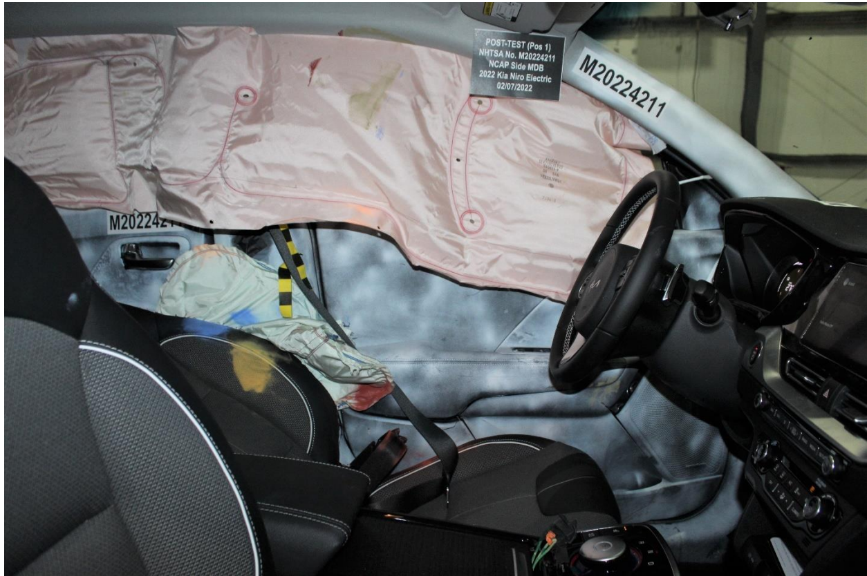
Figure A-47: Post-Test Driver Inner Door Panel View Showing Driver Dummy Contact Locations
