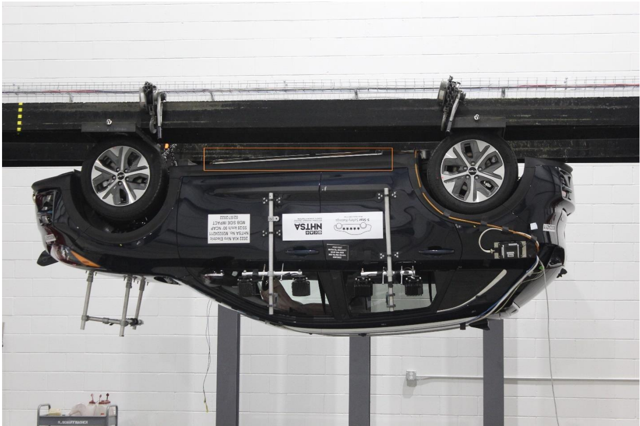
Figure 305-29: FMVSS No. 305 Static Rollover 180 Degrees
