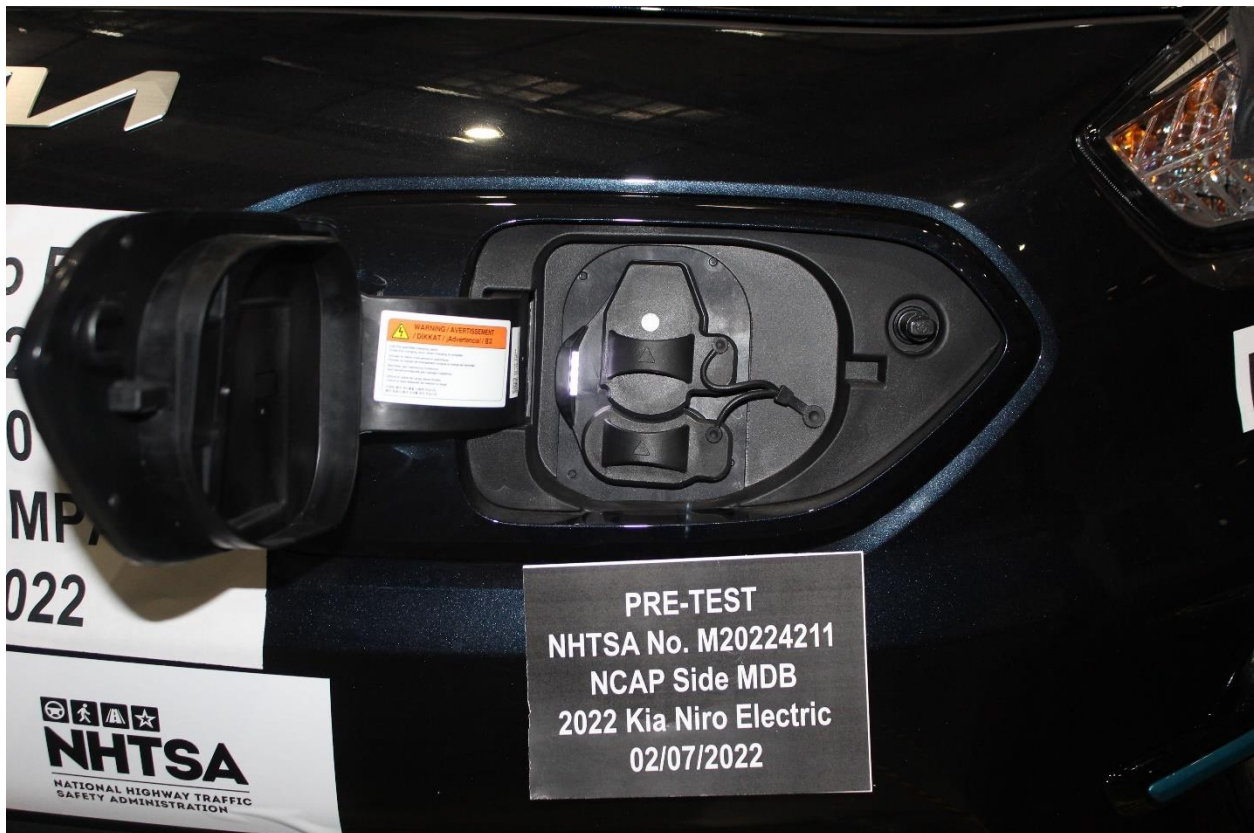
Figure A-82: Pre-Test View of Charging Port
