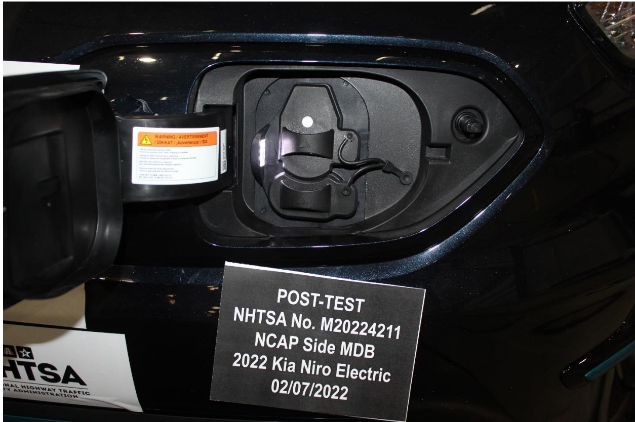
Figure A-83: Post-Test View of Charging Port
