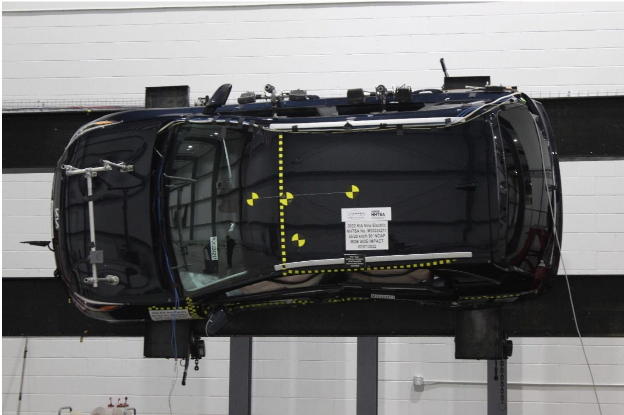
Figure A-99: FMVSS No. 301 Static Rollover 270 Degrees
