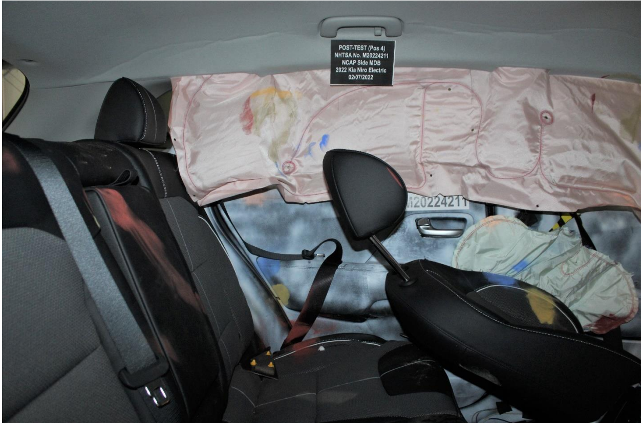
Figure A-74: Post-Test Rear Passenger Inner Door Panel View Showing Rear Passenger Dummy Contact Locations
