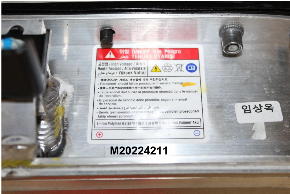
Figure 305-1: Auxiliary Power Module Warning Label
