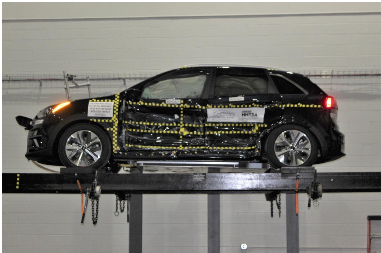
Figure A-96: FMVSS No. 301 Static Rollover 0 Degrees
