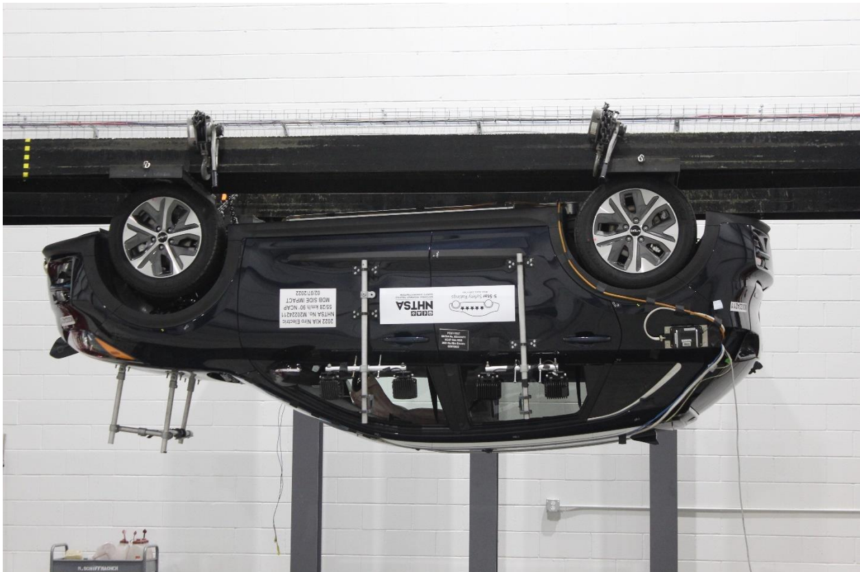
Figure A-98: FMVSS No. 301 Static Rollover 180 Degrees
