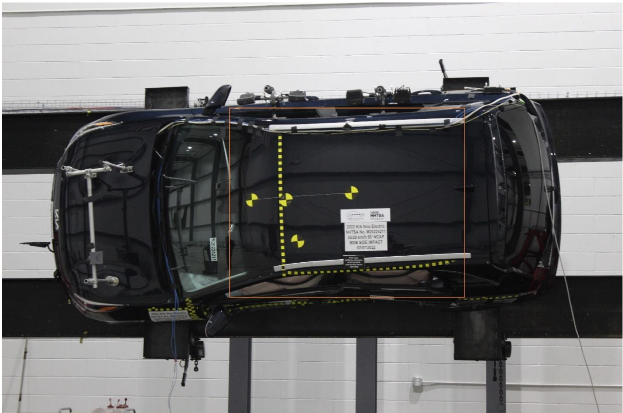
Figure 305-30: FMVSS No. 305 Static Rollover 270 Degrees
