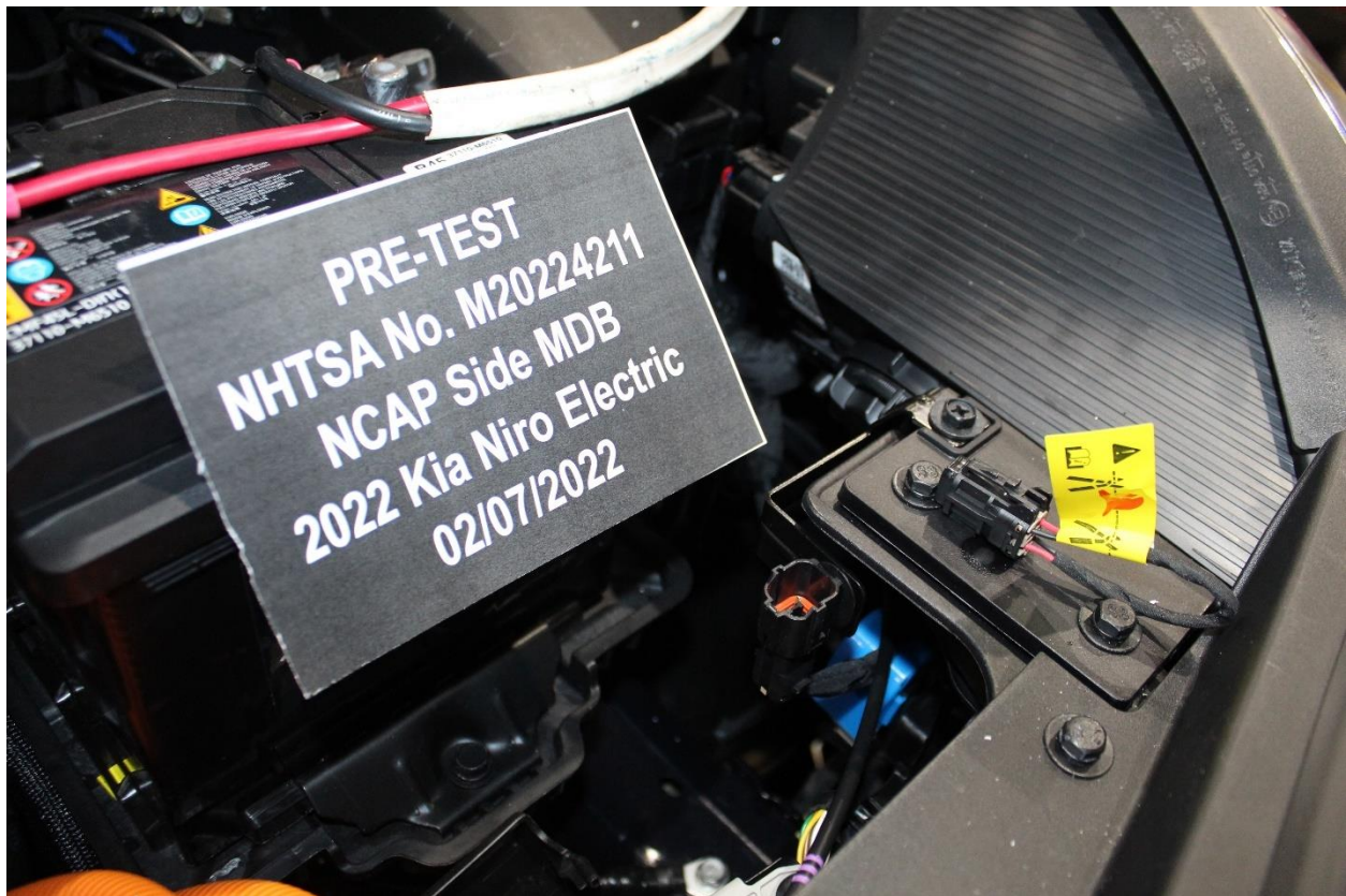
Figure 305-8: Manual High Voltage Service Disconnect Removed Location
