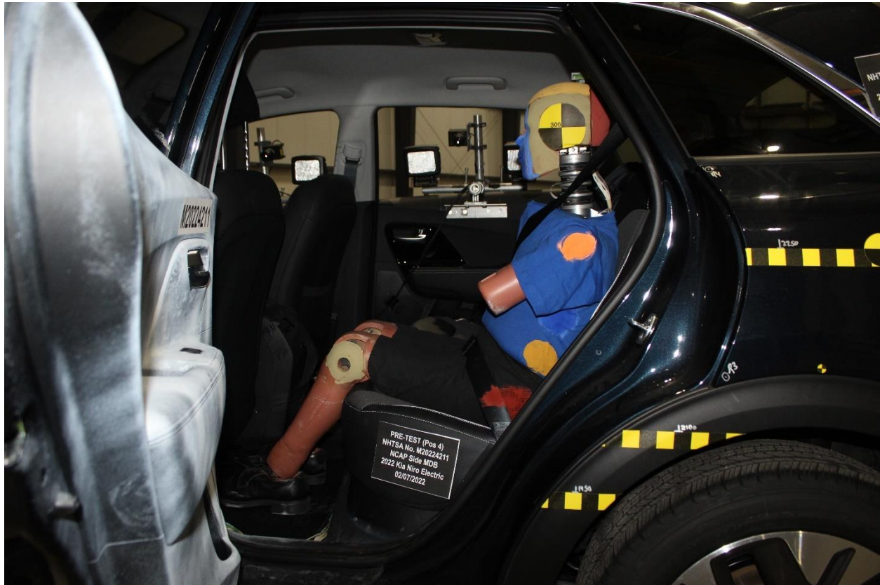
Figure A-55: Pre-Test Left Side View of Rear Passenger Dummy Showing Belt and Chalking
