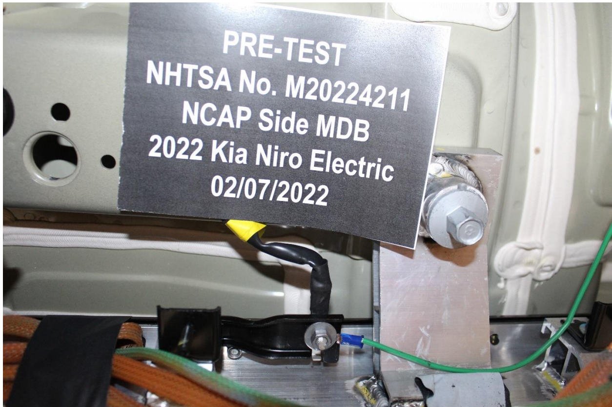
Figure 305-21: Pre-Impact View of Ground Lead Attached
