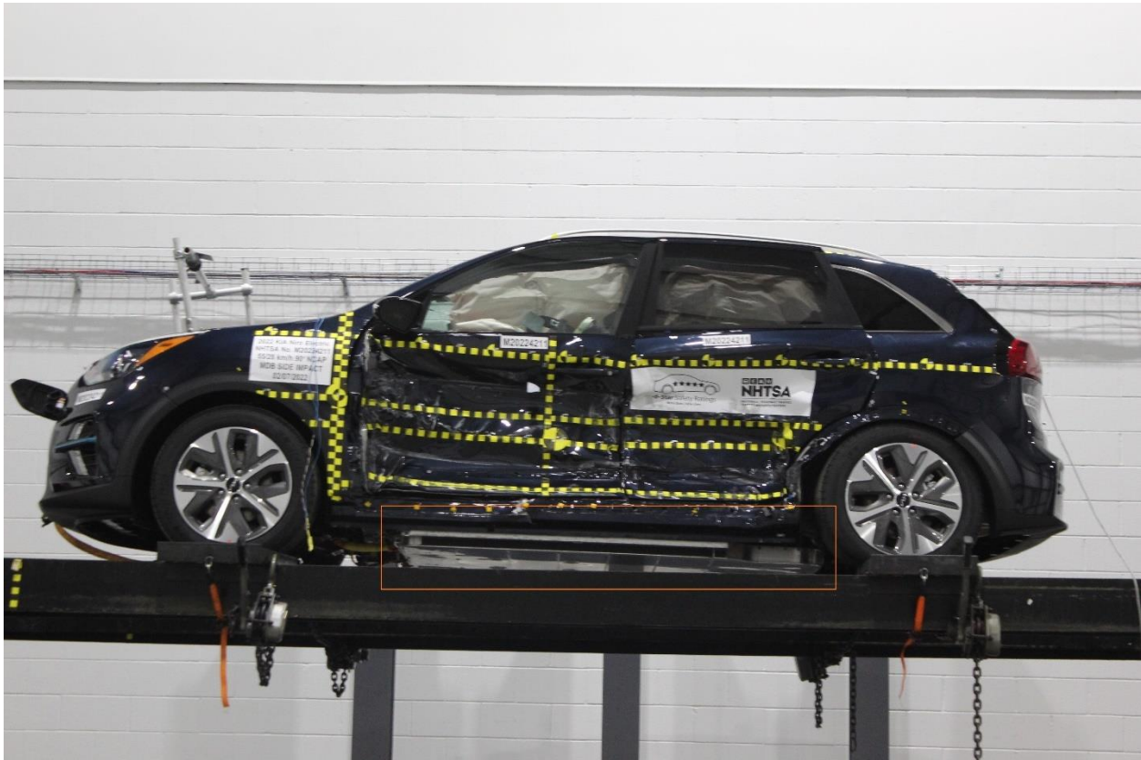
Figure 305-31: FMVSS No. 305 Static Rollover 360 Degrees
