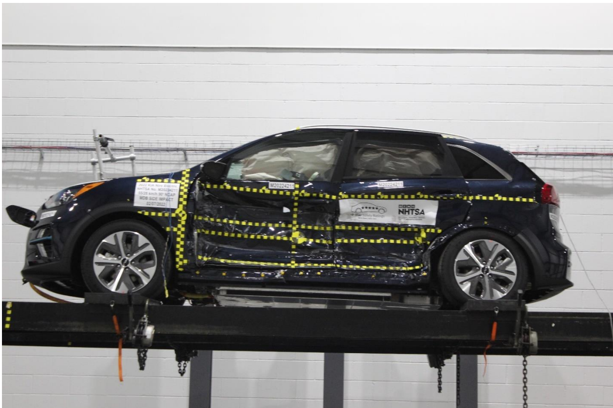
Figure A-100: FMVSS No. 301 Static Rollover 360 Degrees
