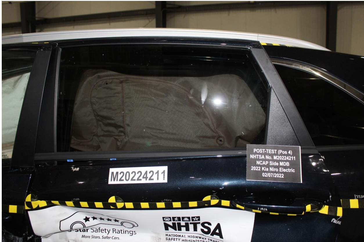
Figure A-57: Post-Test Left Side View of Rear Passenger Dummy Shoulder and Door Top View
