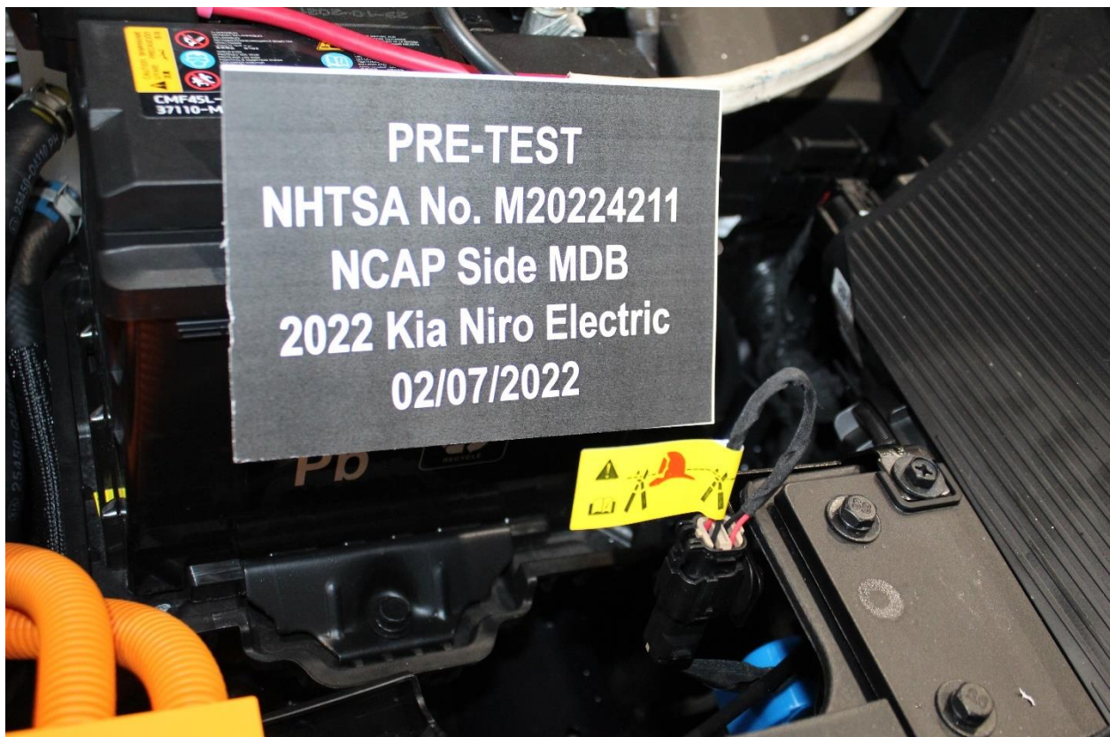
Figure 305-6: Manual High Voltage Service Disconnect in Place
