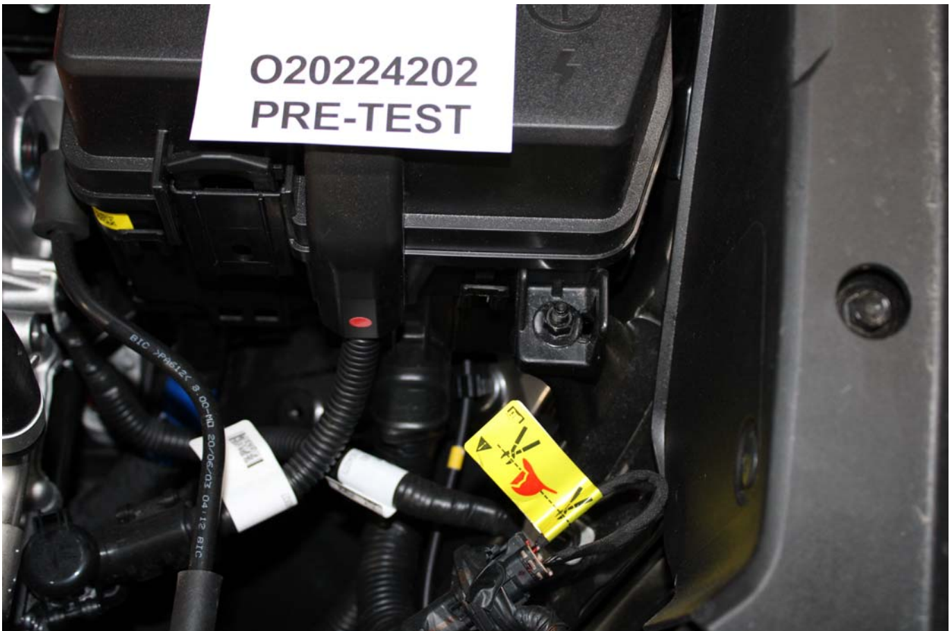
Photo No. 305-03 - First Responder Warning Label
