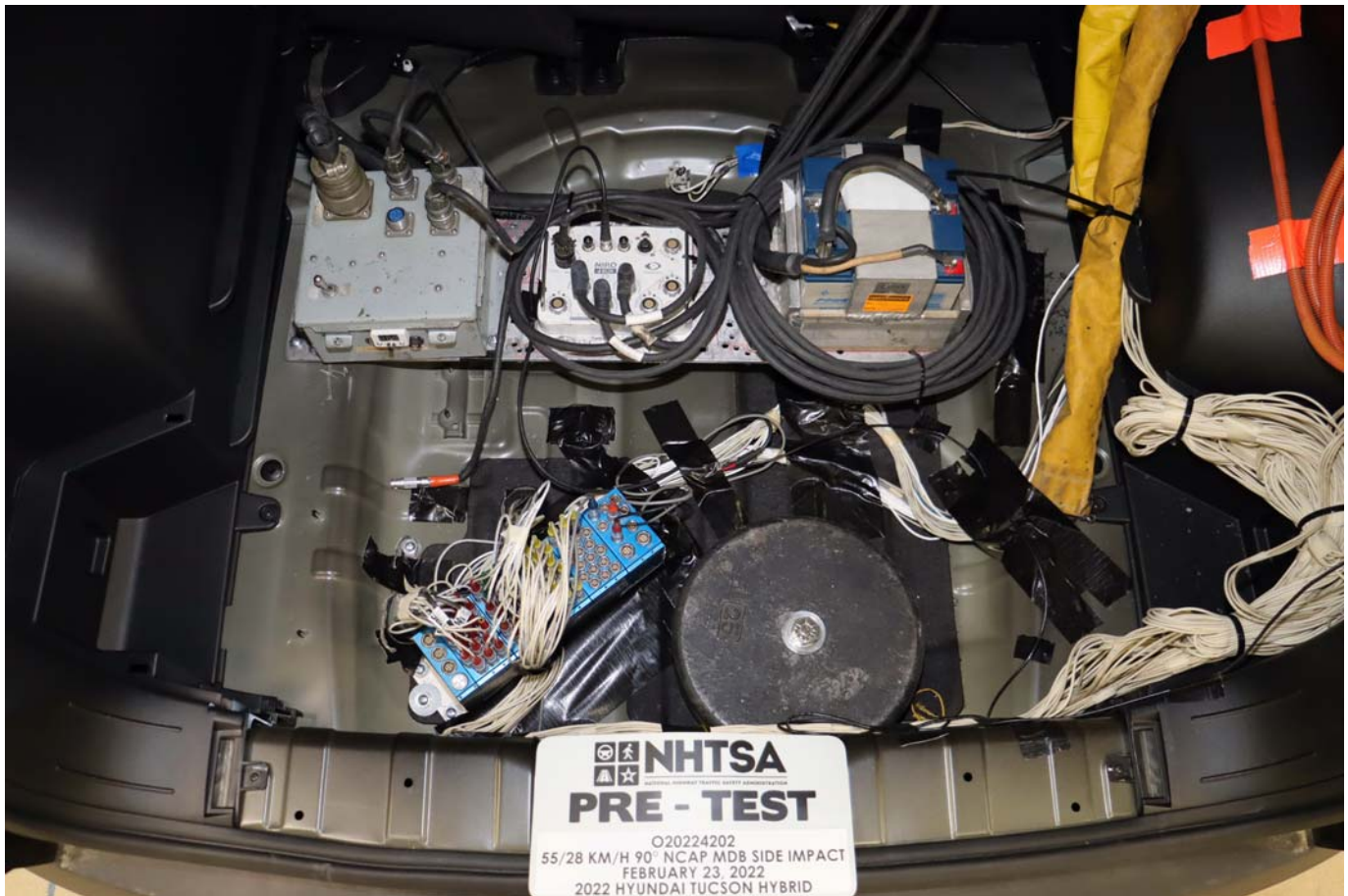
Photo No. 094 - Pre-Test Ballast View
