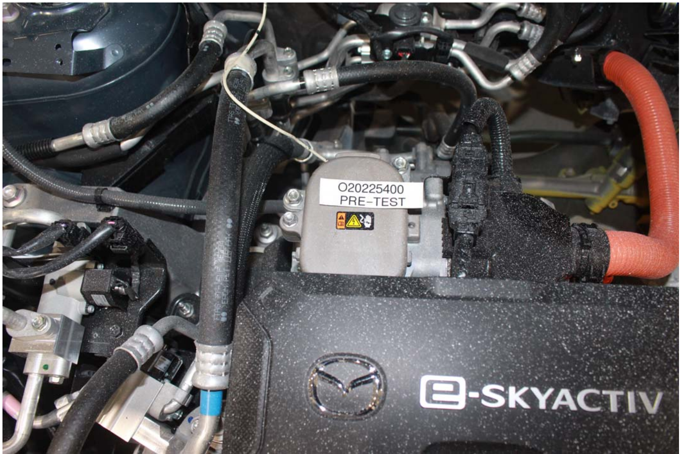
Photo No. 305-02 - Power Inverter Warning Label
