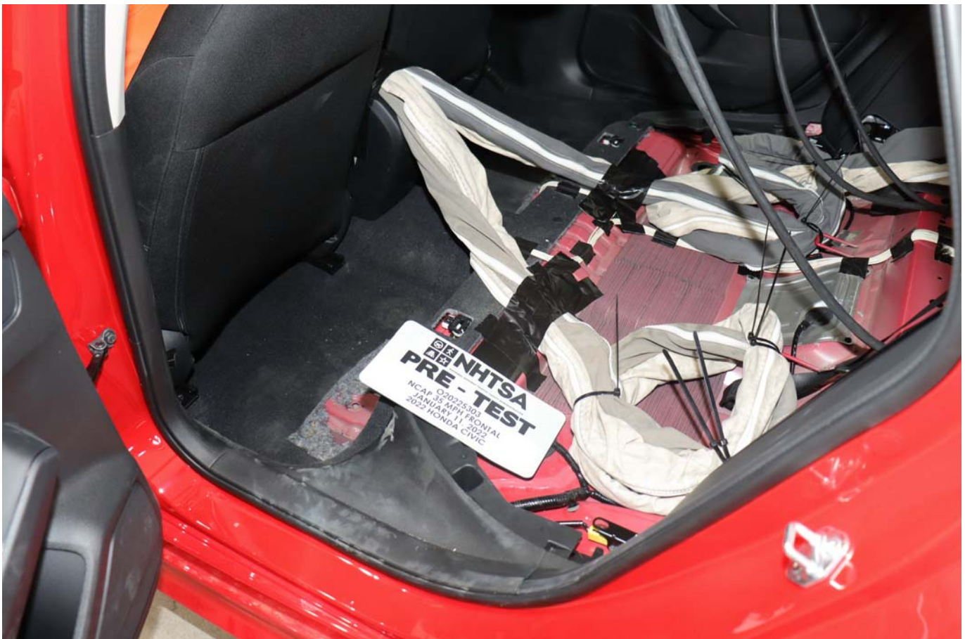
Photo No. 028 - Pre-Test Dummy Cable Routing
