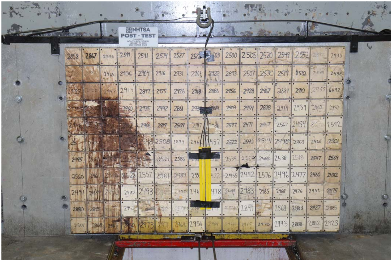
Photo No. 003 - Post-Test Load Cell Wall
