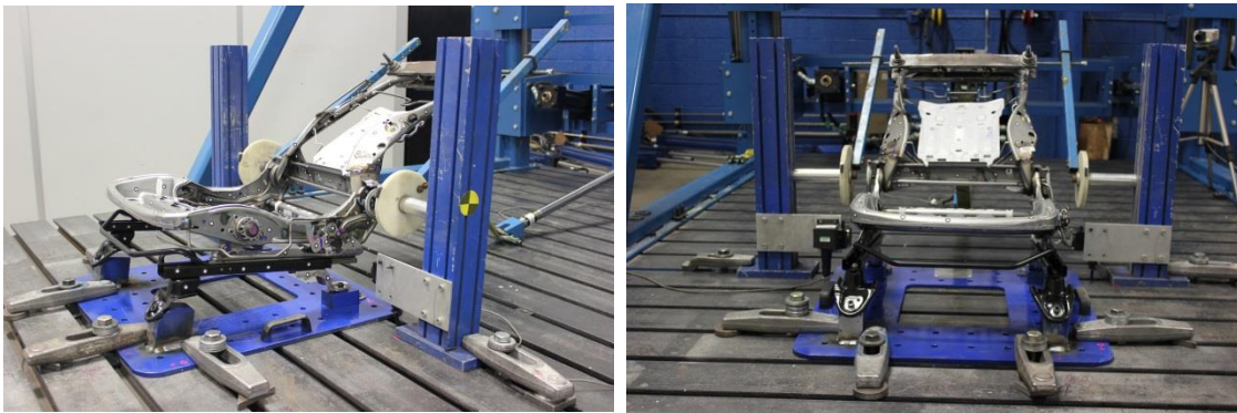
Figure 4: Seat Back Pull Test, Post Test – Manual Seat
