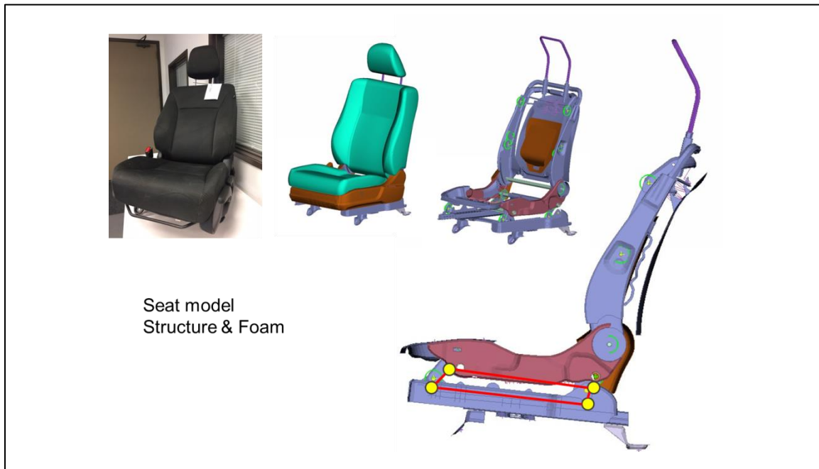
Figure 31: Seat FEM –Mechanism and Cushions (Ex. Manual Seat)
