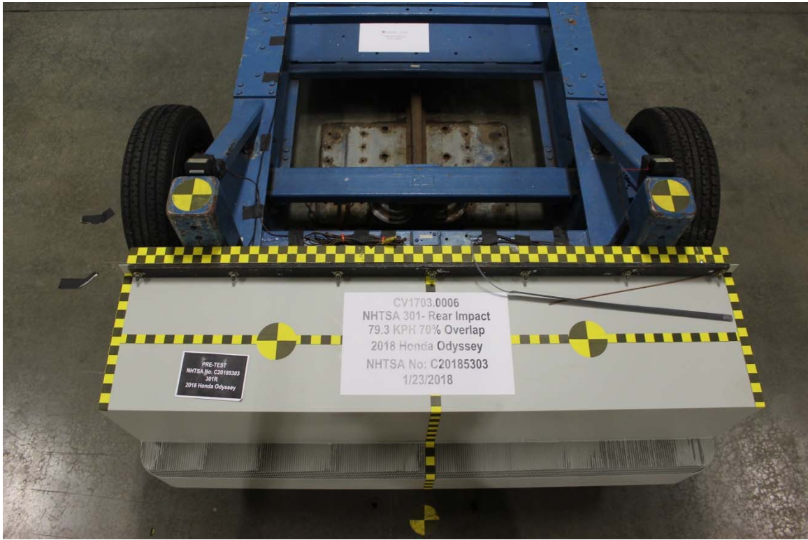
Figure A-25: Pre-Test MDB Top View
