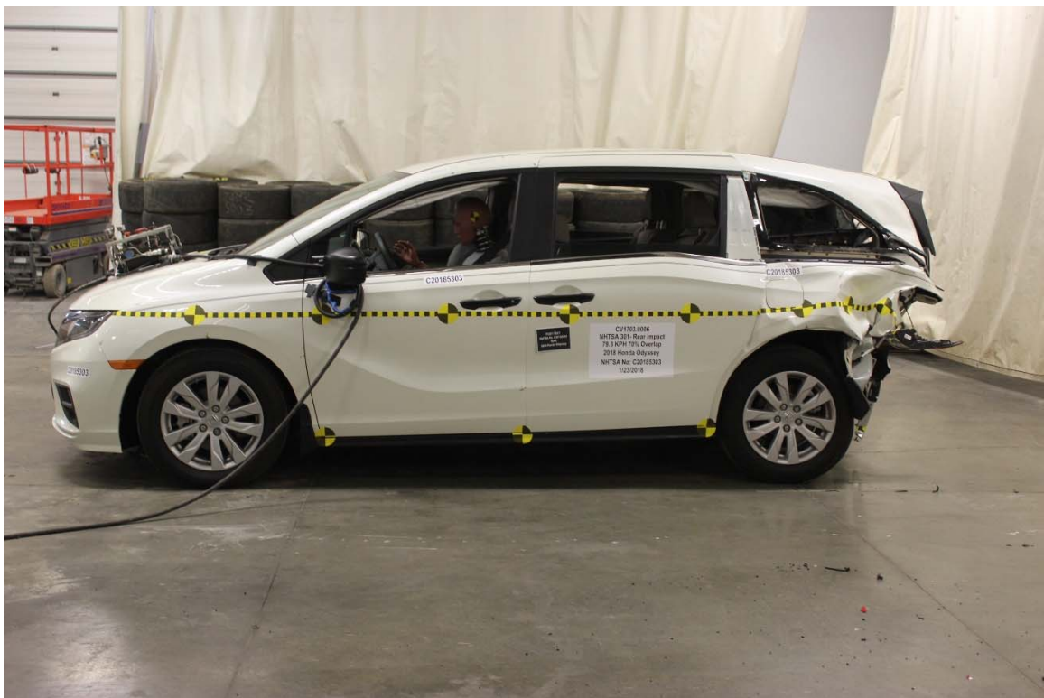
Figure A-6: Post-Test Left Side View
