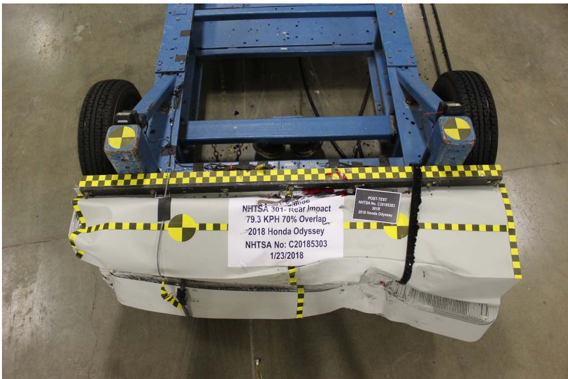
Figure A-26: Post-Test MDB Top View
