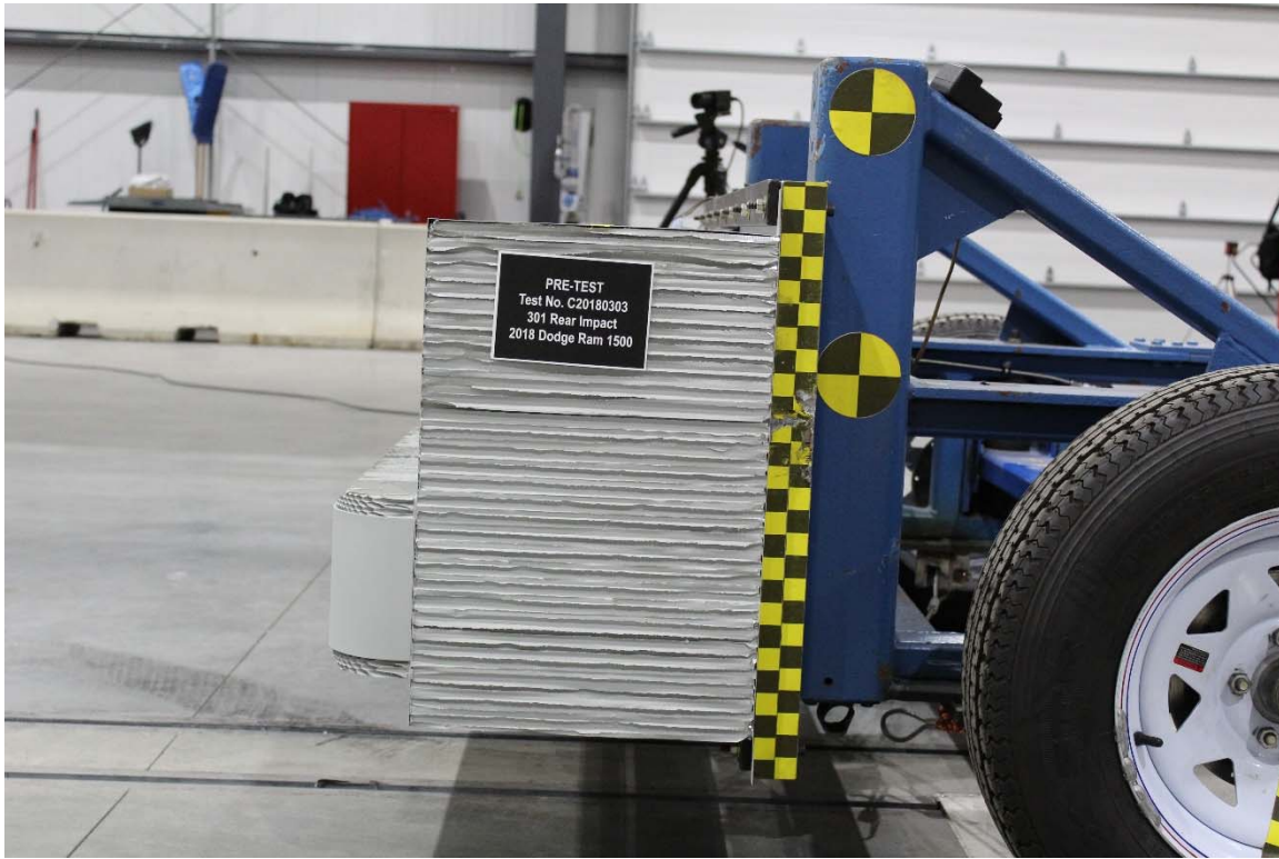
Figure A-21: Pre-Test MDB Left Side View
