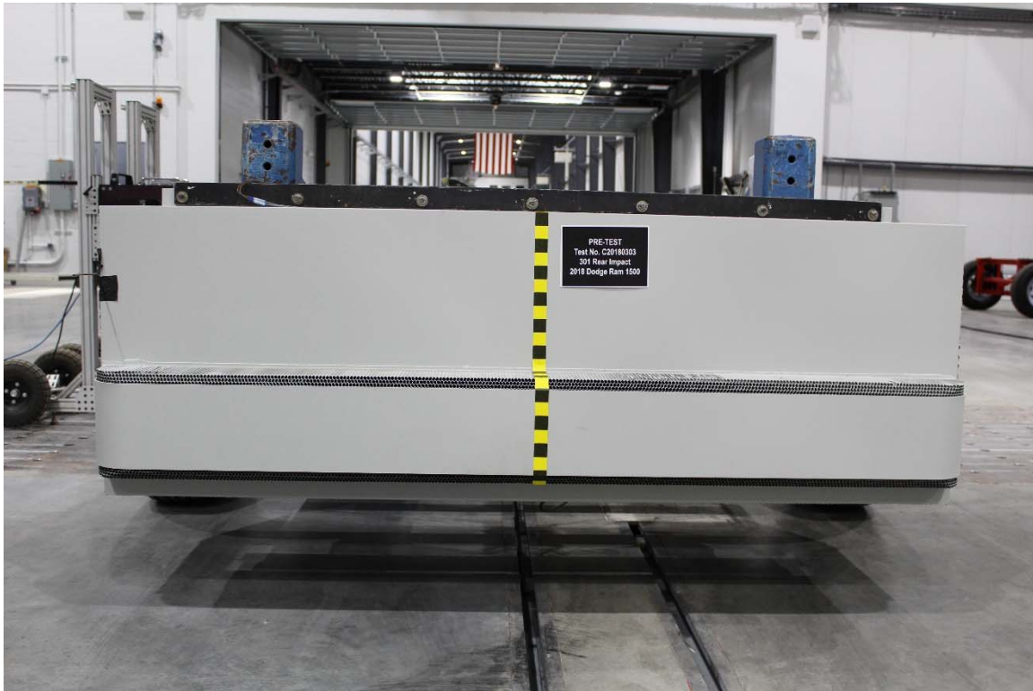
Figure A-19: Pre-Test MDB Front View
