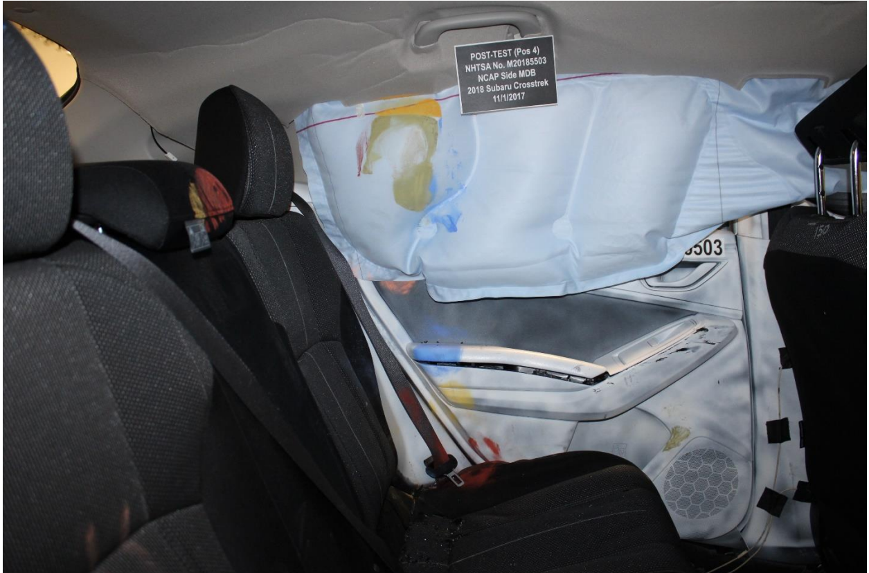
Figure A-74: Post-Test Passenger Inner Door Panel View
