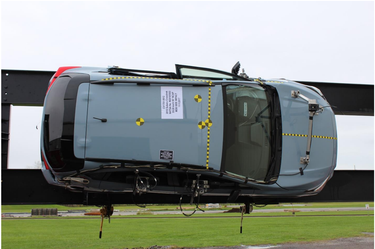
Figure A-97: FMVSS No. 301 Static Rollover 90 Degrees
