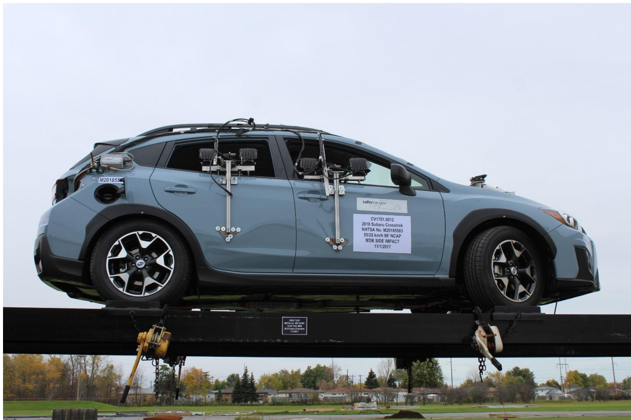
Figure A-96: FMVSS No. 301 Static Rollover 0 Degrees
