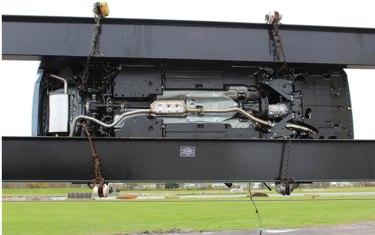
Figure A-99: FMVSS No. 301 Static Rollover 270 Degrees
