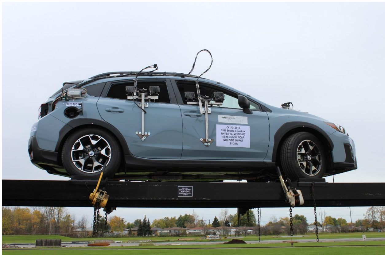
Figure A-100: FMVSS No. 301 Static Rollover 360 Degrees
