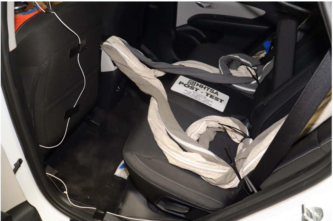
Photo No. 029 - Post-Test Dummy Cable Routing
