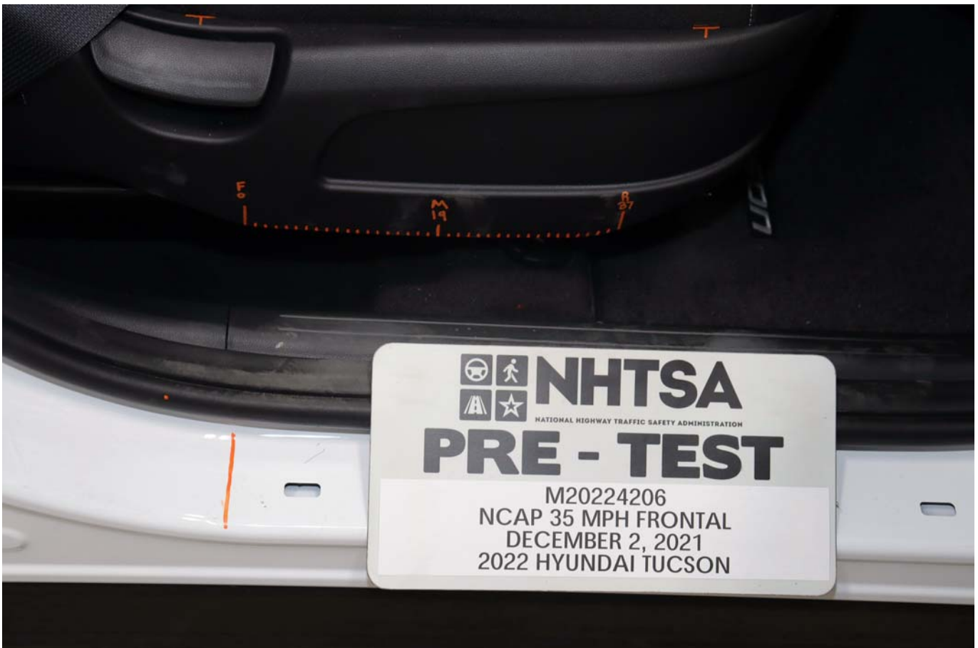
Photo No. 059 - Pre-Test Passenger's Seat Fore-Aft Markings
