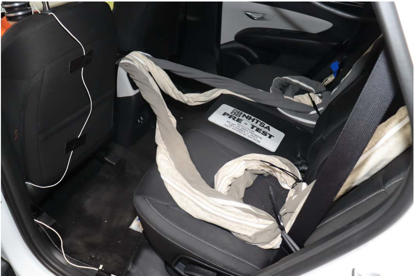
Photo No. 028 - Pre-Test Dummy Cable Routing
