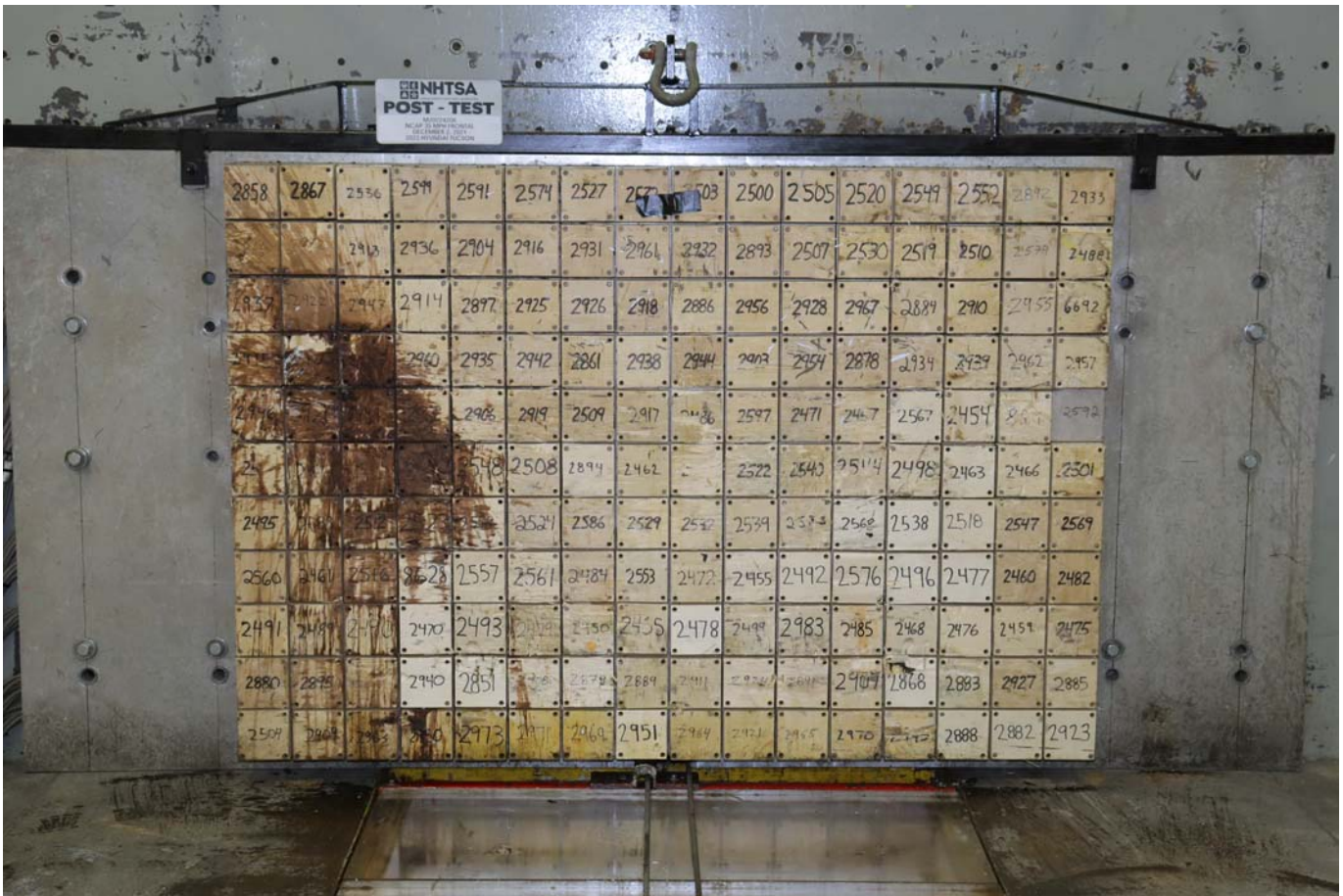
Photo No. 003 - Post-Test Load Cell Wall
