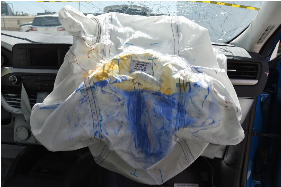
FIGURE 134. Post-Test Passenger Dummy Contact with Front Airbag
