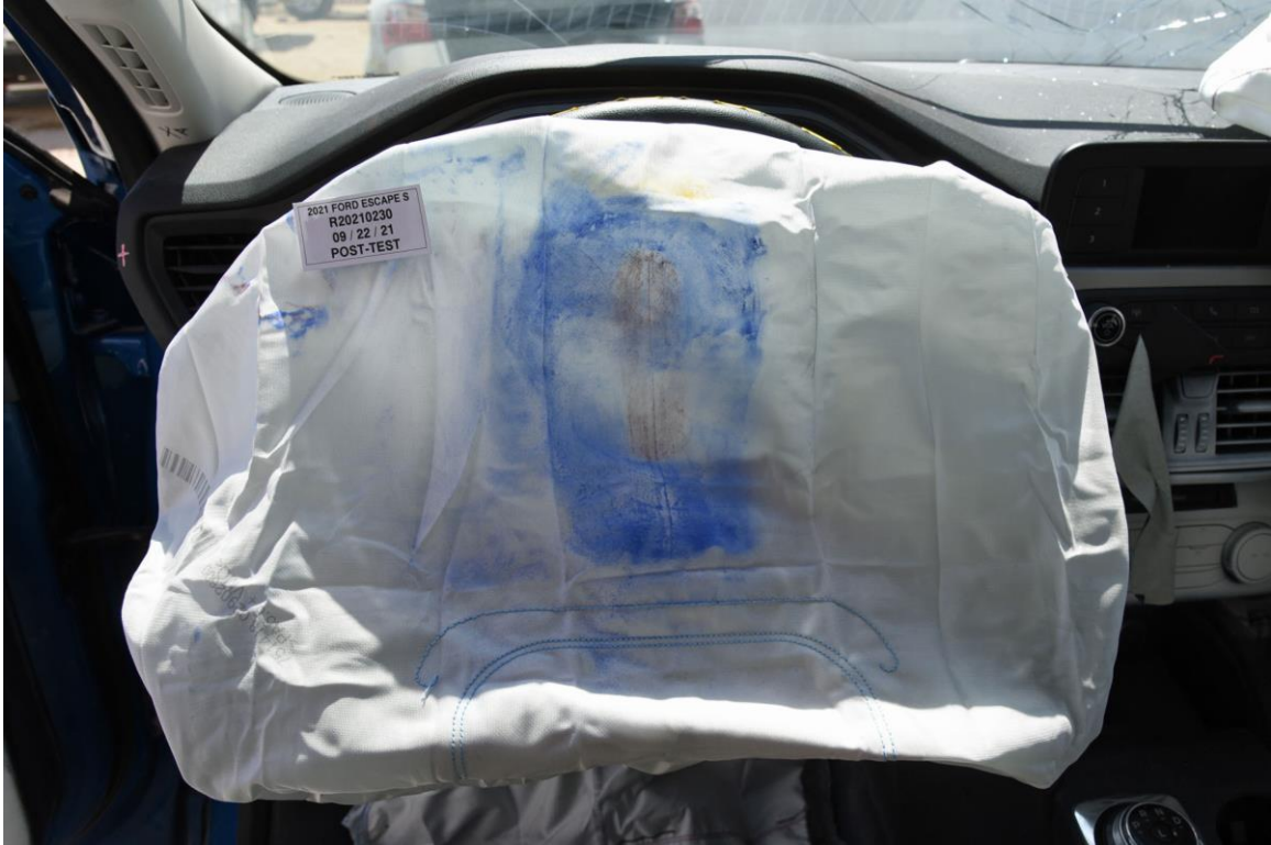
FIGURE 89. Post-Test Driver Dummy Contact with Front Airbag
