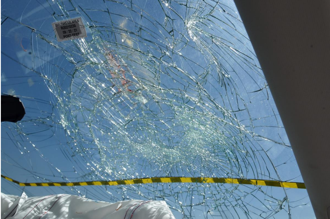
FIGURE 136a. Post-Test Passenger Dummy Contact with Windshield
