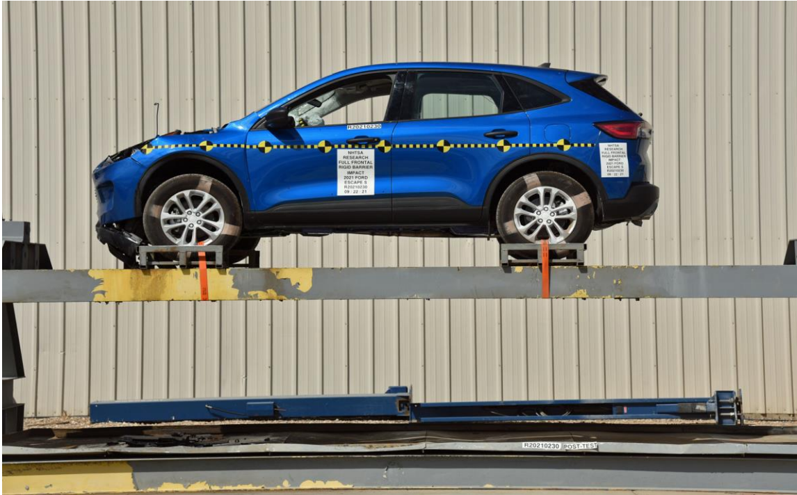
FIGURE 143. Vehicle at 360° on Static Rollover Device
