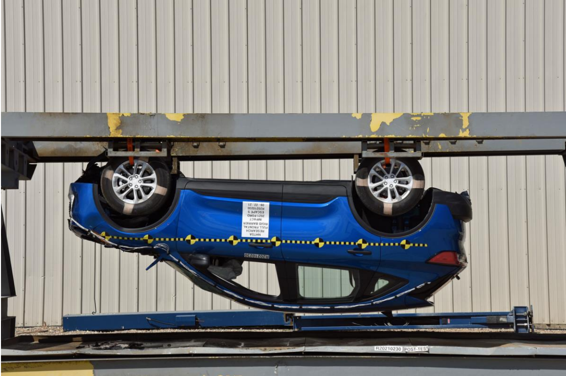
FIGURE 141. Vehicle at 180° on Static Rollover Device
