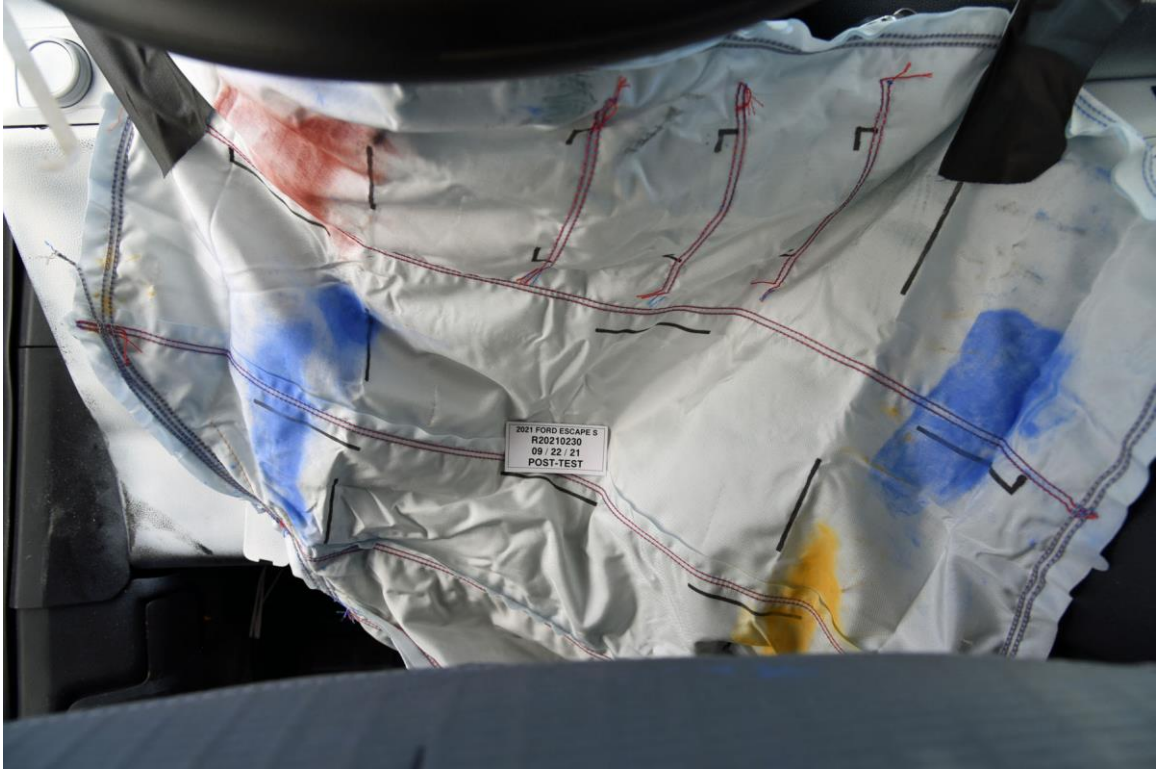
FIGURE 91. Post-Test Driver Dummy Contact with Knee Airbag
