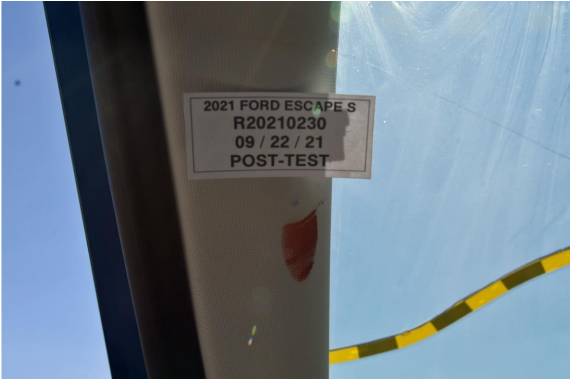
FIGURE 91a. Post-Test Driver Dummy Contact with A-Pillar
