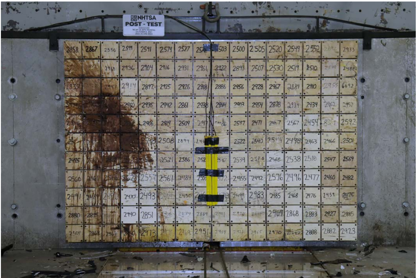
Photo No. 003 - Post-Test Load Cell Wall
