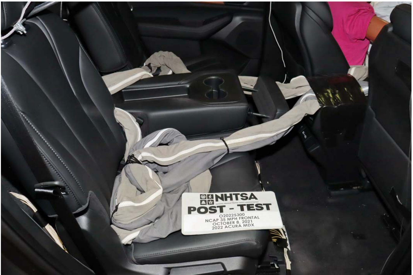
Photo No. 029 - Post-Test Dummy Cable Routing
