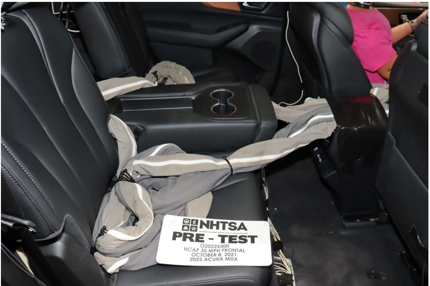
Photo No. 028 - Pre-Test Dummy Cable Routing
