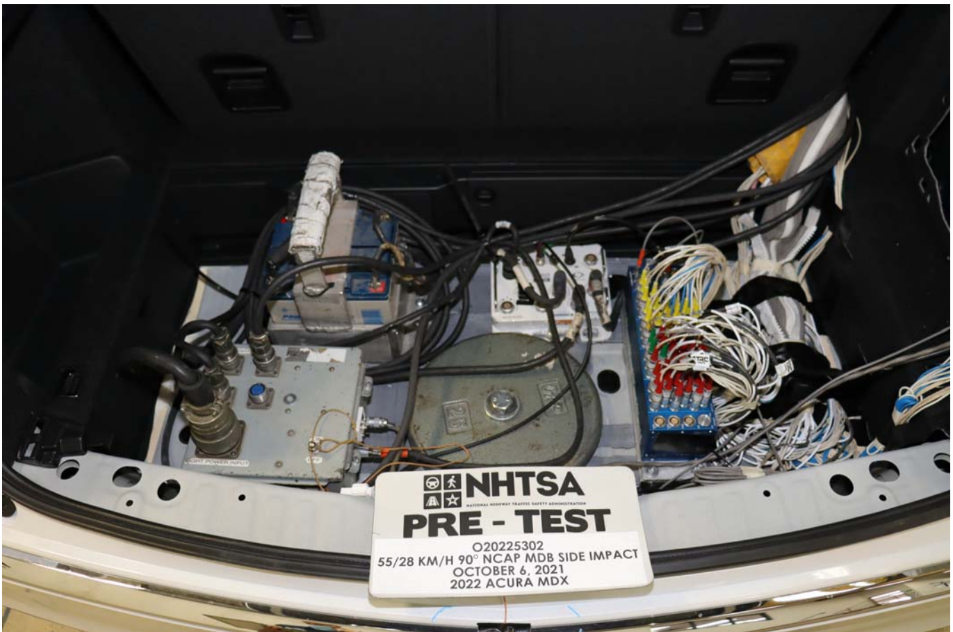
Photo No. 094 - Pre-Test Ballast View
