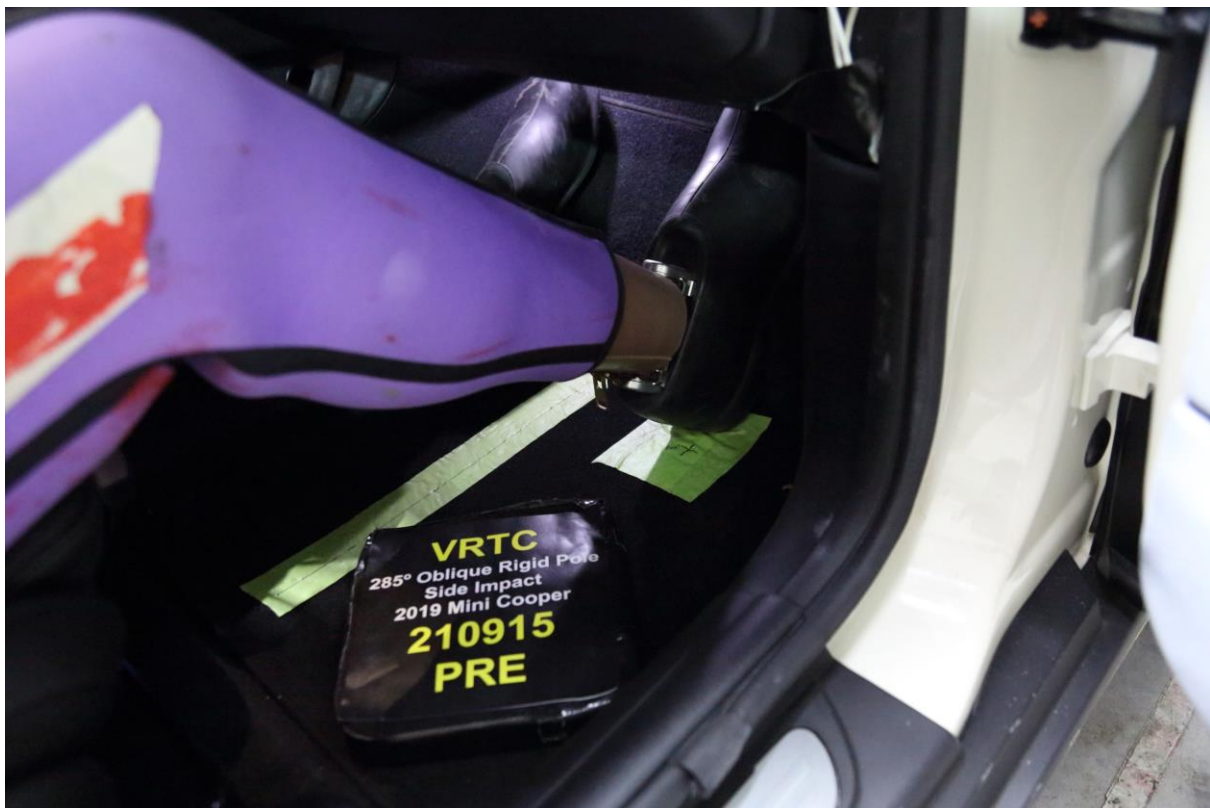
No. 032 Pre-Test Placement of Dummy Feet
