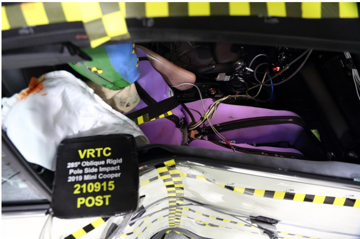
No. 041 Post-Test Dummy and Door Clearance View
