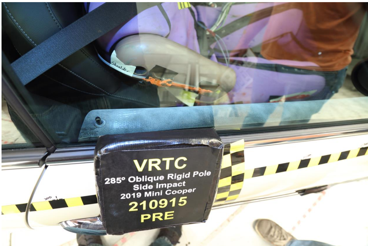
No. 040 Pre-Test Dummy and Door Clearance View
