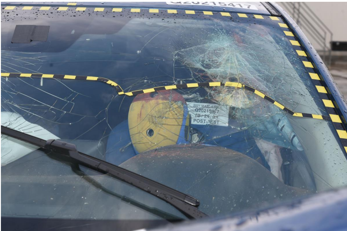
FIGURE 44. Post-Test Driver Front Windshield View
