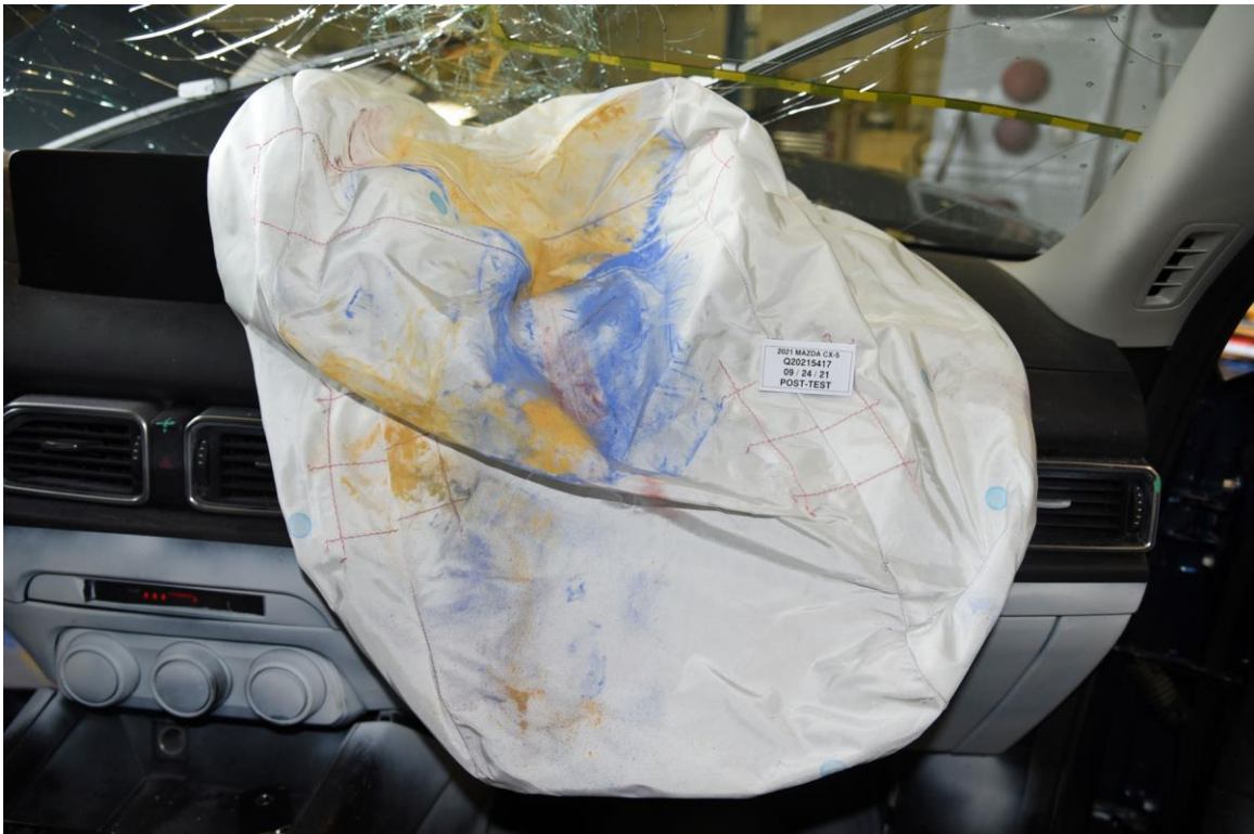
FIGURE 134. Post-Test Passenger Dummy Contact with Front Airbag
