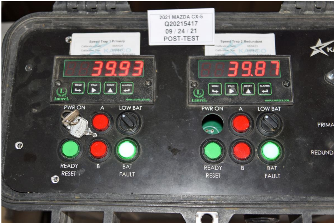
FIGURE 138. Post-Test Speed Trap Read-Out
