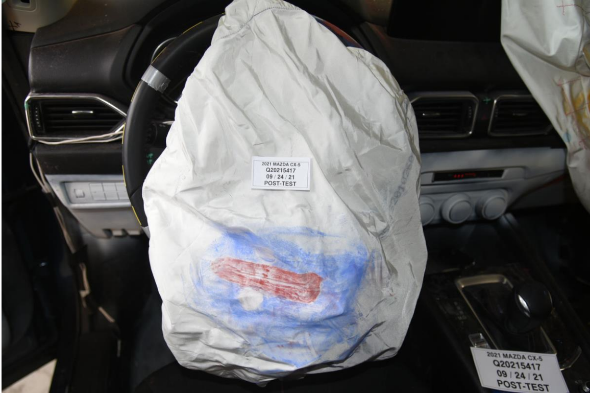
FIGURE 89. Post-Test Driver Dummy Contact with Front Airbag
