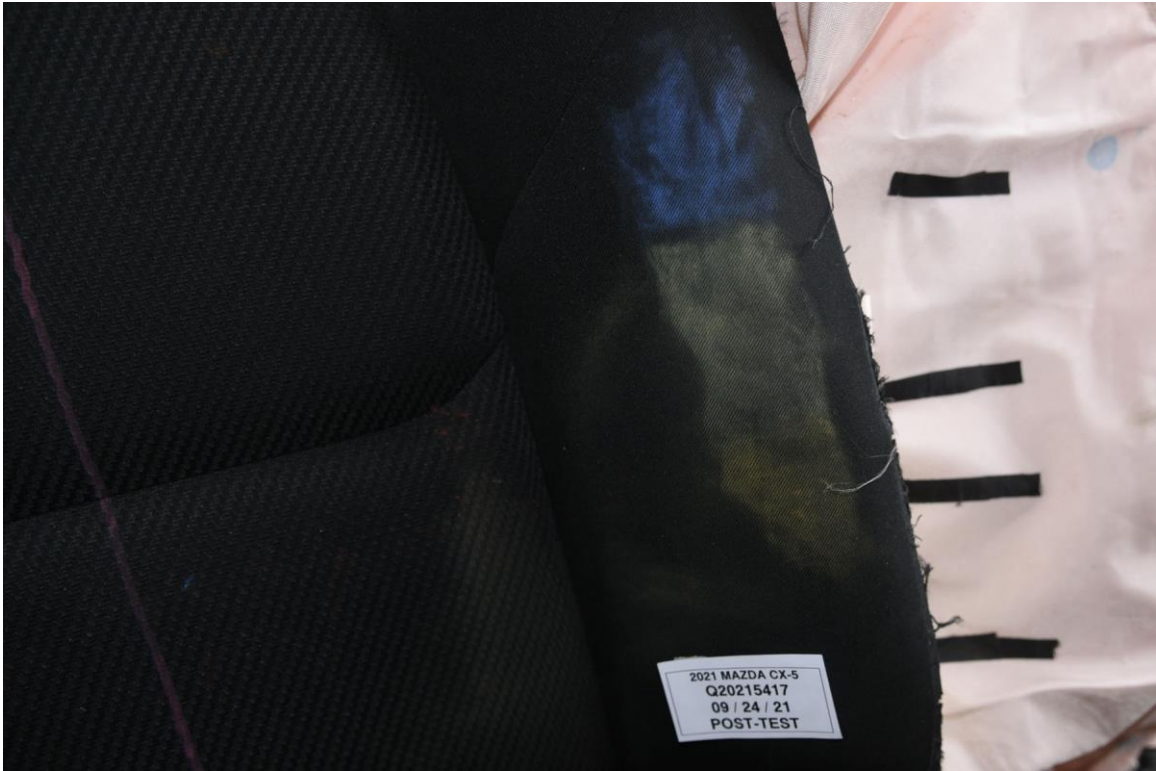
FIGURE 91b. Post-Test Driver Dummy Contact with Vehicle Interior
