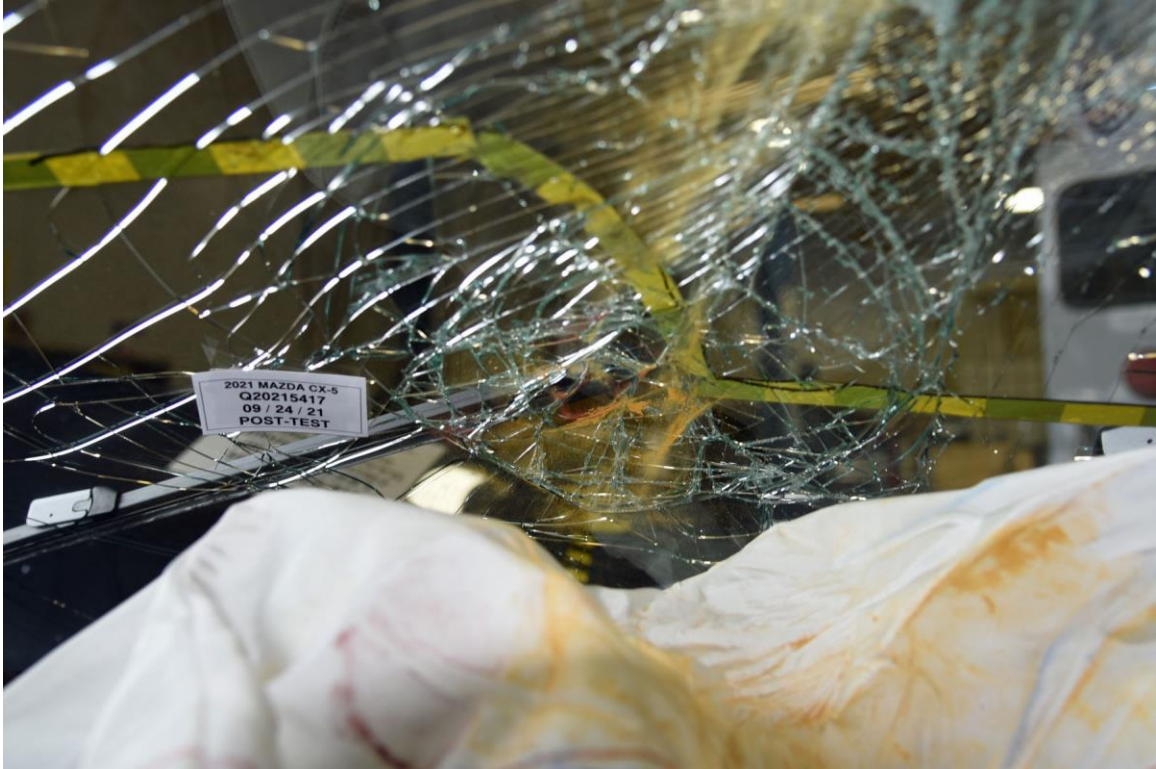
FIGURE 136a. Post-Test Passenger Dummy Contact with Windshield
