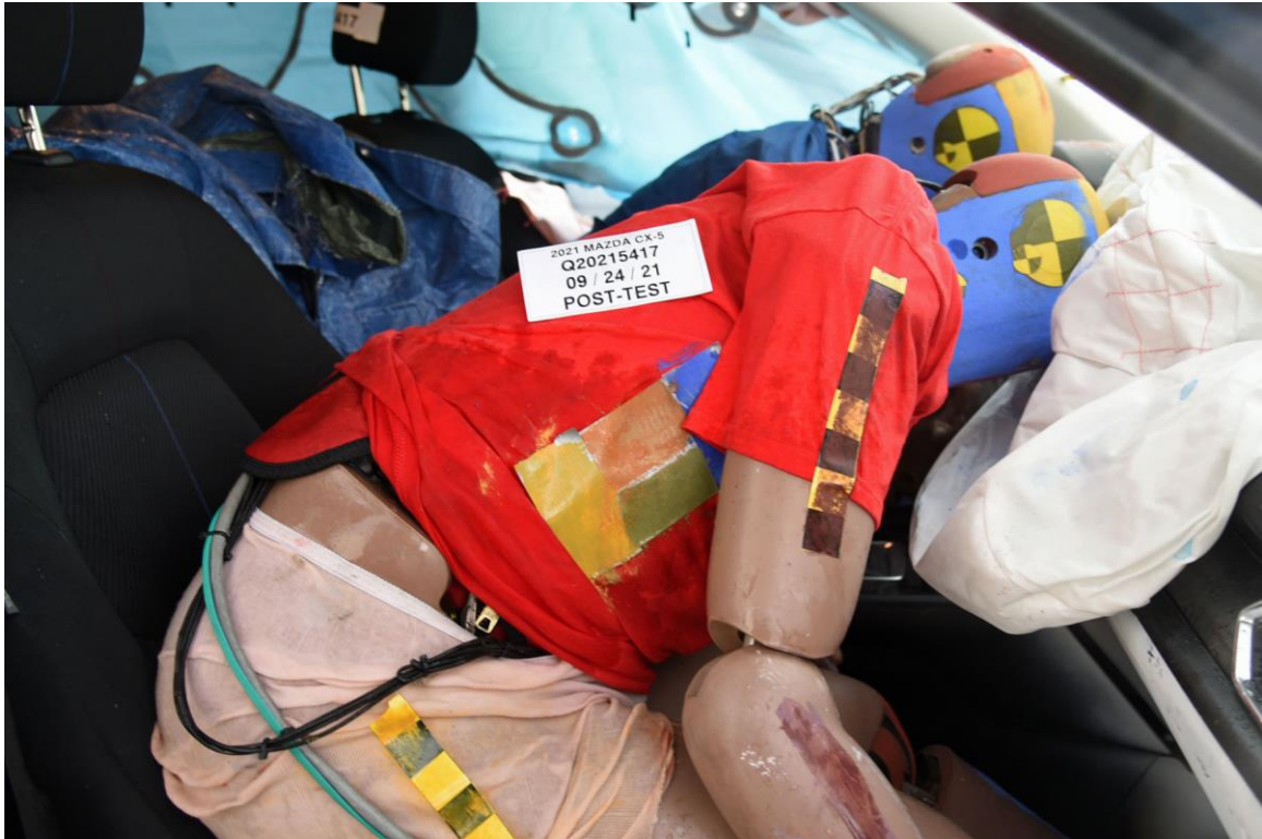
FIGURE 103. Post-Test View of Passenger Abdomen
