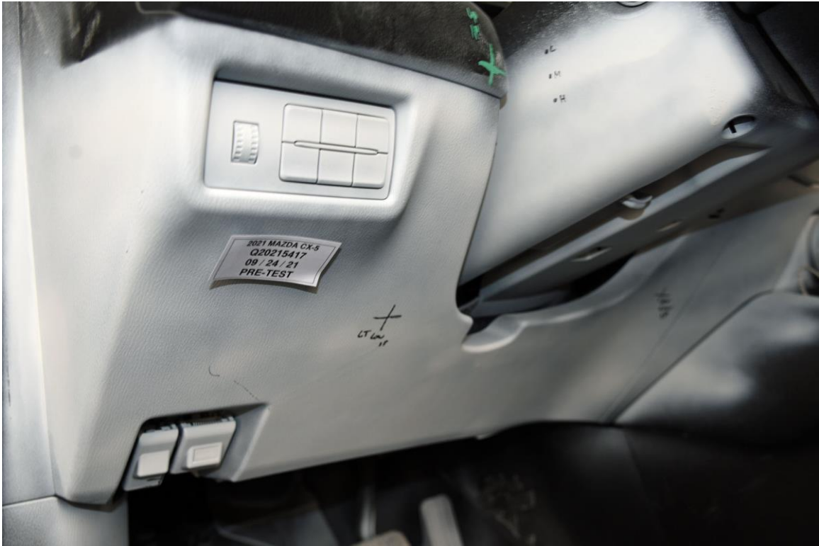
FIGURE 77. Pre-Test Left Side View of Driver Knee Bolster
