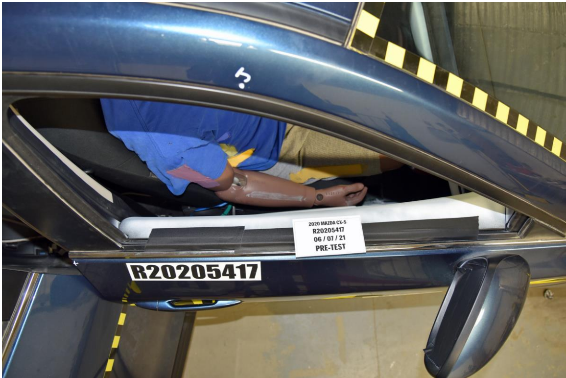
FIGURE 96. Pre-Test View of Passenger Door Clearance
