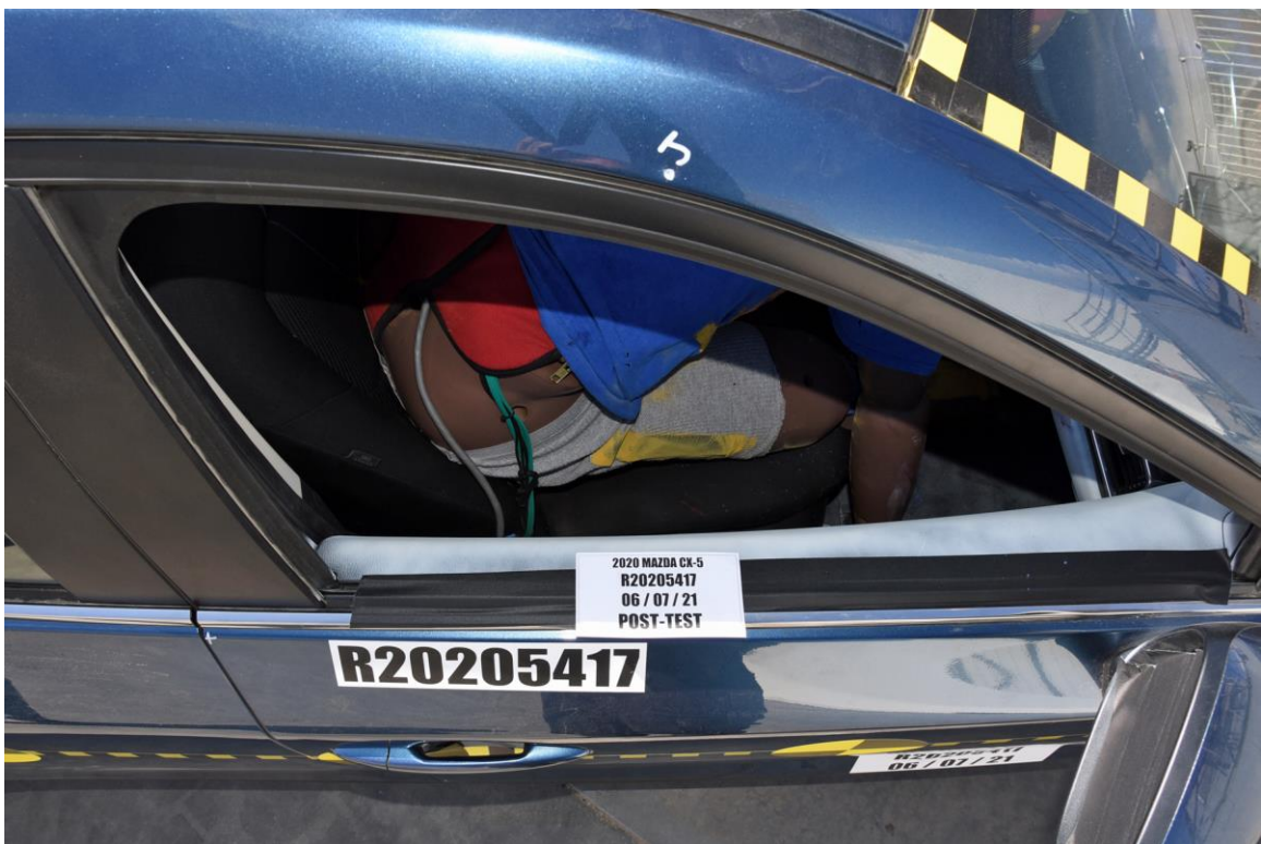
FIGURE 97. Post-Test View of Passenger Door Clearance
