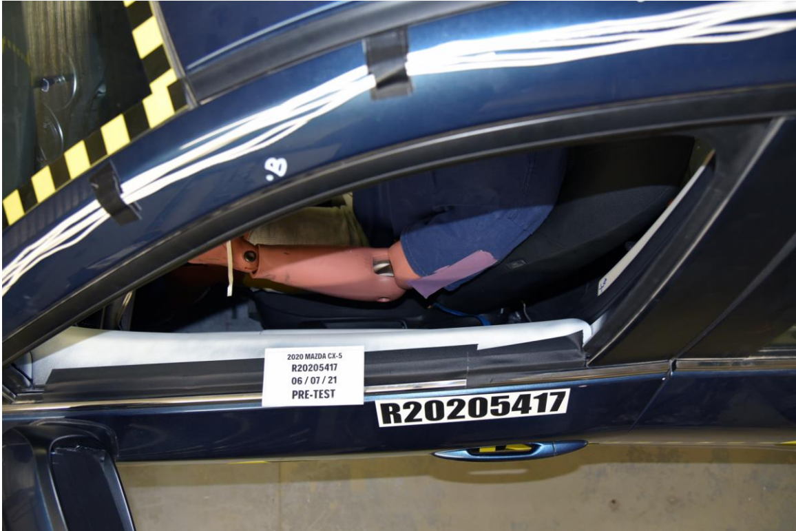
FIGURE 47. Pre-Test View of Driver Door Clearance
