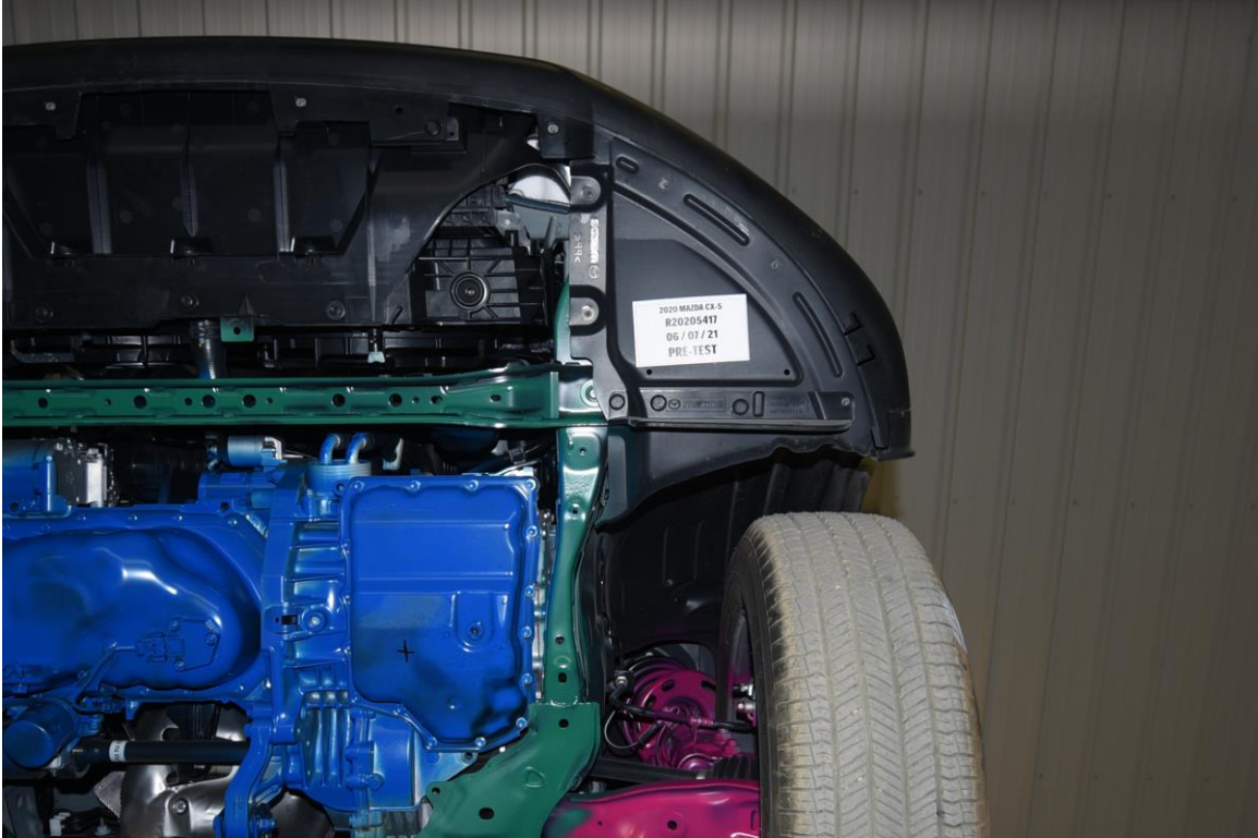
FIGURE 35. Pre-Test Driver Side Bumper to Rail Attachments and Crush Initiators
