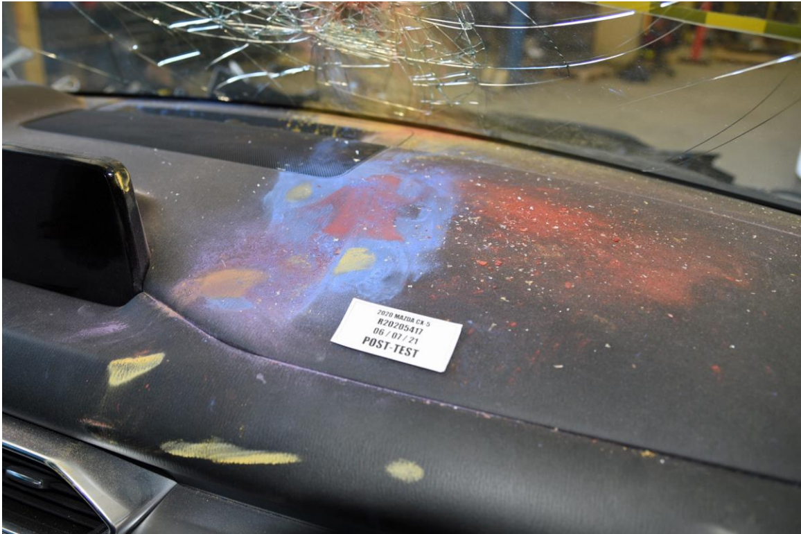
FIGURE 136b. Post-Test Passenger Dummy Contact with Dashboard
