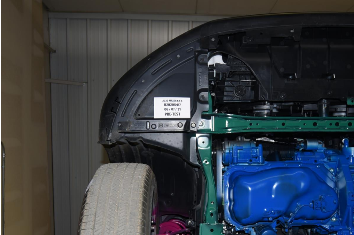
FIGURE 37. Pre-Test Passenger Side Bumper to Rail Attachments and Crush Initiators
