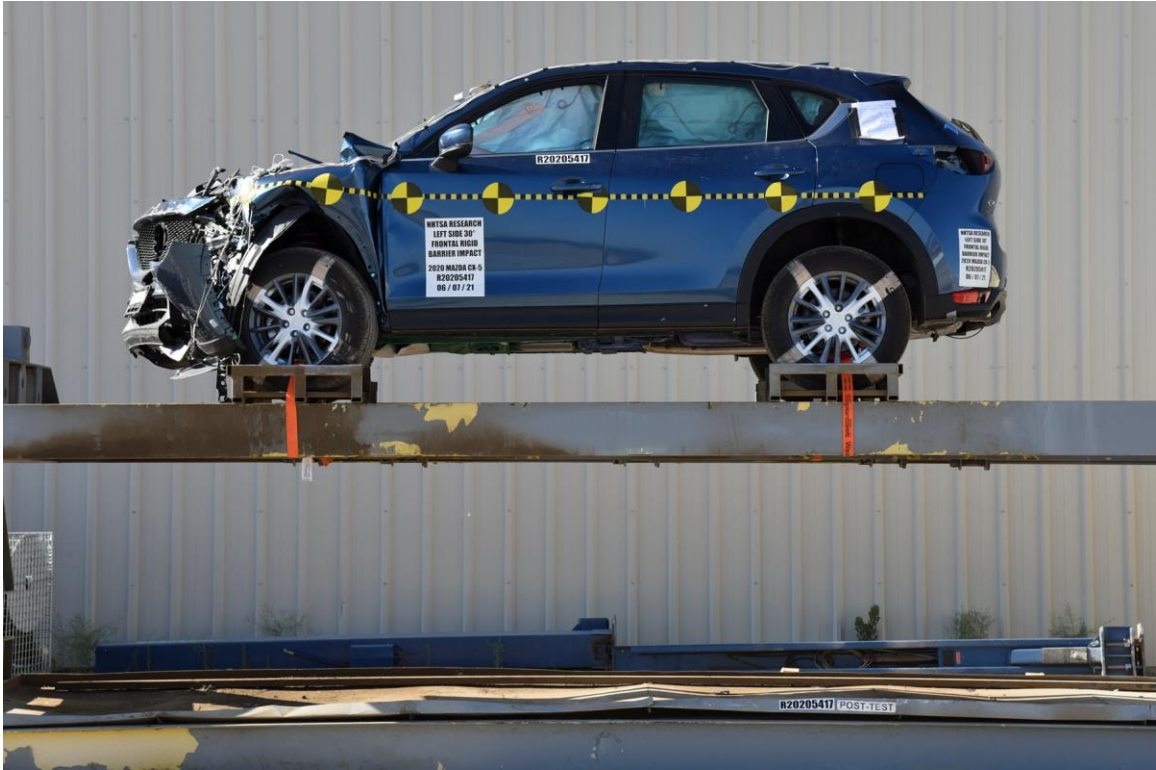
FIGURE 143. Vehicle at 360° on Static Rollover Device
