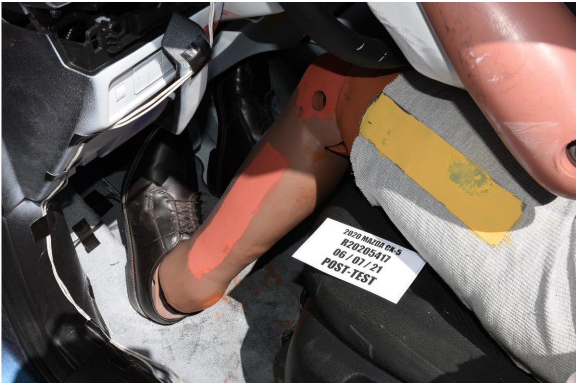
FIGURE 64. Post-Test View of the Driver Left Leg
