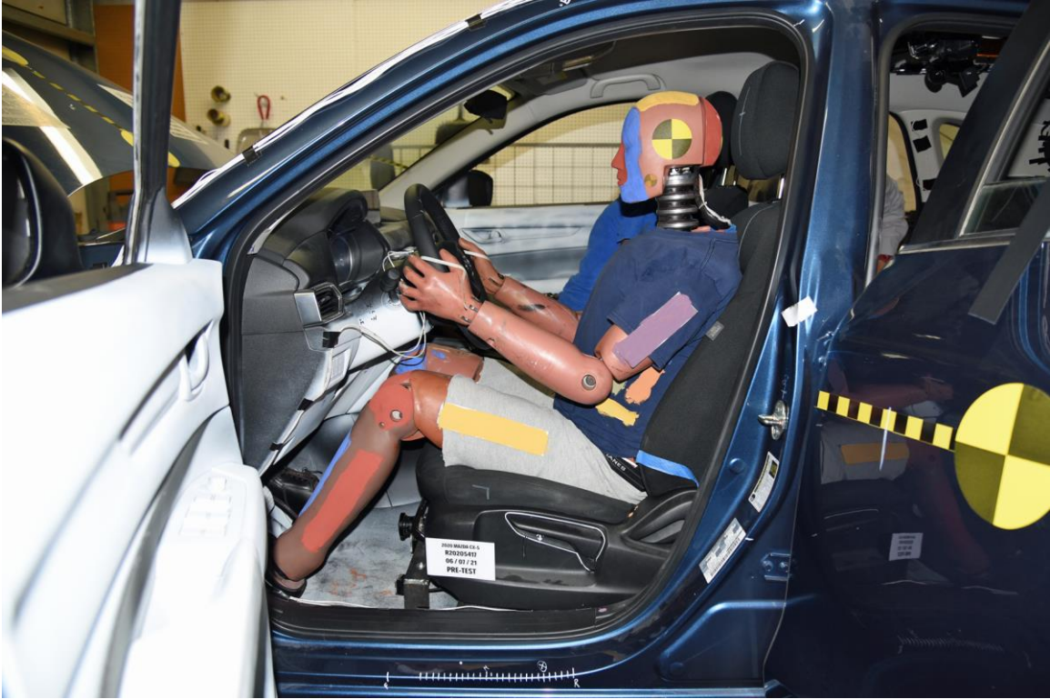
FIGURE 49. Pre-Test Left Side View of Driver and Interior
