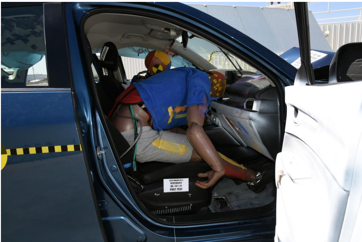
FIGURE 99. Post-Test Right Side View of Passenger and Interior
