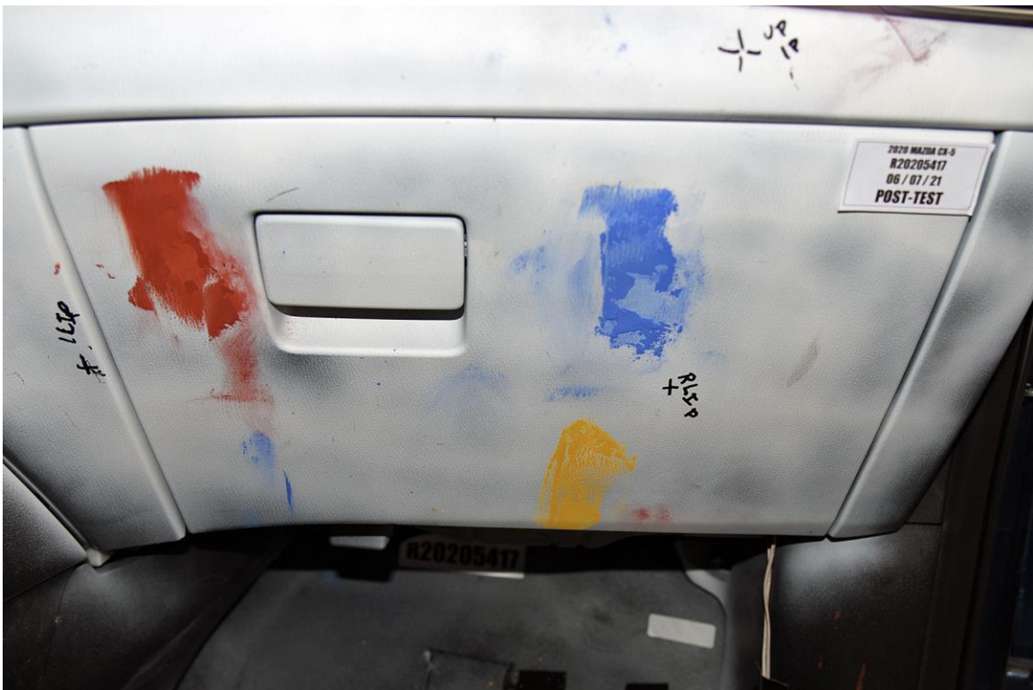
FIGURE 125. Post-Test Center View of Passenger Knee Bolster
