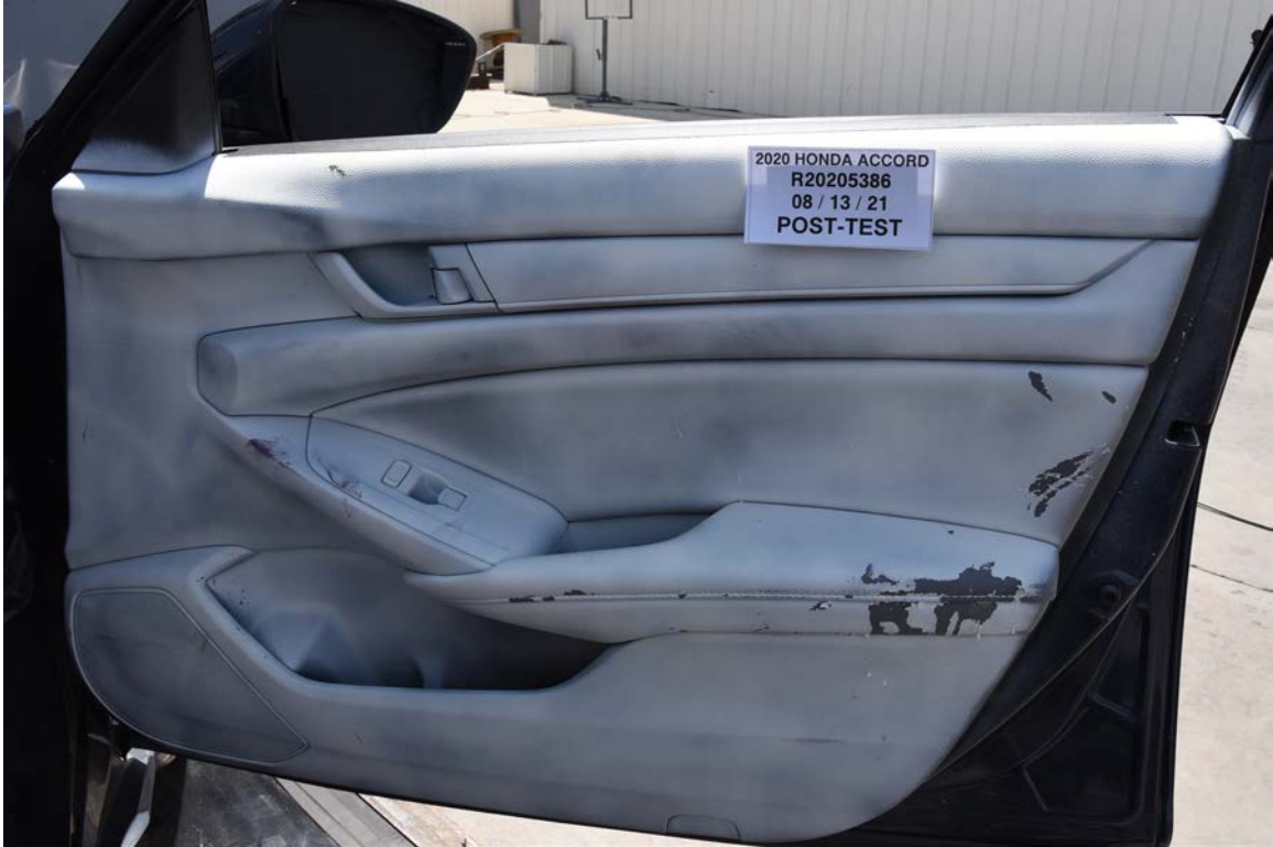
FIGURE 121. Post-Test Passenger Inner Door Panel
