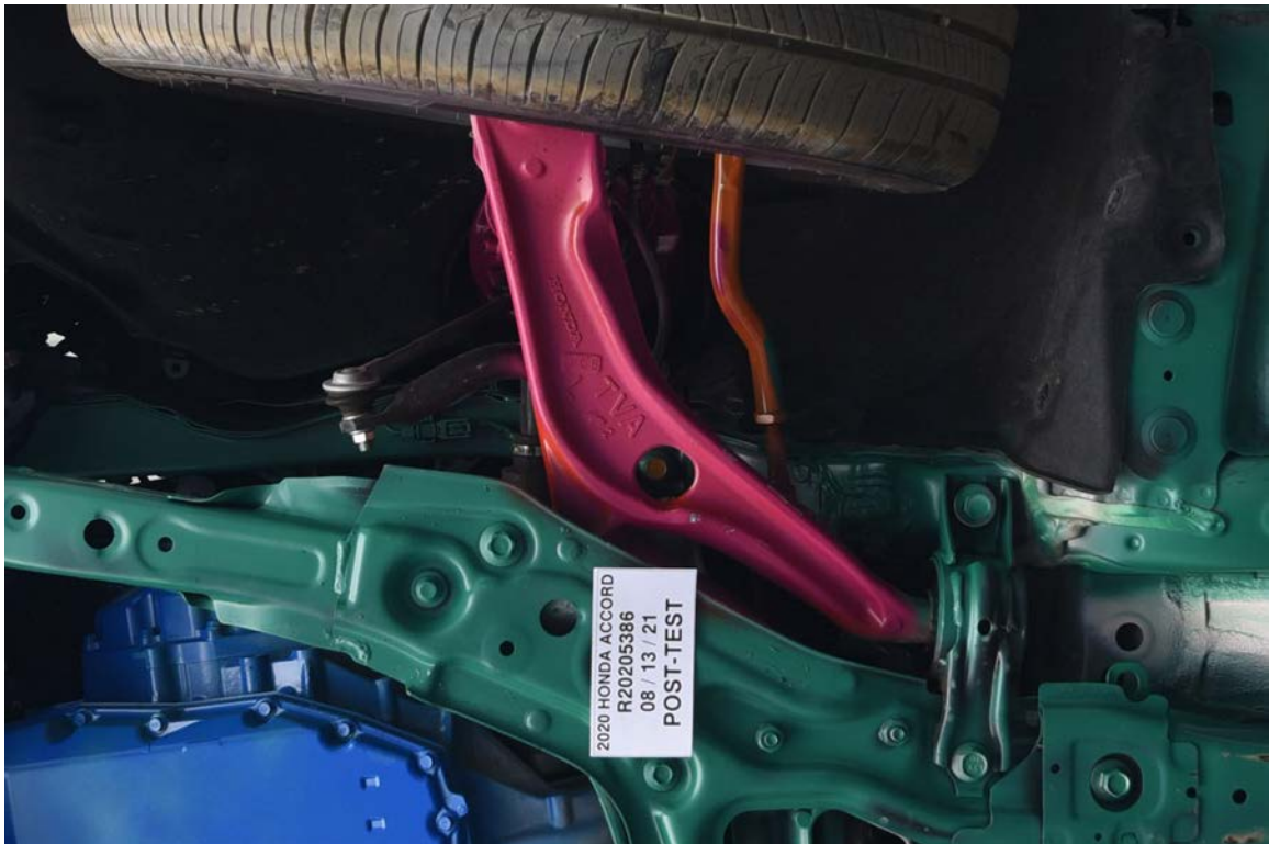
FIGURE 40. Post-Test Driver Side Rocker
