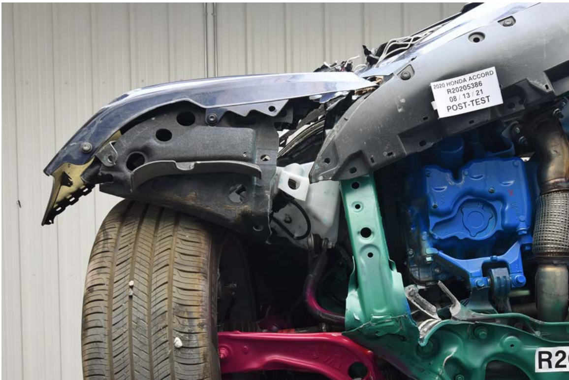
FIGURE 38. Post-Test Passenger Side Bumper to Rail Attachments and Crush Initiators
