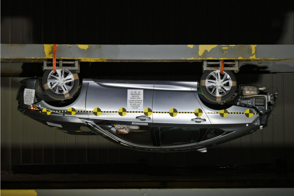
FIGURE 141. Vehicle at 180° on Static Rollover Device
