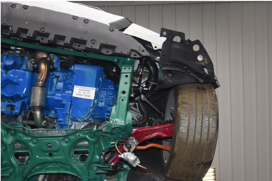
FIGURE 36. Post-Test Driver Side Bumper to Rail Attachments and Crush Initiators
