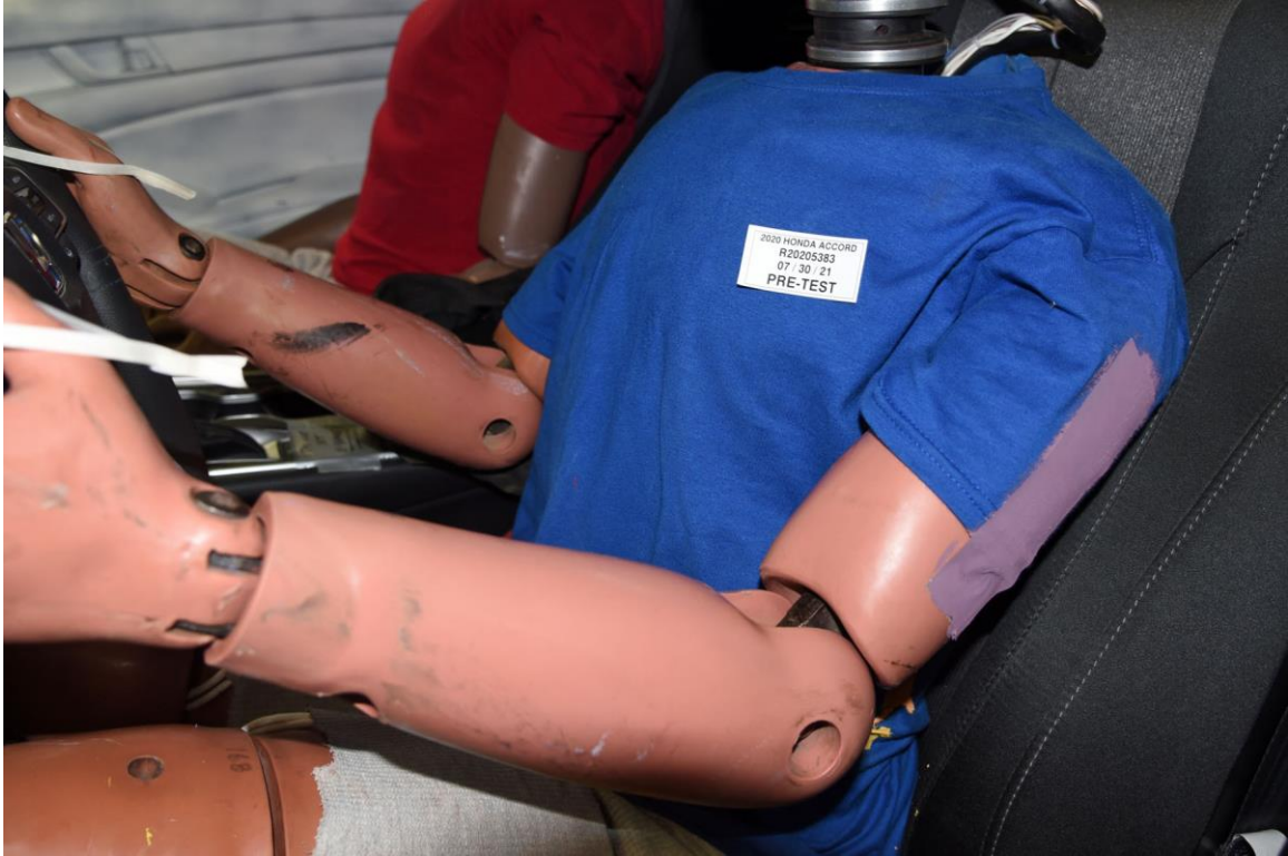
FIGURE 55. Pre-Test View of Driver Abdomen
