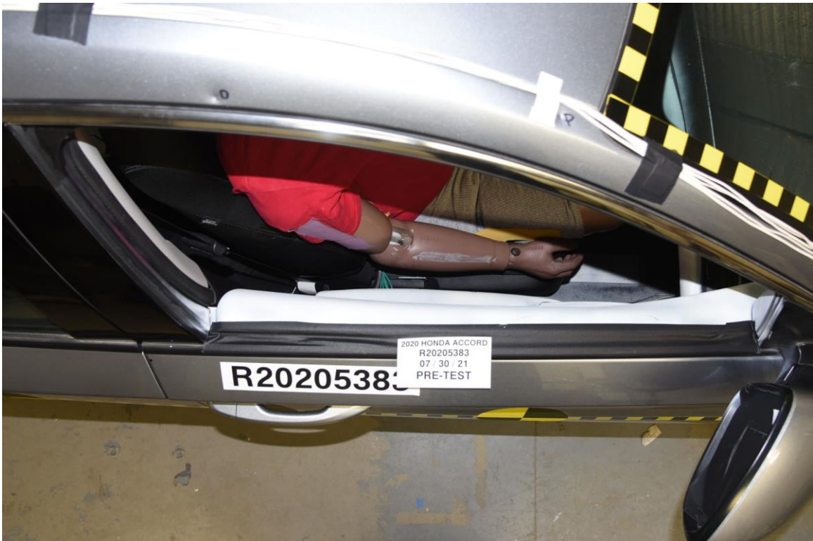
FIGURE 96. Pre-Test View of Passenger Door Clearance
