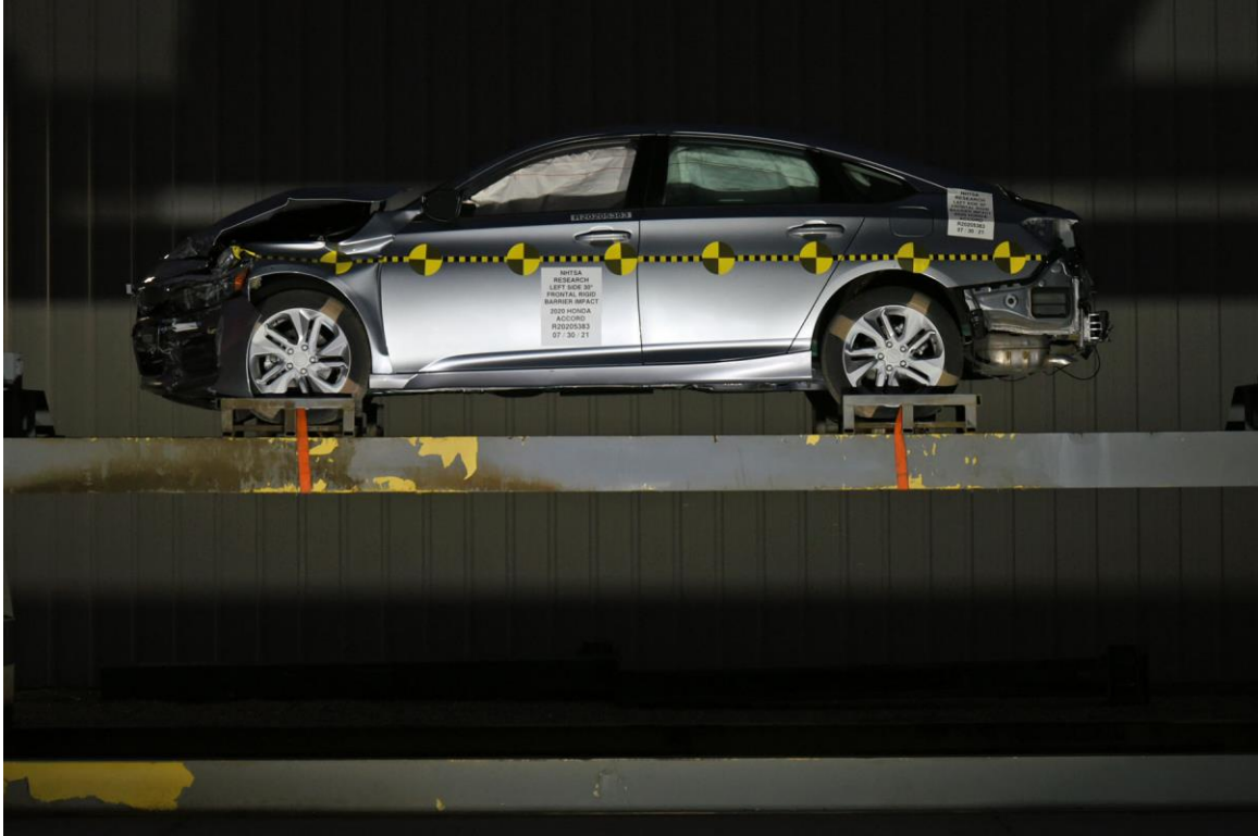
FIGURE 139. Vehicle at 0° on Static Rollover Device
