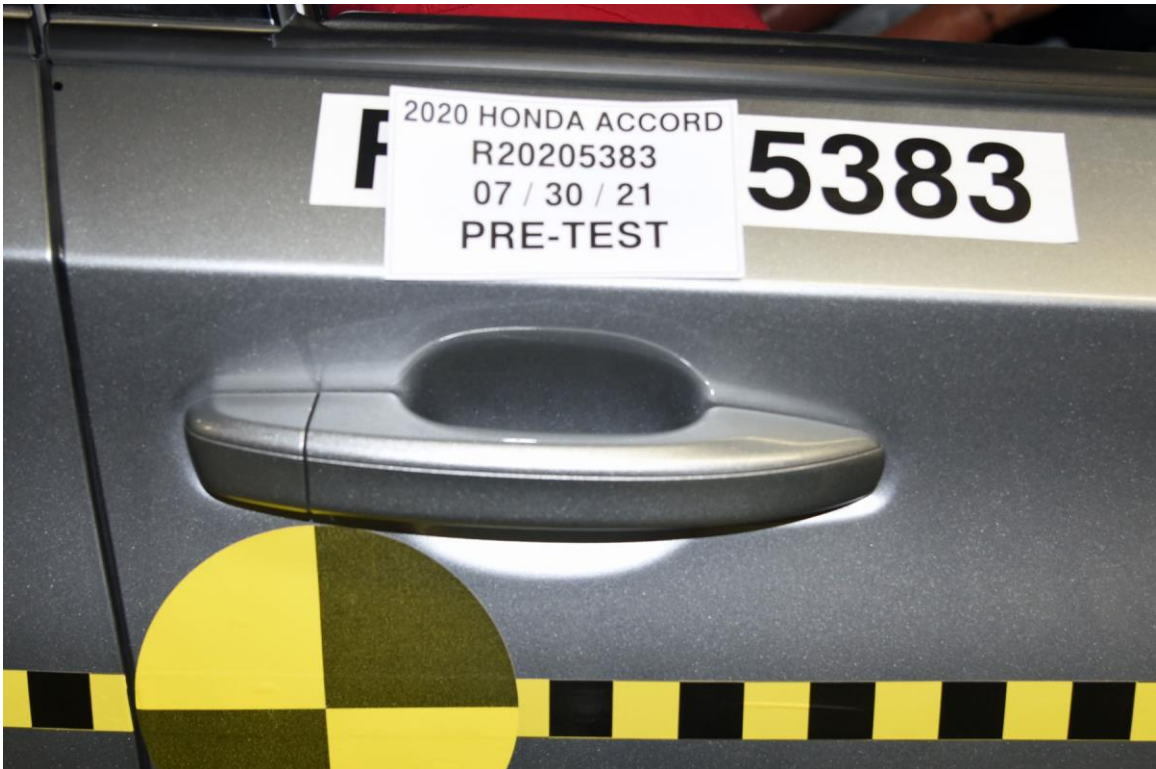
FIGURE 118. Pre-Test Close-up View of Passenger Door Latch
