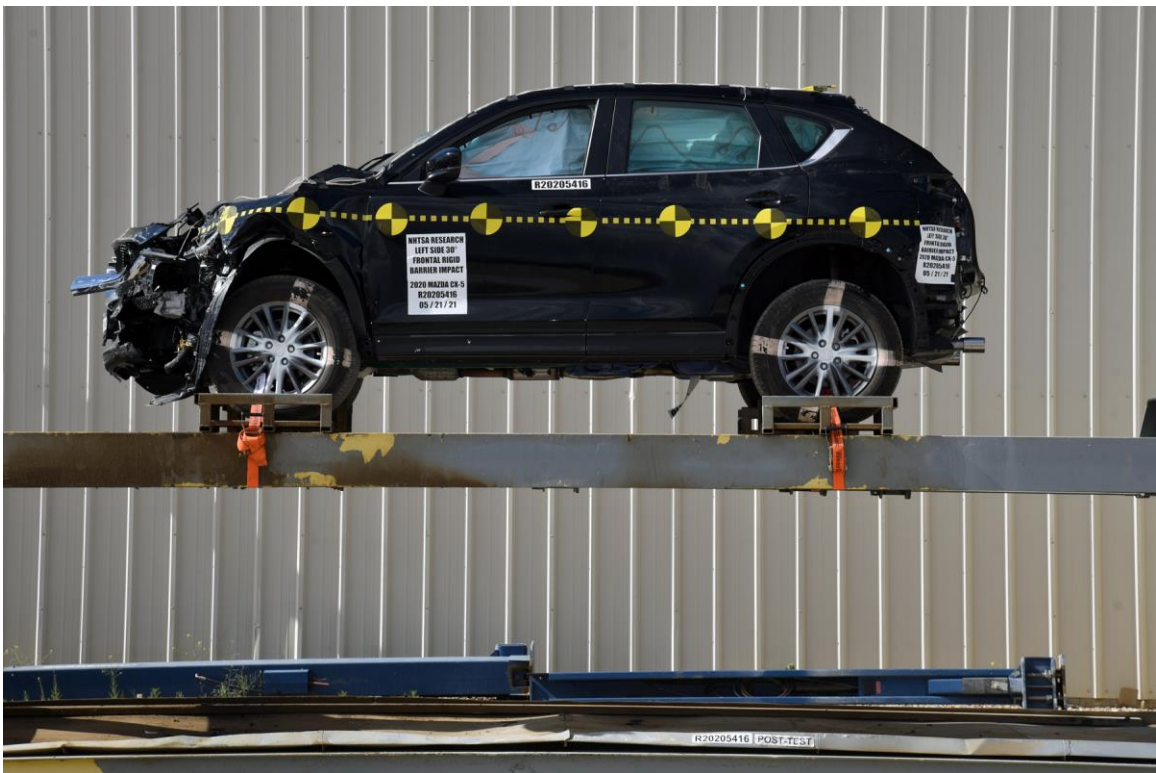
FIGURE 144. Vehicle at 360° on Static Rollover Device
