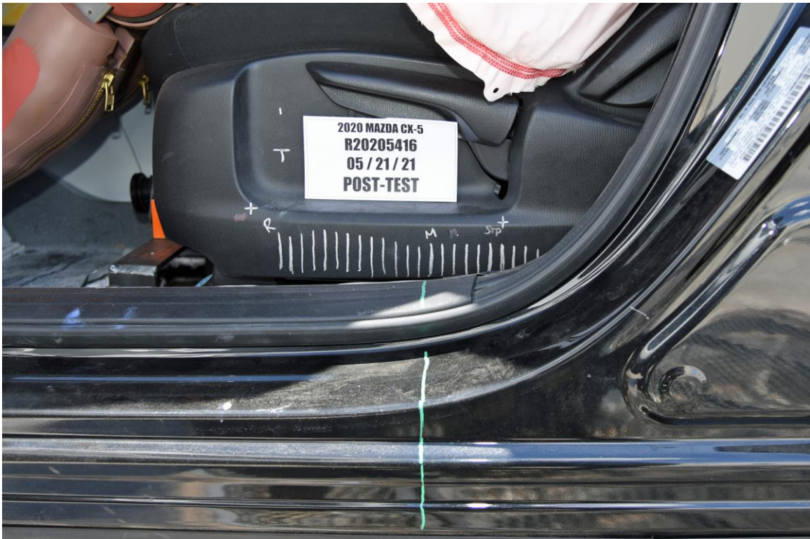
FIGURE 70. Post-Test Driver Seat Fore-Aft Markings
