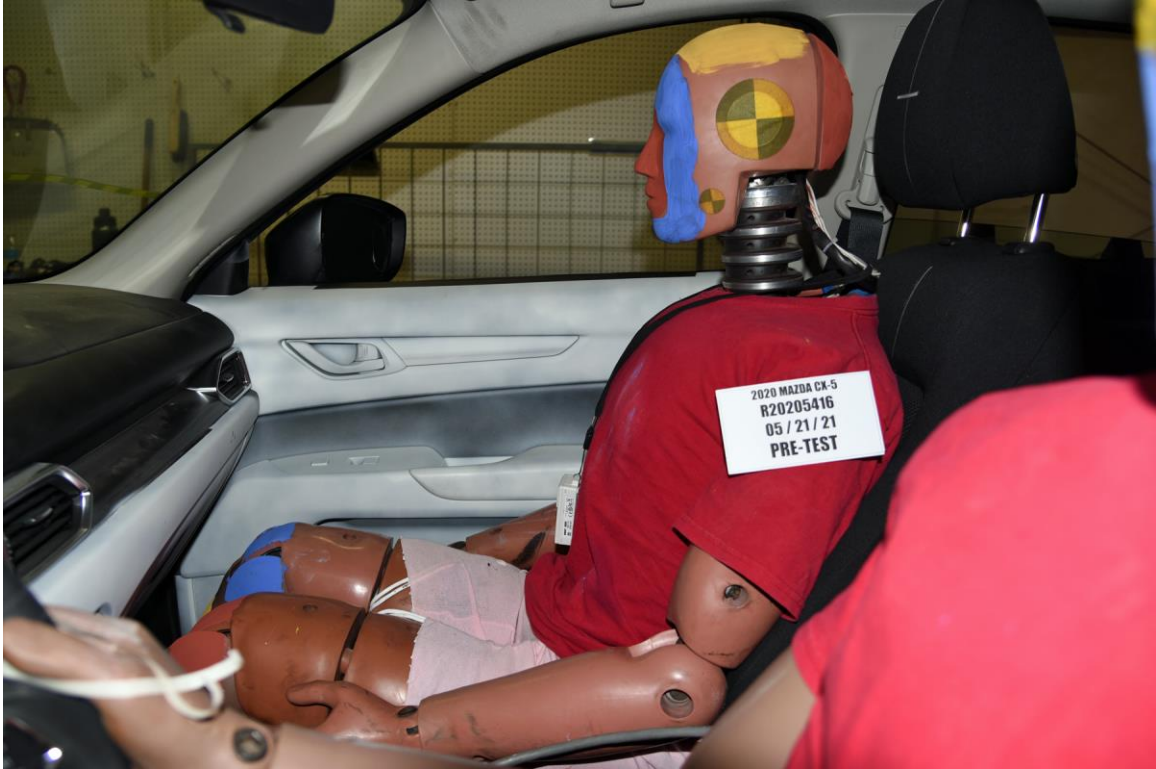
FIGURE 104. Pre-Test Left Side Passenger and Interior View
