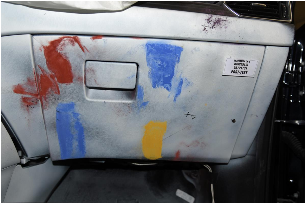
FIGURE 125. Post-Test Center View of Passenger Knee Bolster
