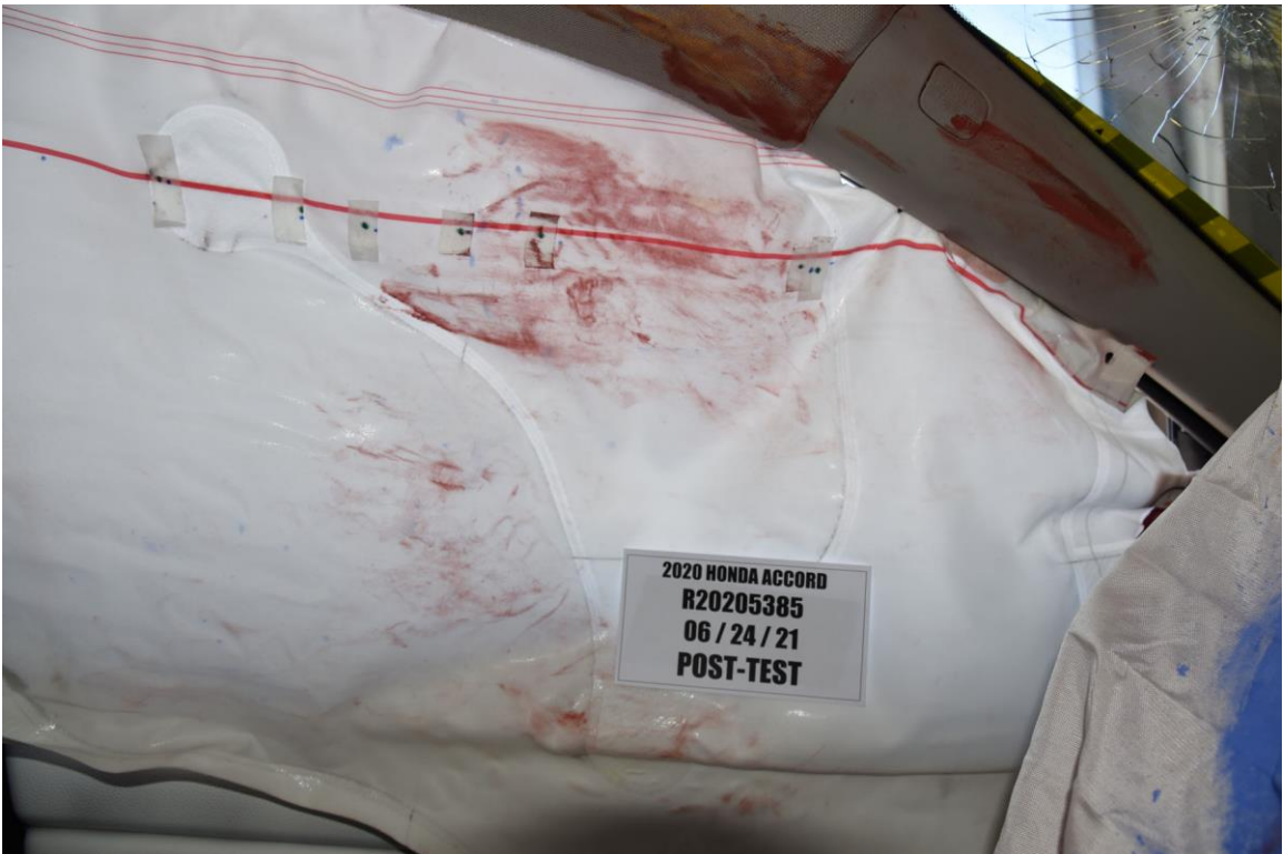
FIGURE 90. Post-Test Driver Dummy Contact with Side Airbag
