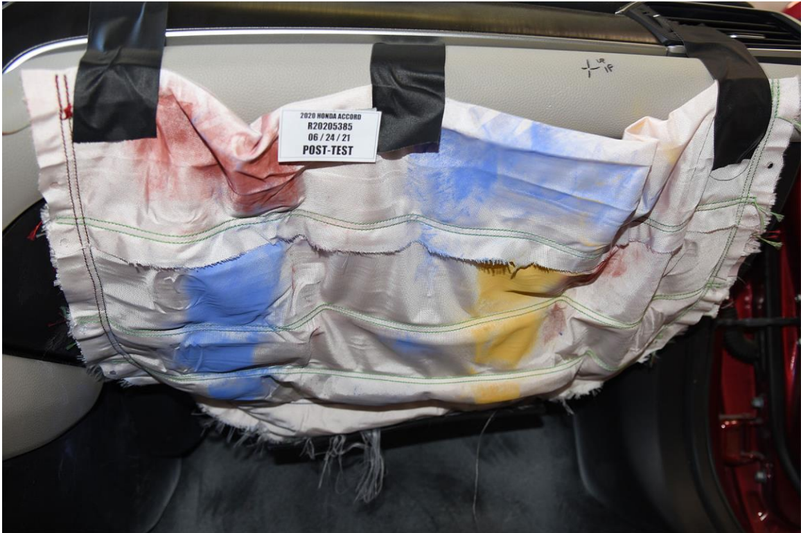
FIGURE 136. Post-Test Passenger Dummy Contact with Knee Airbag
