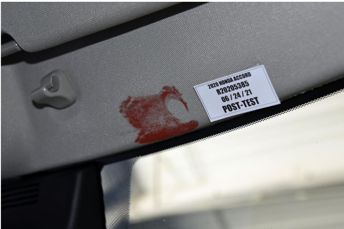
FIGURE 136a. Post-Test Passenger Dummy Contact with Headliner
