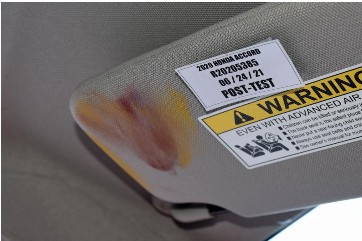
FIGURE 91a. Post-Test Driver Dummy Contact with Headliner and Visor
