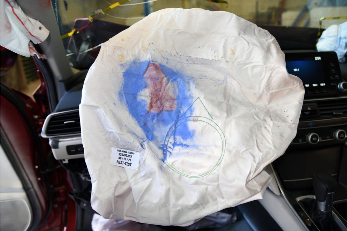
FIGURE 89. Post-Test Driver Dummy Contact with Front Airbag
