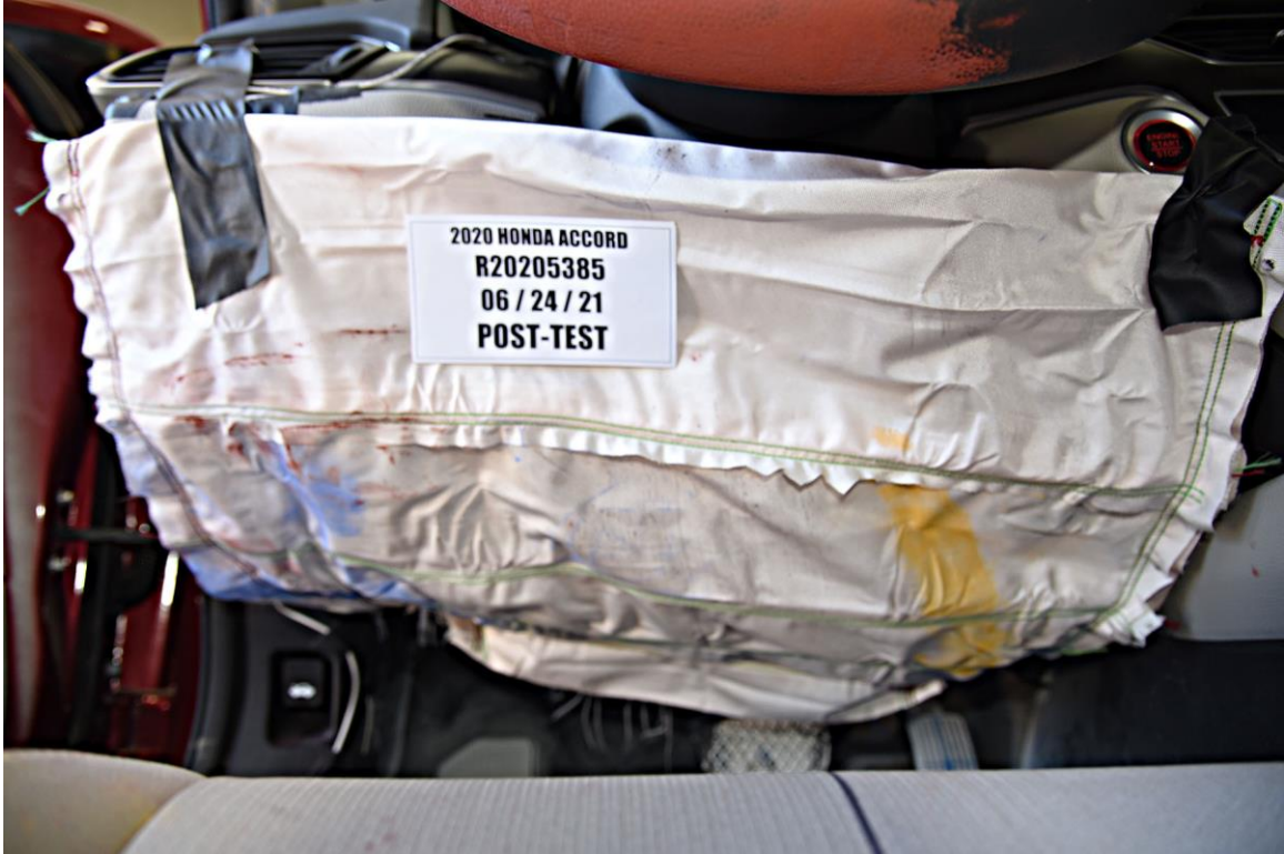
FIGURE 91. Post-Test Driver Dummy Contact with Knee Airbag
