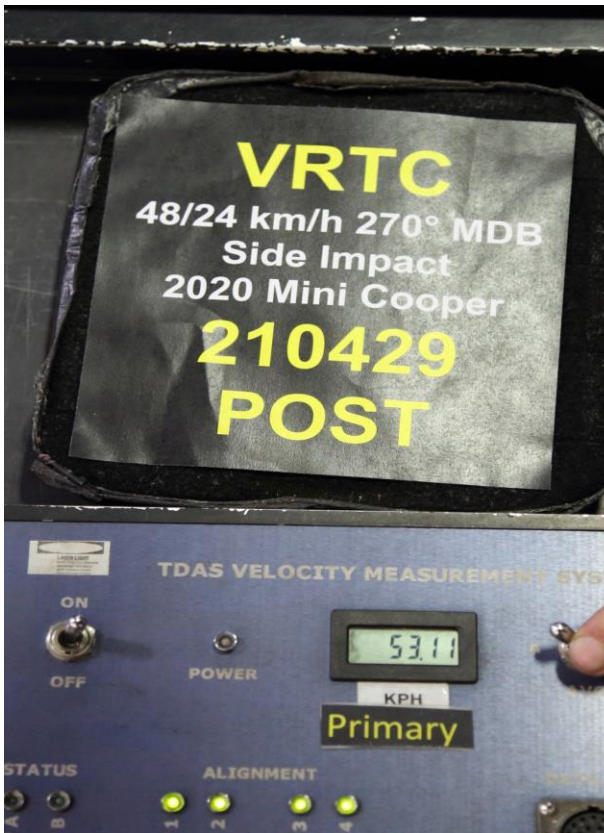
095 Post-Test Primary and Redundant Speed Trap Read-Out
