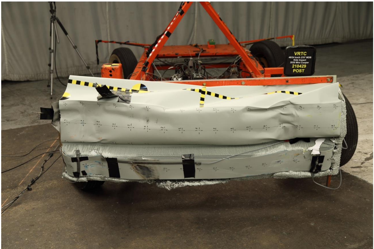
085 Post-Test Front View of MDB Impactor Face
