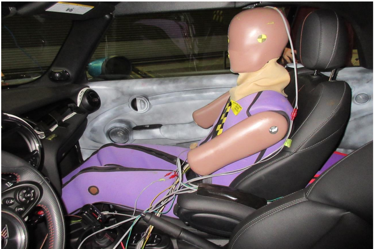
044 Pre-Test Left Side View of Passenger Dummy and Front Seat of Occupant Compartment
