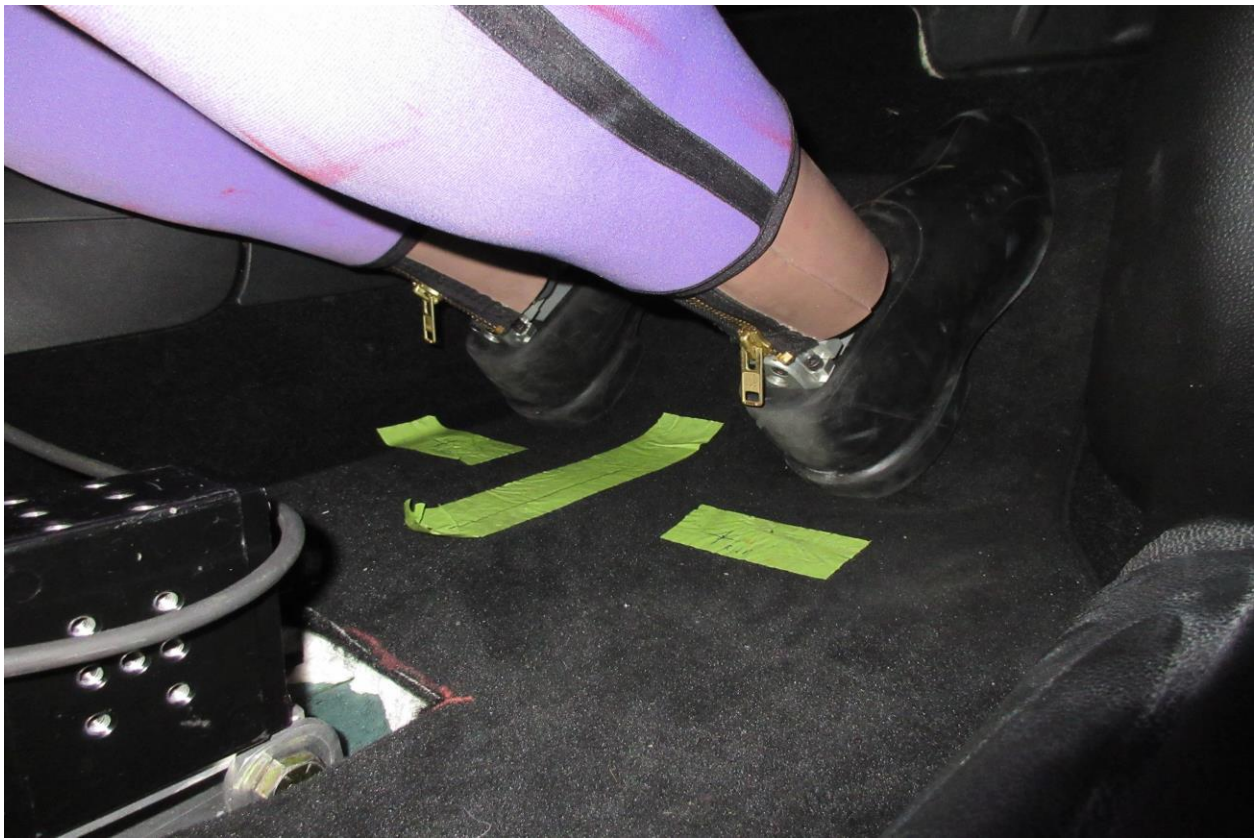
034 Pre-Test Placement of Passenger Dummy's Feet
