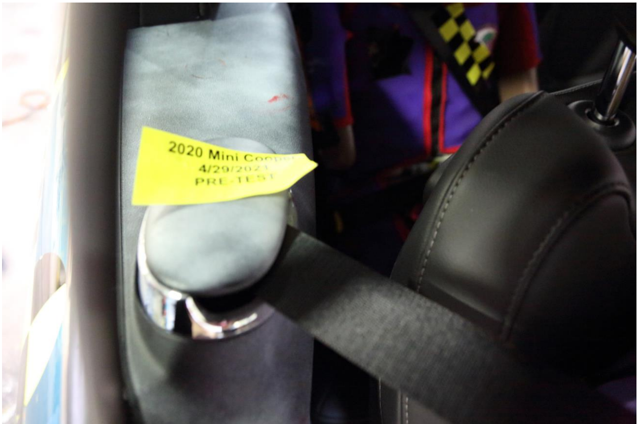
035 Pre-Test View of Belt Anchorage for Passenger Dummy
