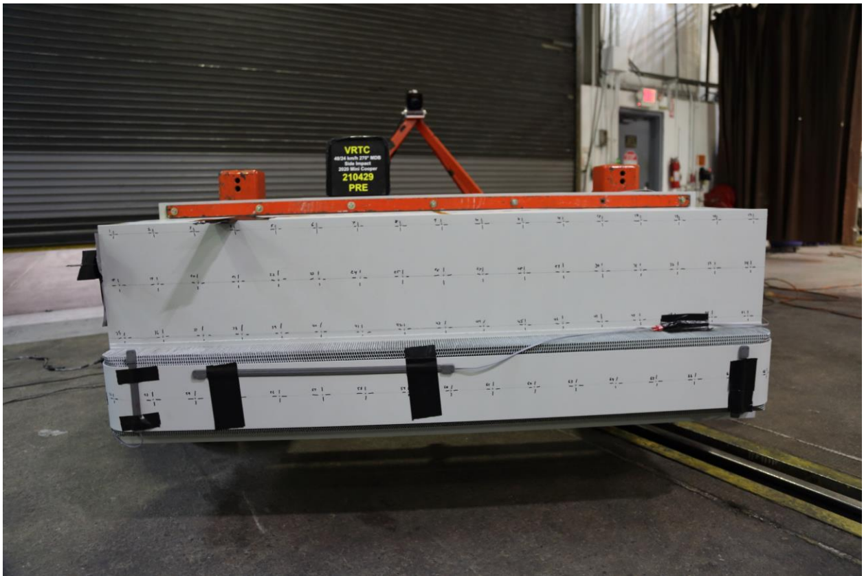
084 Pre-Test Front View of MDB Impactor Face
