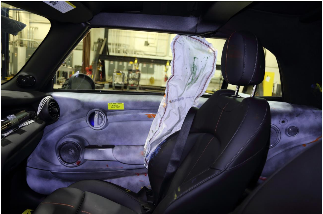
047 Post-Test Passenger Inner Door Panel View Showing Passenger Dummy Contact Locations
