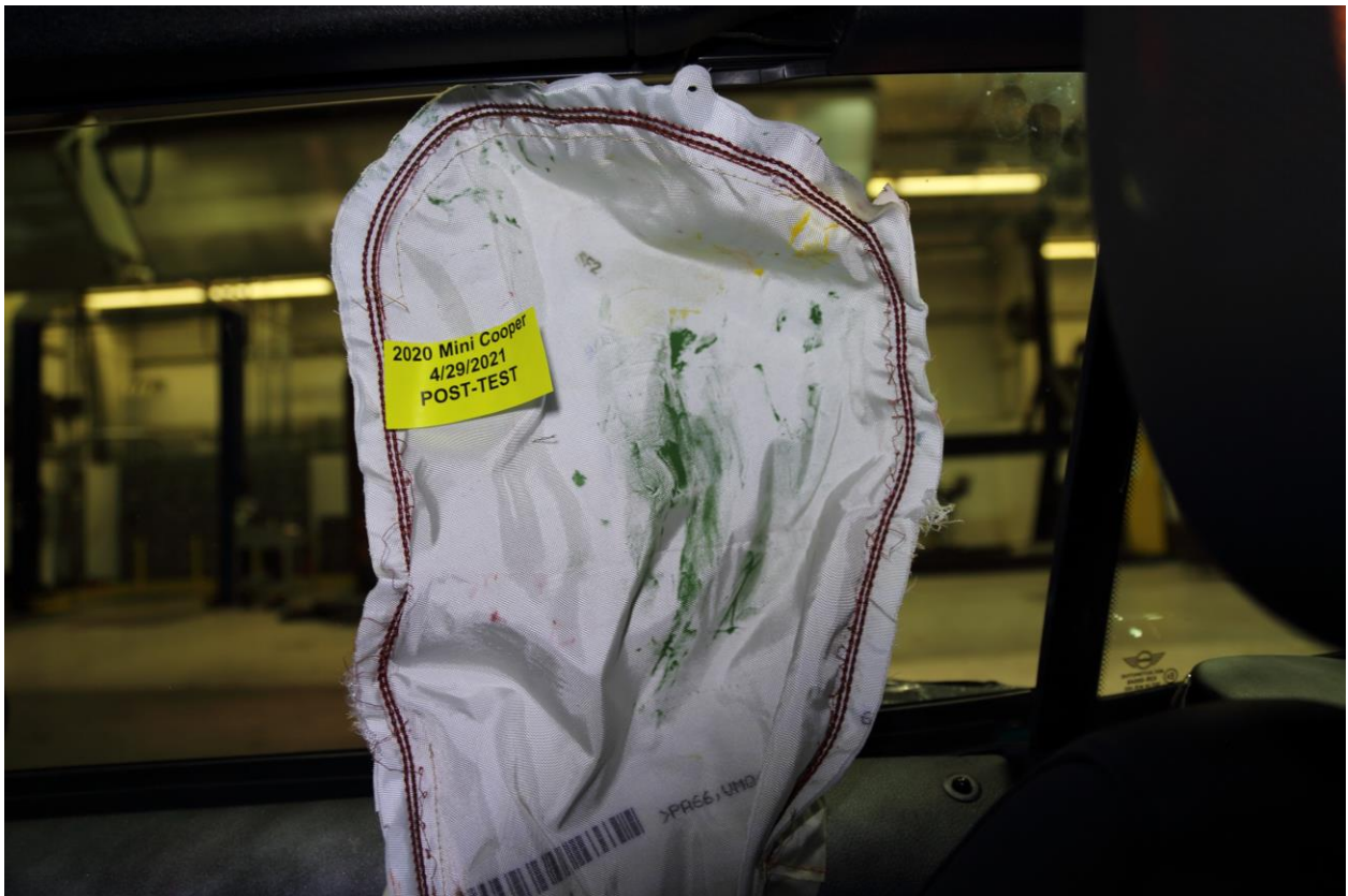
049 Post-Test Passenger Dummy Close-Up Head Contact with Side Airbag View
