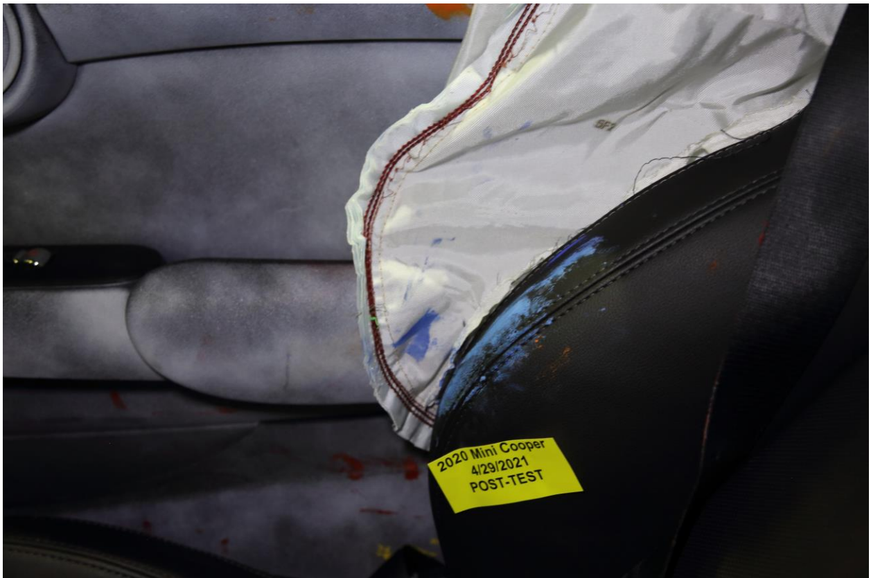
051 Post-Test Passenger Dummy Close-Up Torso Contact with Side Airbag View
