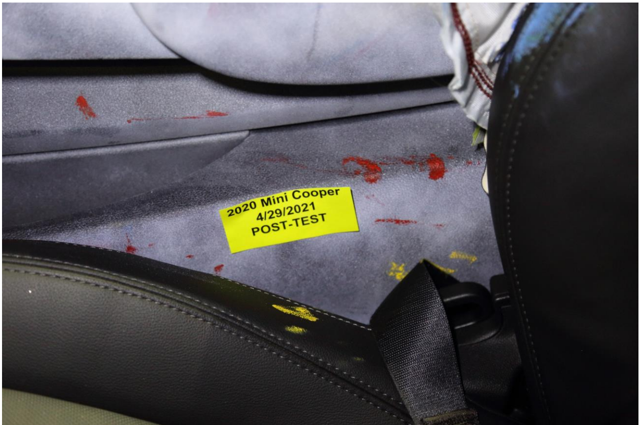
052 Post-Test Passenger Dummy Close-Up Pelvis Contact View
