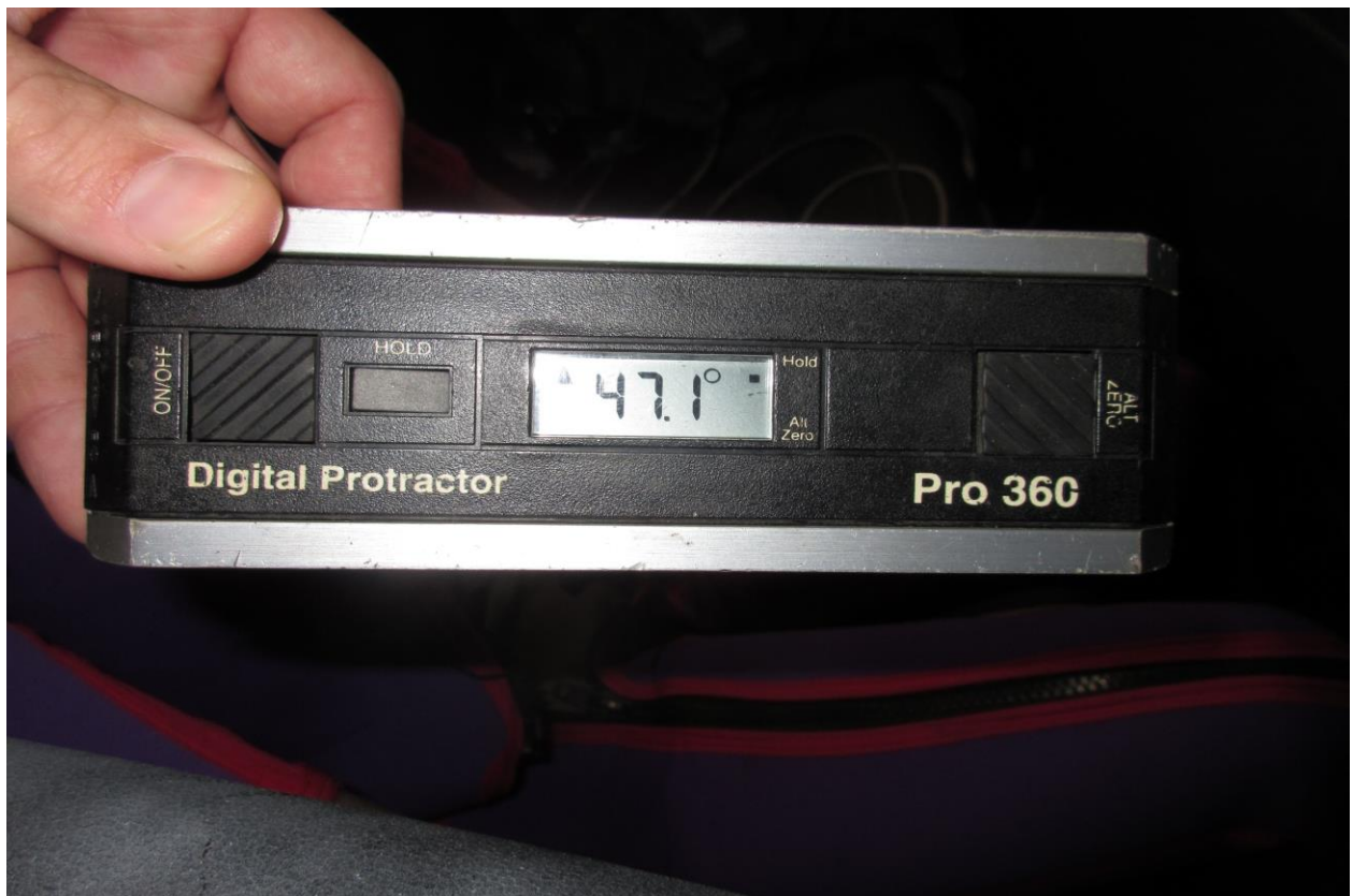
108 WorldSID-05F H-Point Inclinometer
