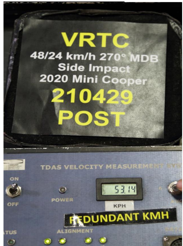
095 Post-Test Primary and Redundant Speed Trap Read-Out
