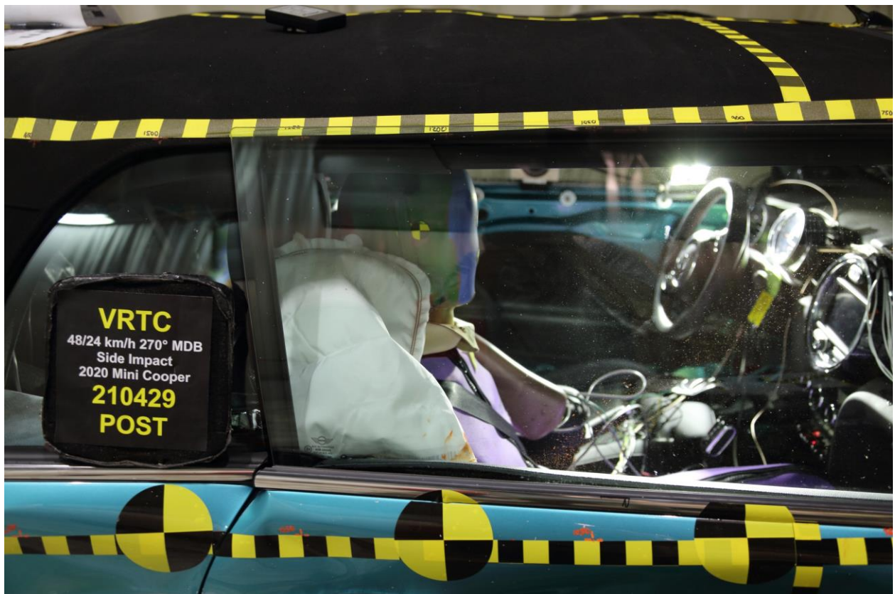
029 Post-Test Right Side View of Driver Dummy Shoulder and Door Top View
