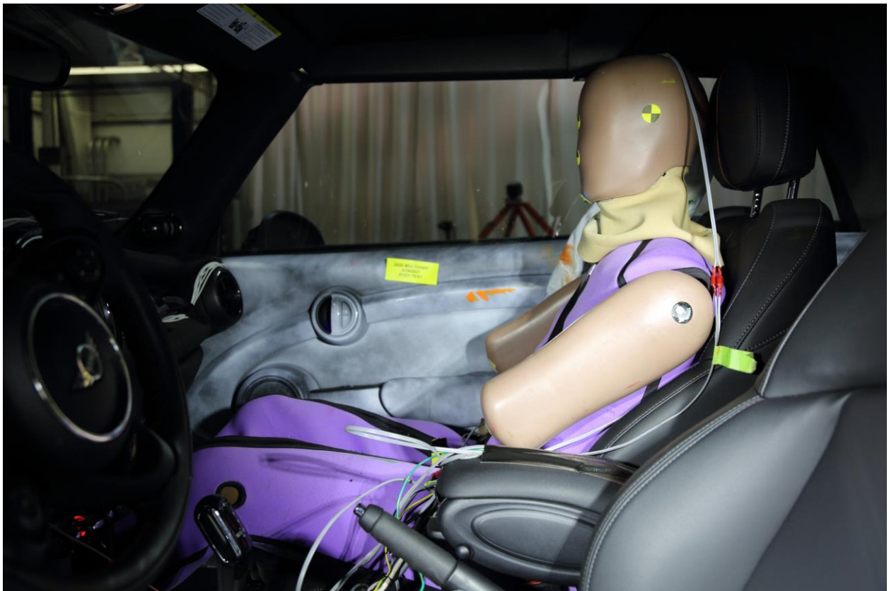
045 Post-Test Left Side View of Passenger Dummy and Front Seat of Occupant Compartment
