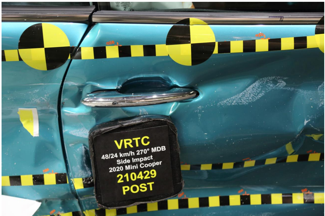
022 Post-Test Right Front Door Latch Close-Up
