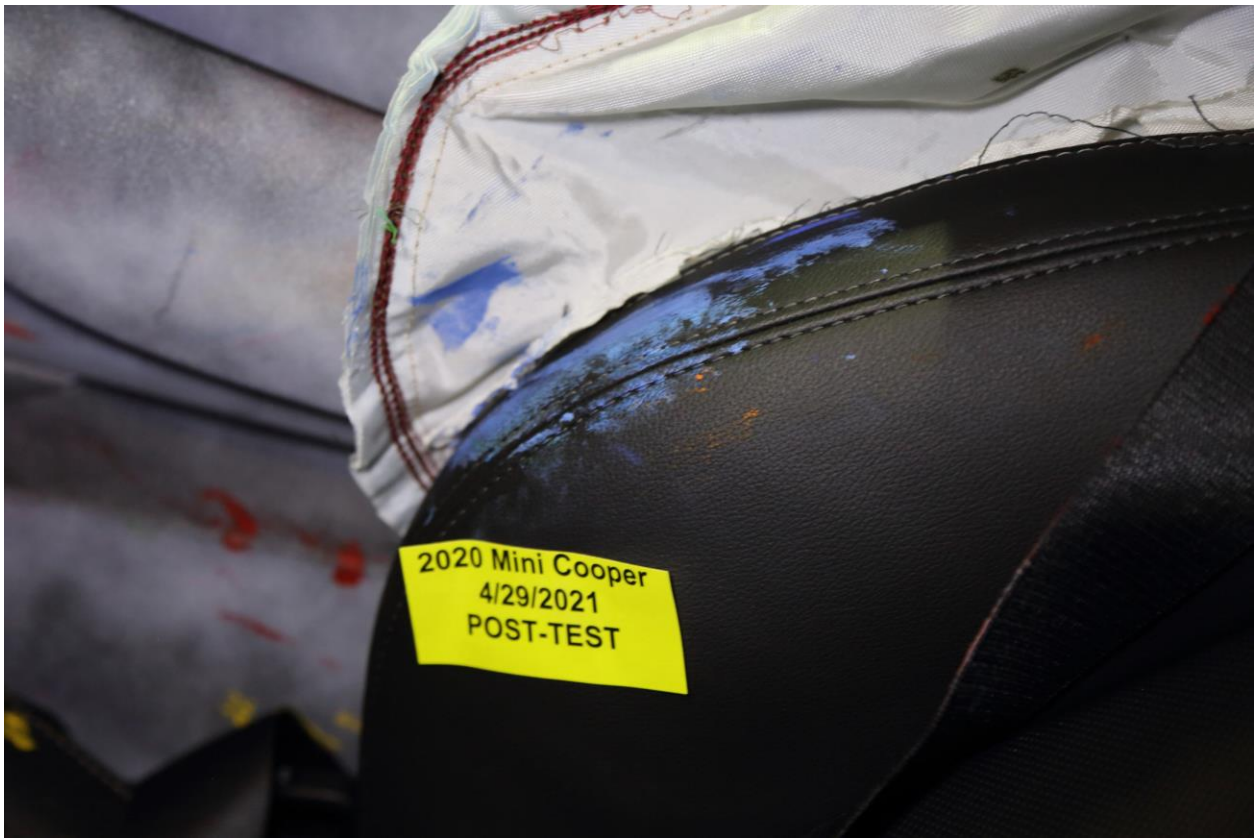
050 Post-Test Passenger Dummy Close-Up Torso Contact with Vehicle Interior View
