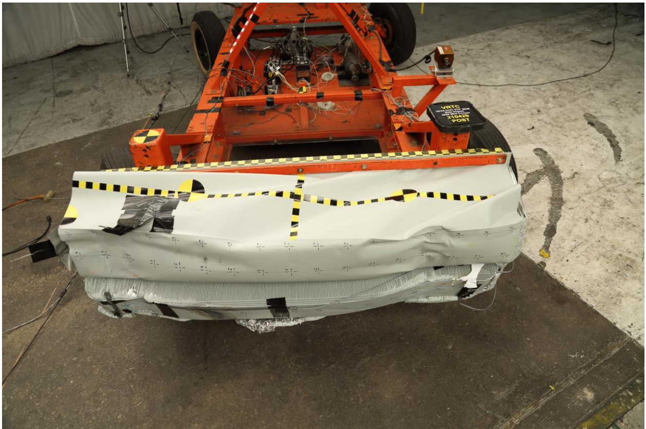
087 Post-Test Top View of MDB Impactor Face
