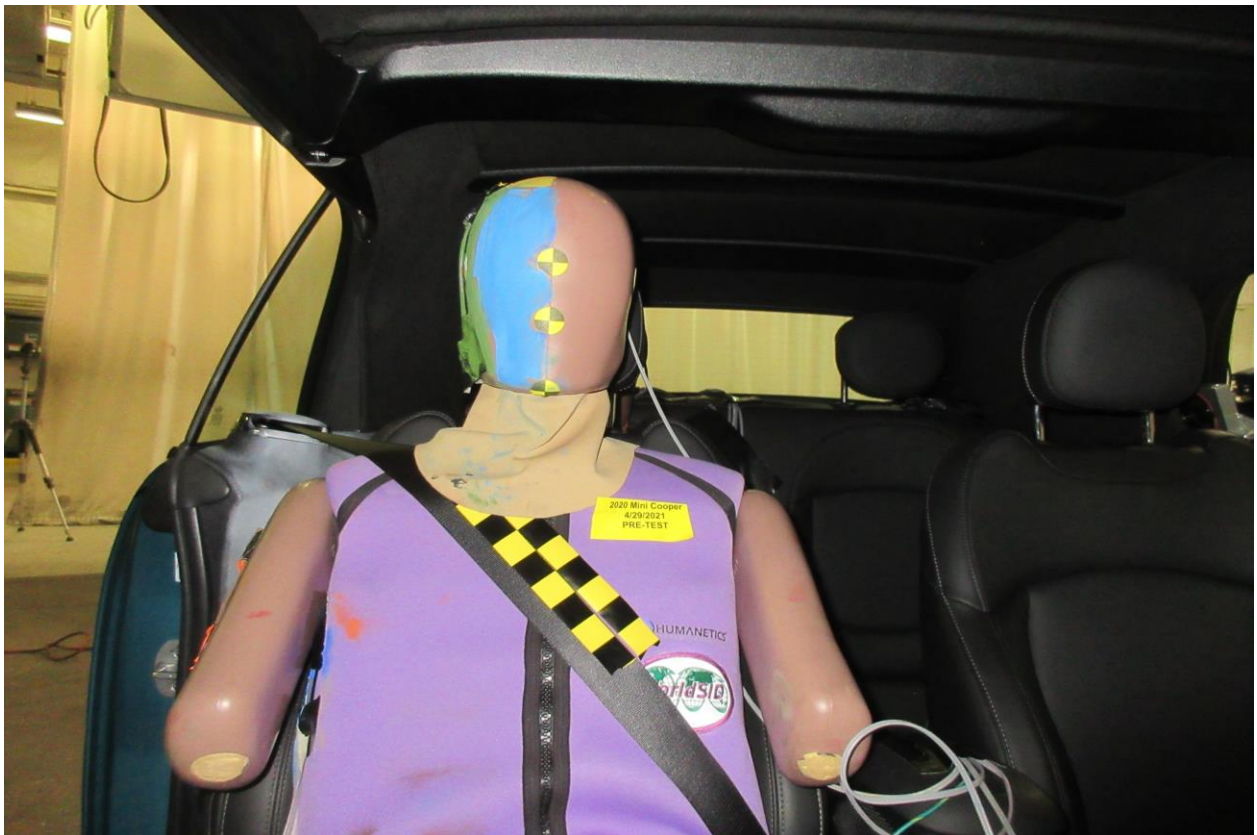
031 Pre-Test Frontal View of Passenger Dummy Head and Shoulders in Relation to Head Restraint
