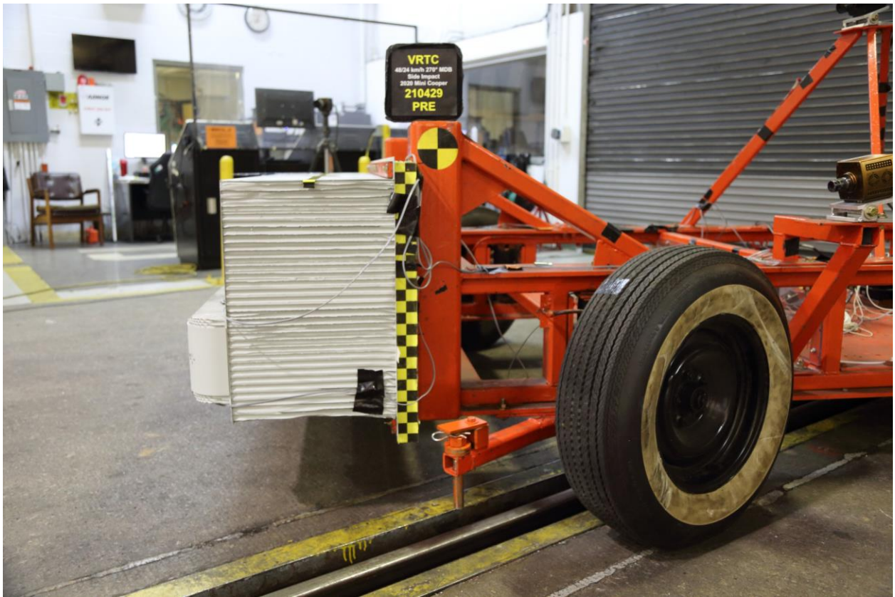
088 Pre-Test Left Side View of MDB Impactor Face
