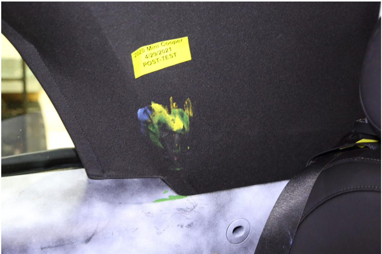
075 Post-Test Rear Passenger Dummy Close-Up Head Contact with Vehicle View
