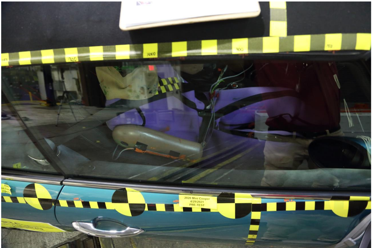
042 Pre-Test Passenger Dummy and Door Clearance View
