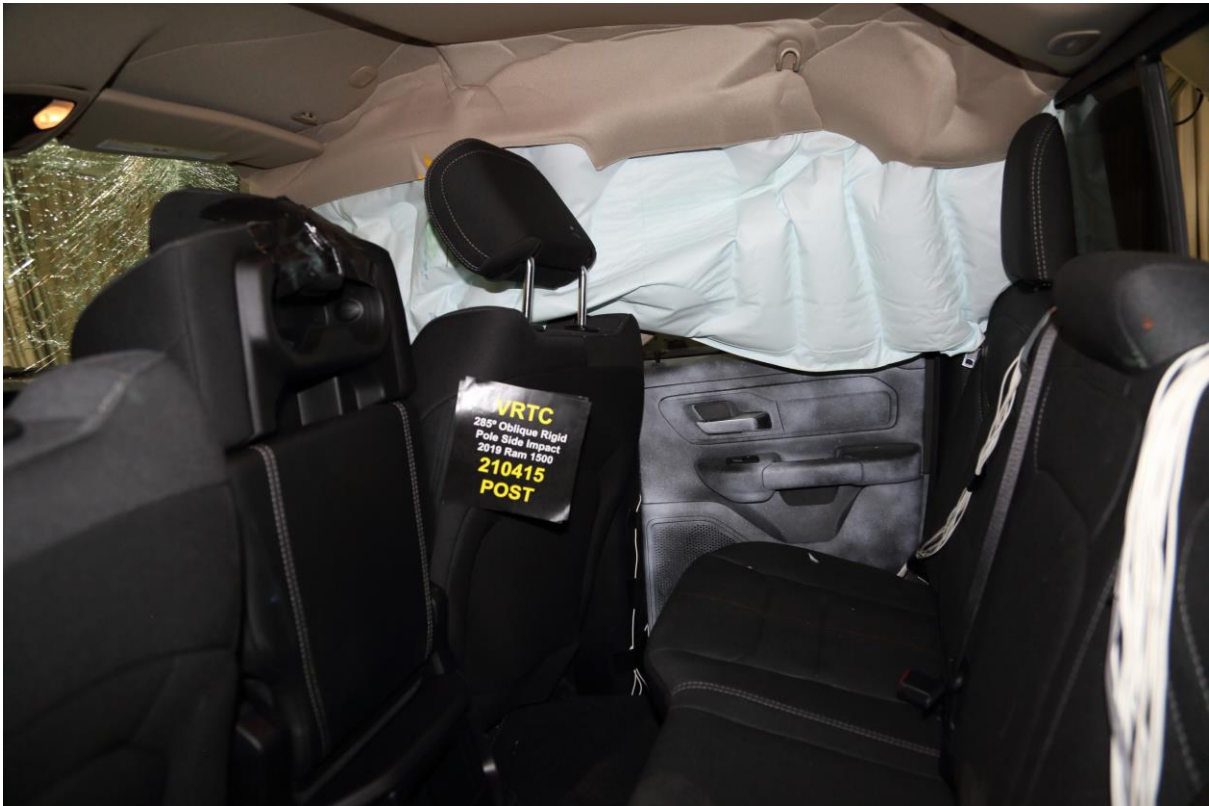
No. 053 Post-Test Left Side View of Dummy and Rear Seat of Occupant Compartment
