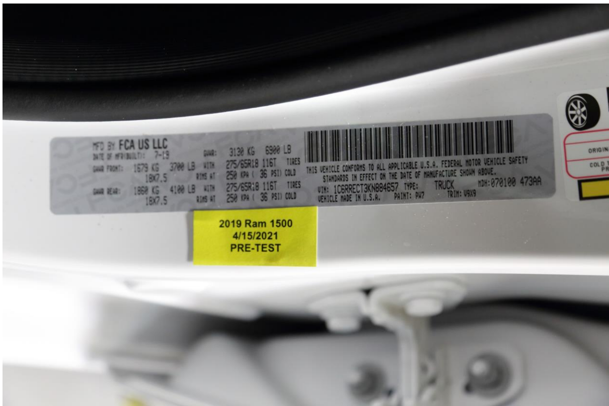
No. 056 Close-Up View of Vehicle Certification Label
