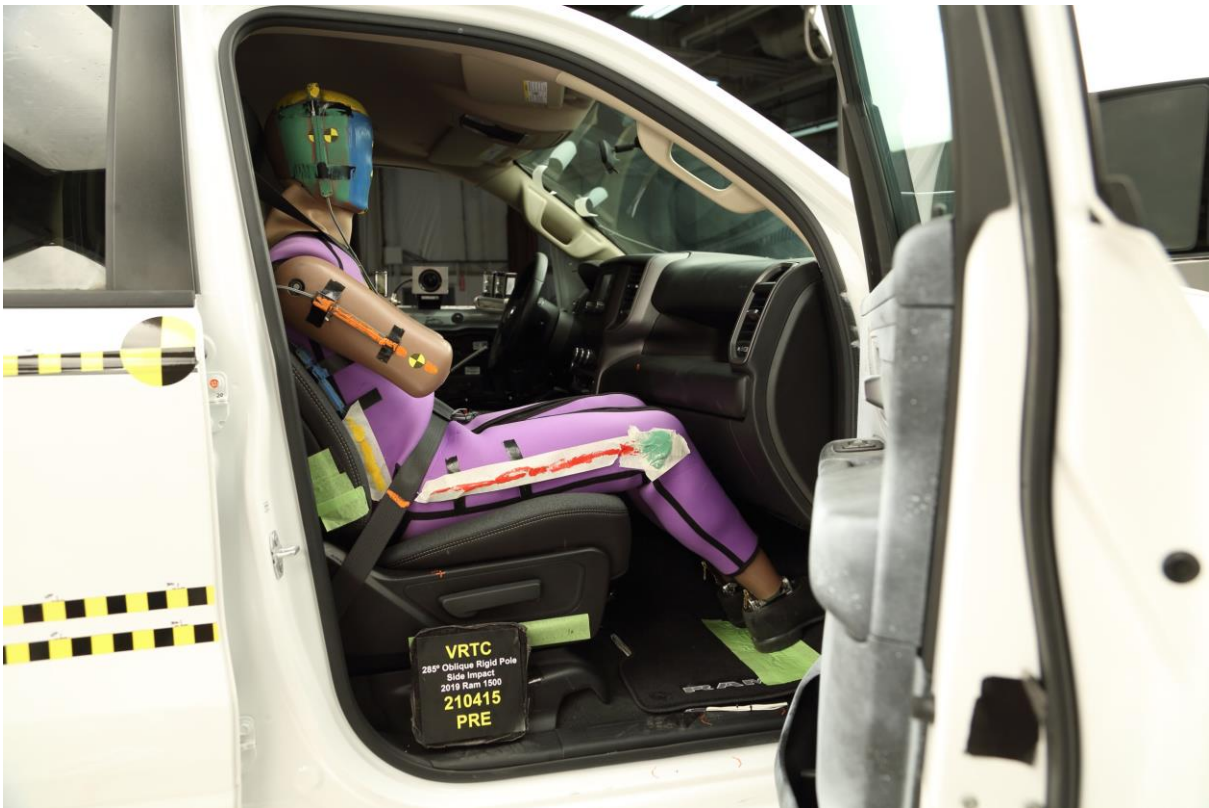
No. 023 Pre-Test Right Side View of Dummy Showing Belt and Chalking
