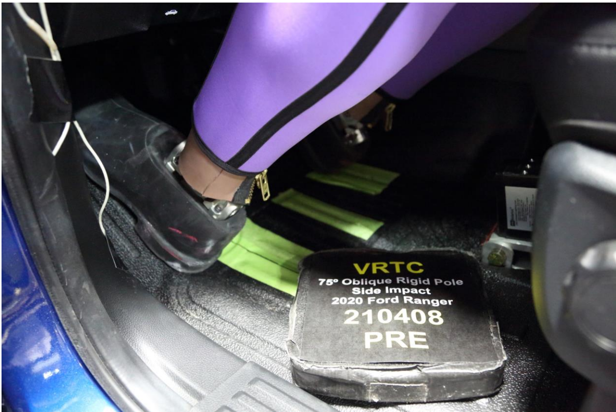
No. 032 Pre-Test Placement of Dummy Feet
