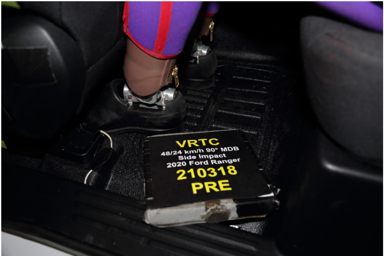
064 Pre-Test Placement of Rear Passenger Dummy's Feet
