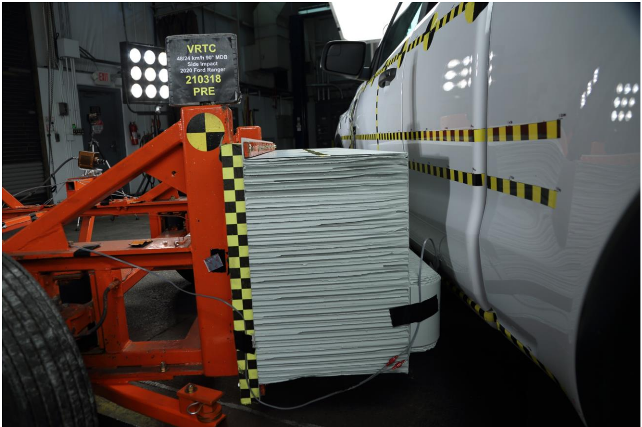
018 Pre-Test Right Side View MDB Positioned Against Side of Test Vehicle
