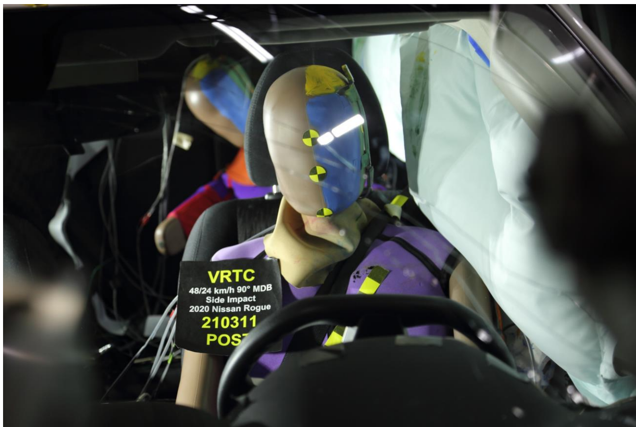
026 Post-Test Front Close-Up View of Driver Dummy
