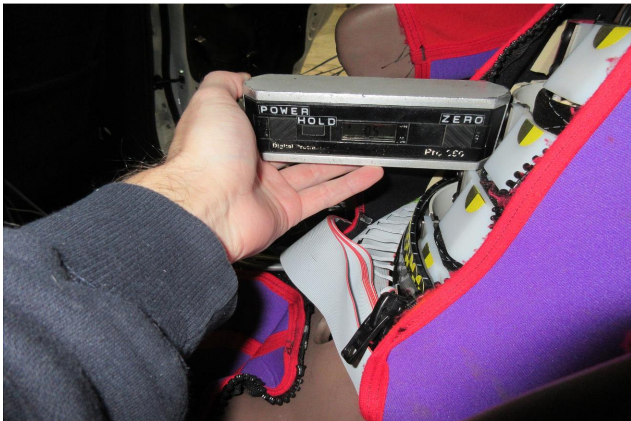
No. 107 WorldSID-05F Thorax Rib 2 Inclinometer
