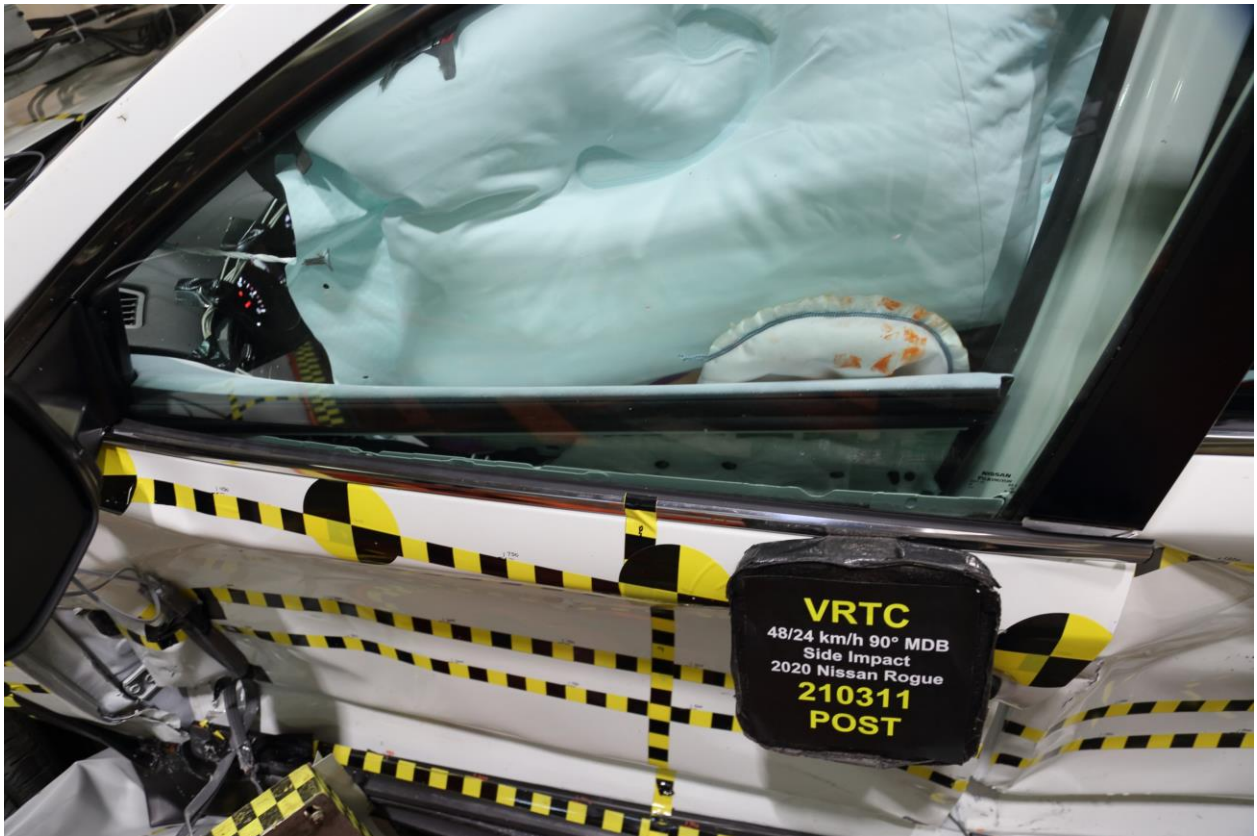
043 Post-Test Driver Dummy and Door Clearance View
