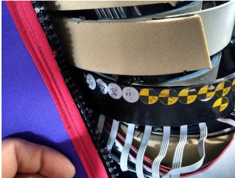
Figure 3. Right side of WorldSID 5th dummy showing chest band location
