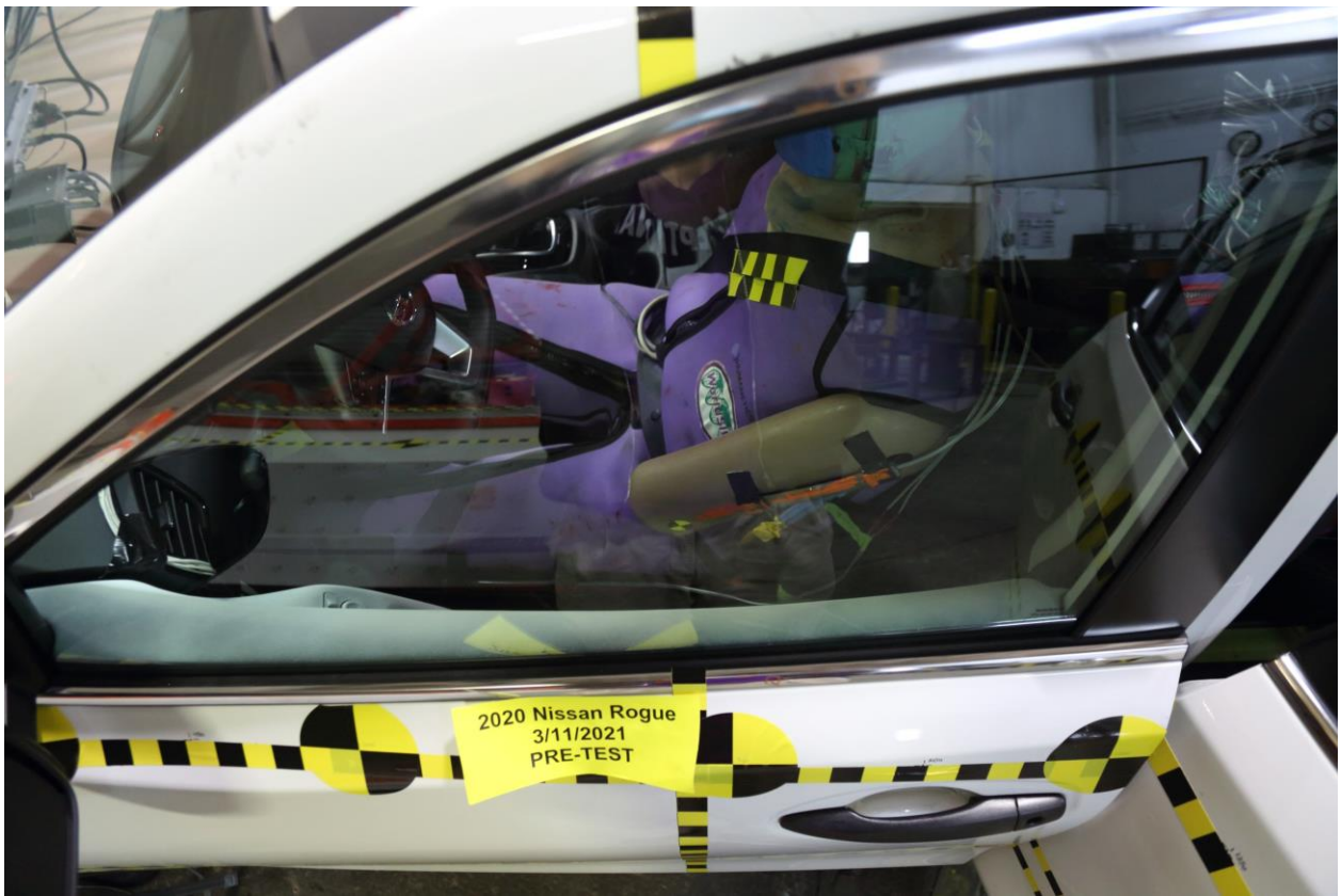
042 Pre-Test Driver Dummy and Door Clearance View
