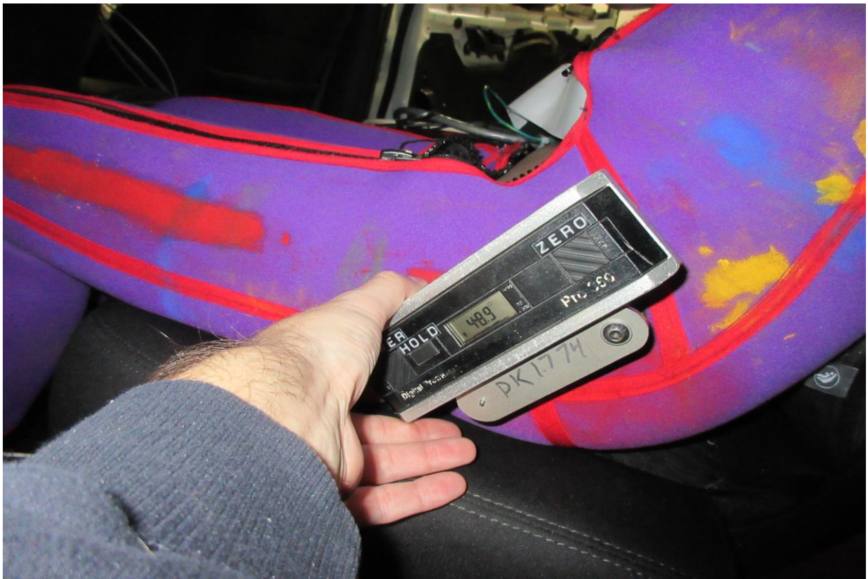
No. 108 WorldSID-05F H-Point Inclinometer
