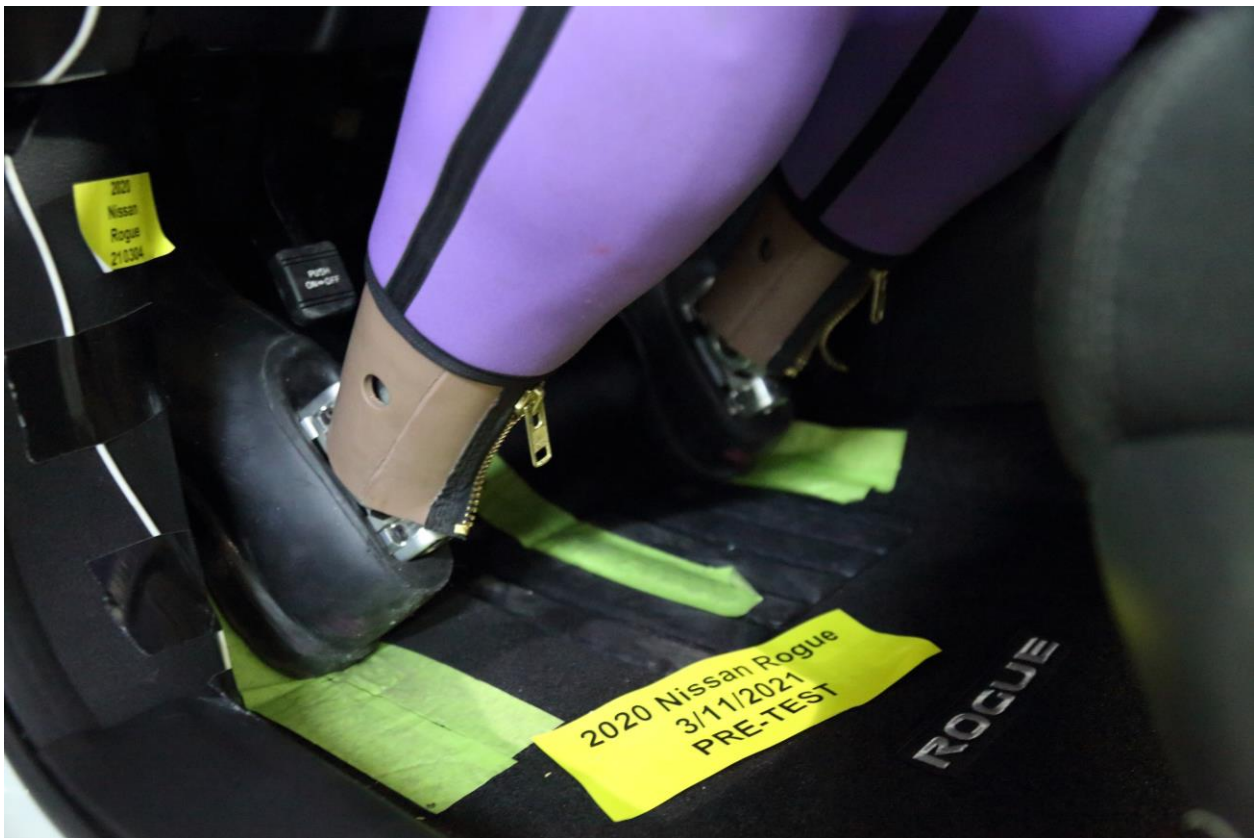
034 Pre-Test Placement of Driver's Dummy Feet
