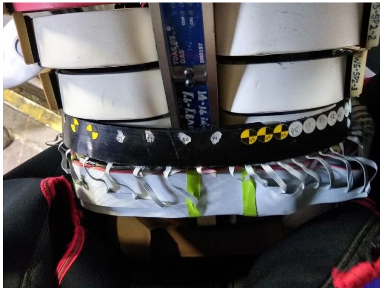
Figure 1. Rear of WorldSID 5th dummy showing chest band location
