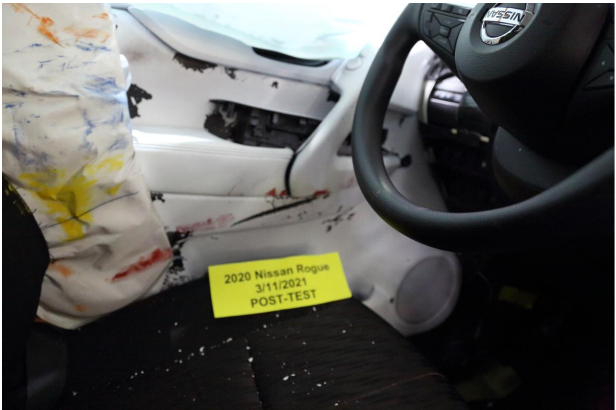
052 Post-Test Driver Dummy Close-Up Pelvis Contact View
