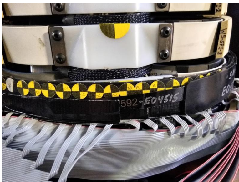
Figure 2. Front of WorldSID 5th dummy showing chest band location
