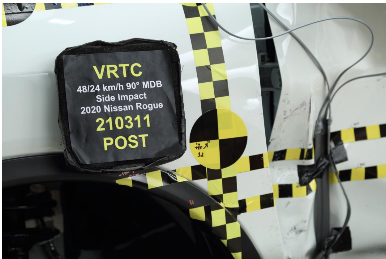
020 Post-Test Close-Up View of Impact Point Target
