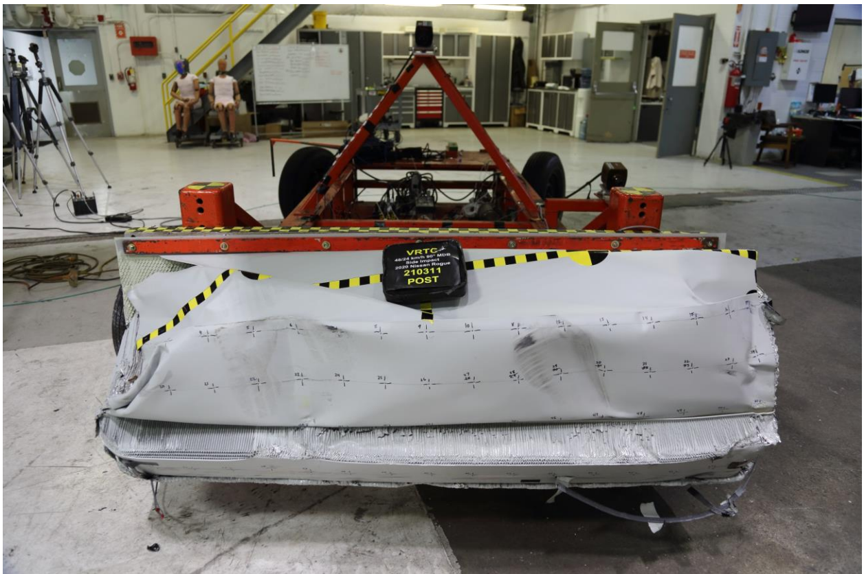
085 Post-Test Front View of MDB Impactor Face
