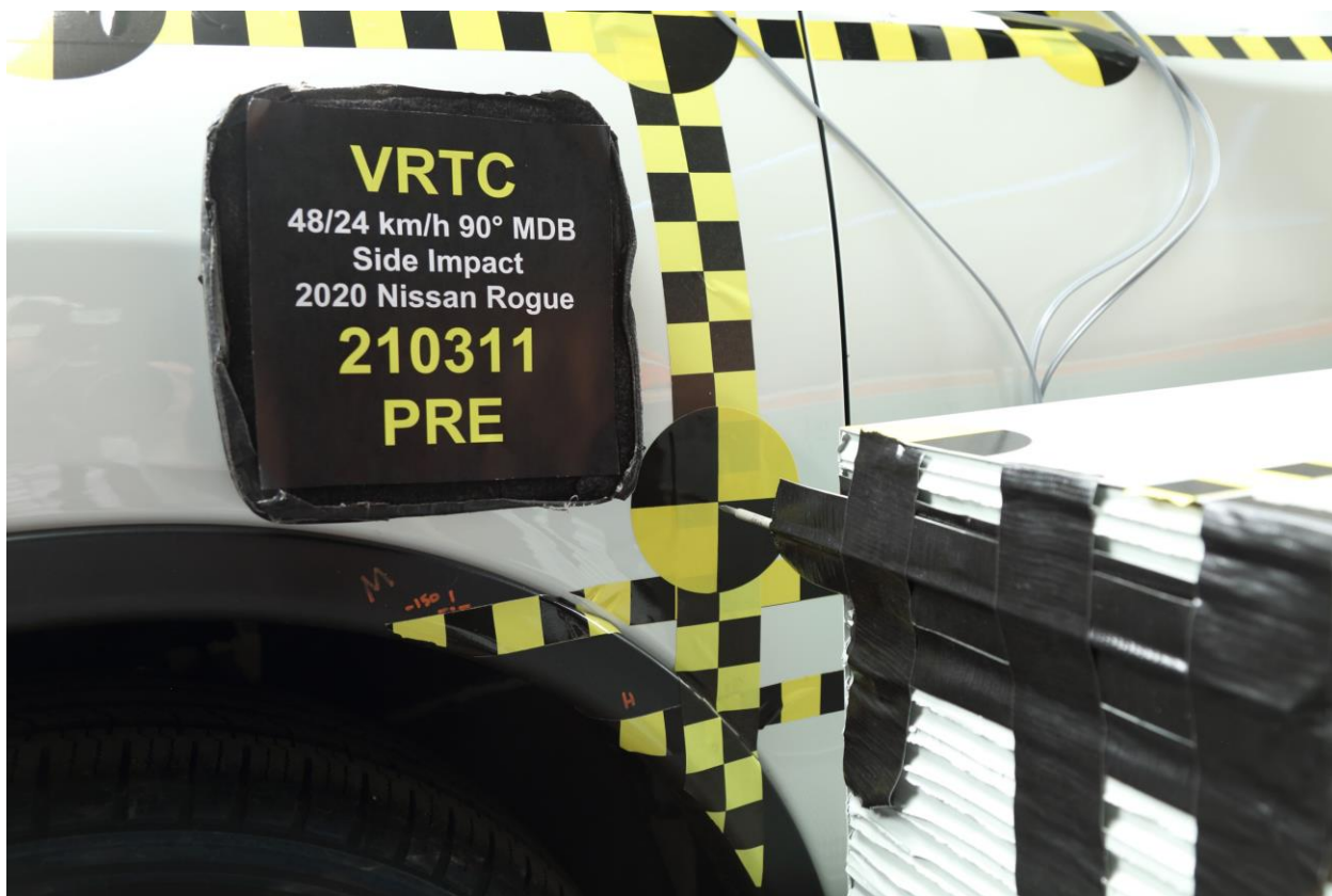
019 Pre-Test Close-Up View of Impact Point Target
