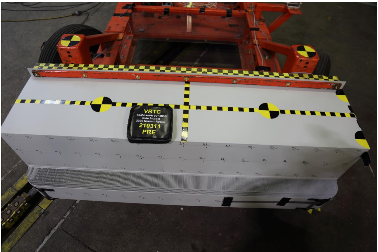
086 Pre-Test Top View of MDB Impactor Face
