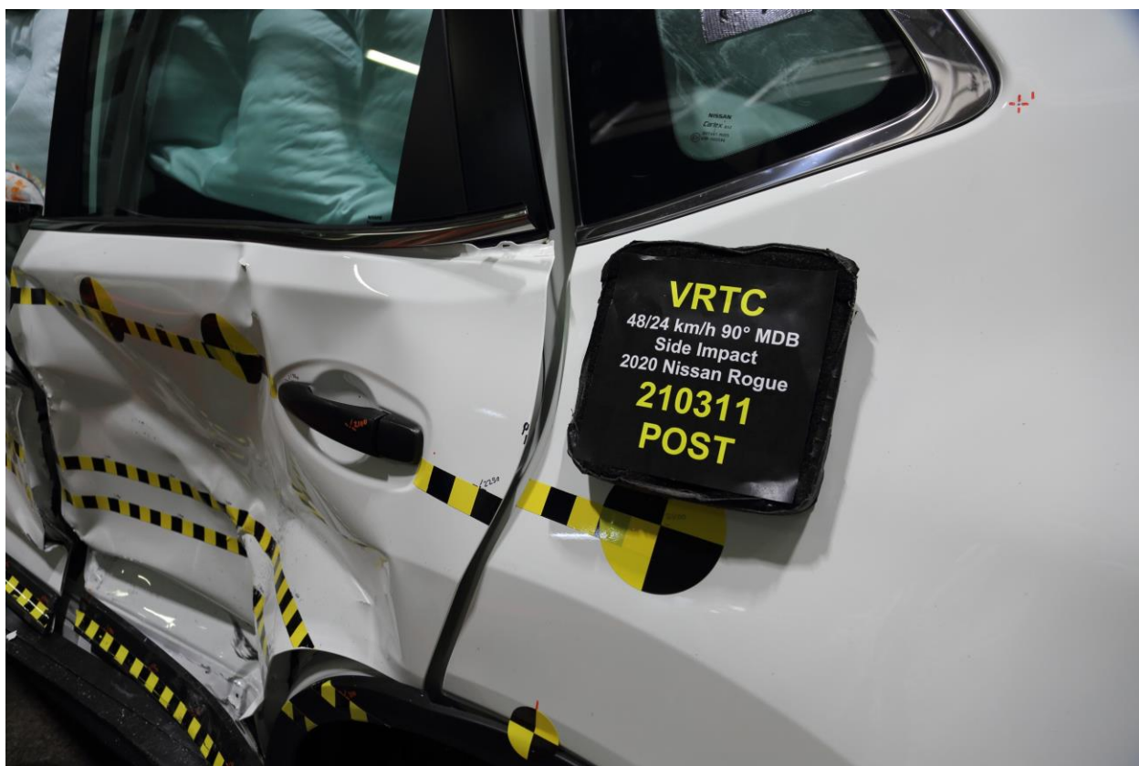
024 Post-Test Left Rear Door Latch Close-Up
