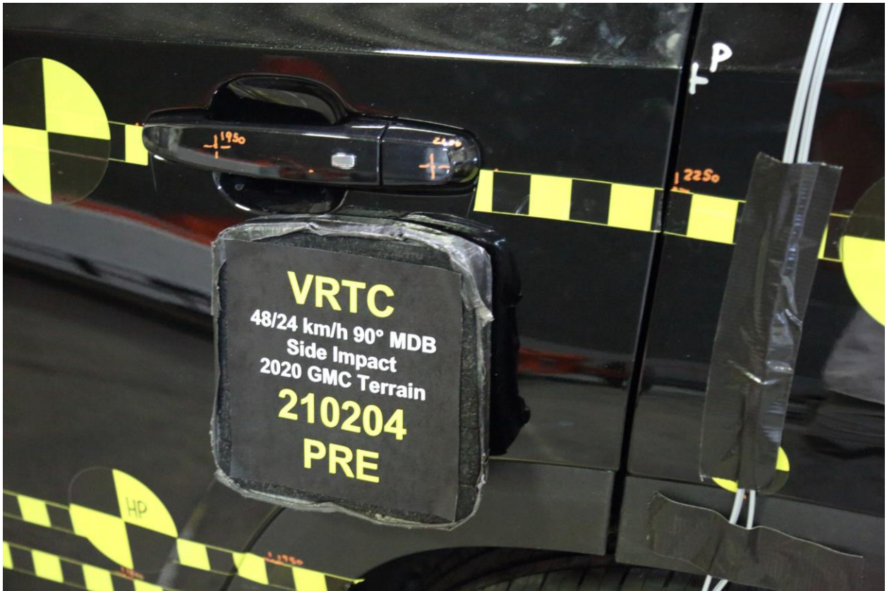
023 Pre-Test Left Rear Door Latch Close-Up
