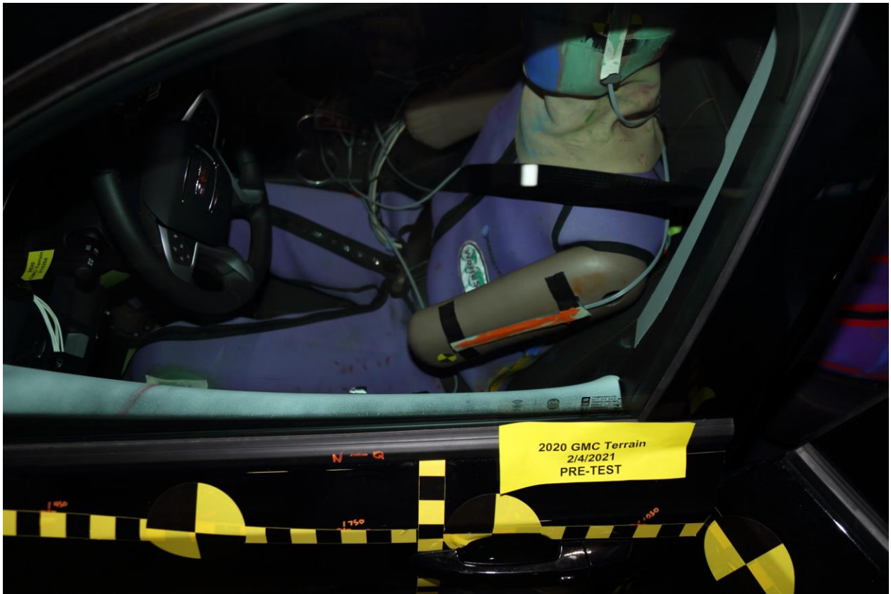
042 Pre-Test Driver Dummy and Door Clearance View
