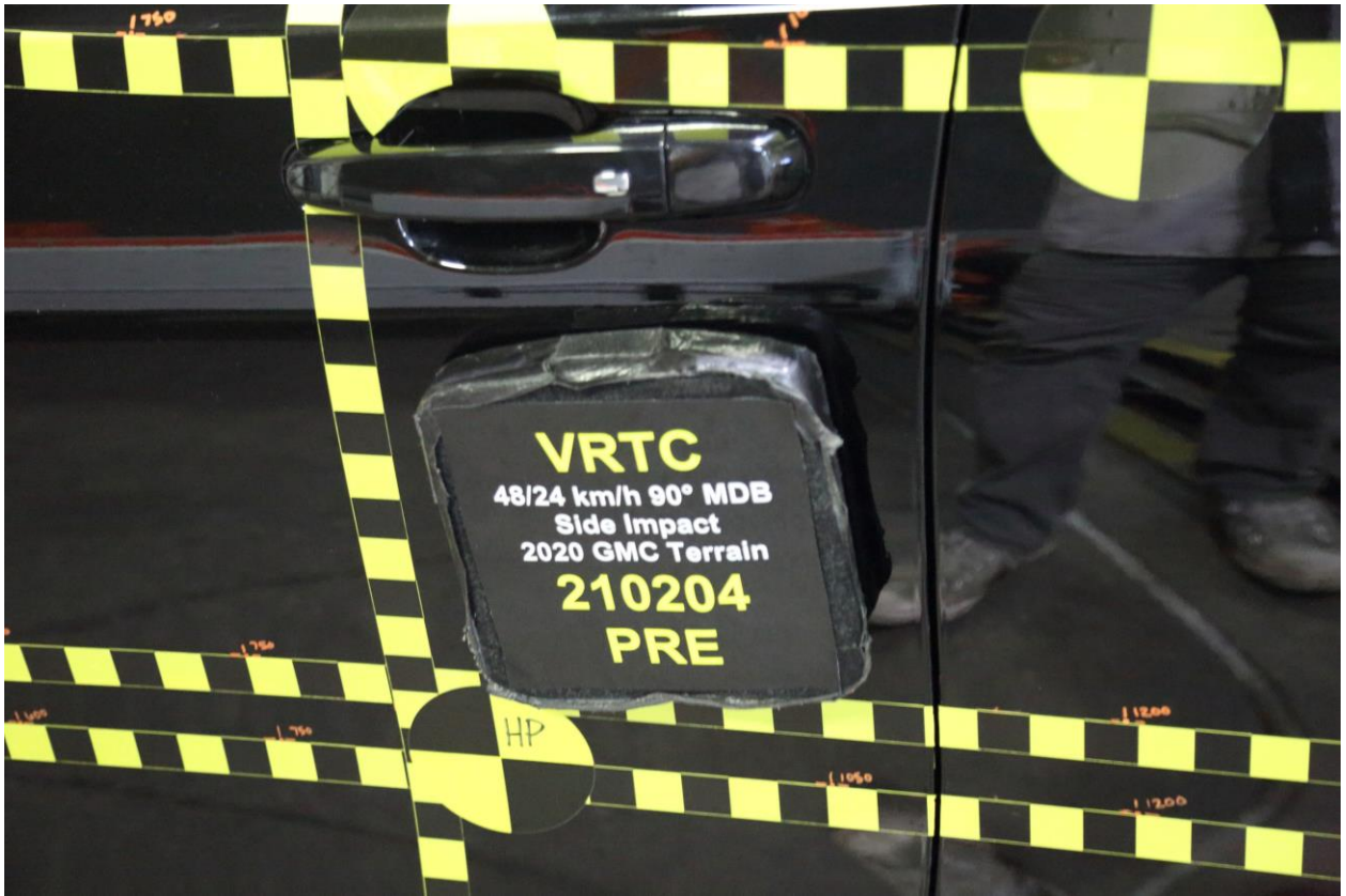
021 Pre-Test Left Front Door Latch Close-Up
