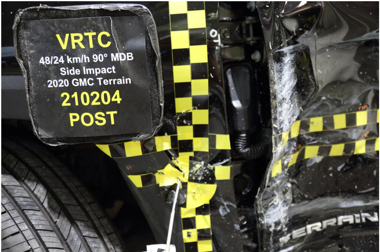
020 Post-Test Close-Up View of Impact Point Target
