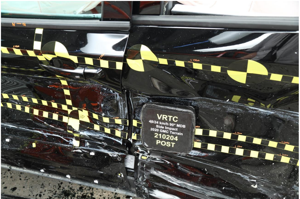
022 Post-Test Left Front Door Latch Close-Up
