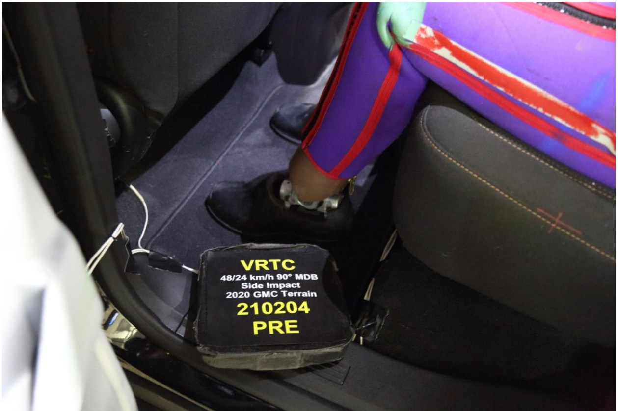
064 Pre-Test Placement of Rear Passenger Dummy's Feet
