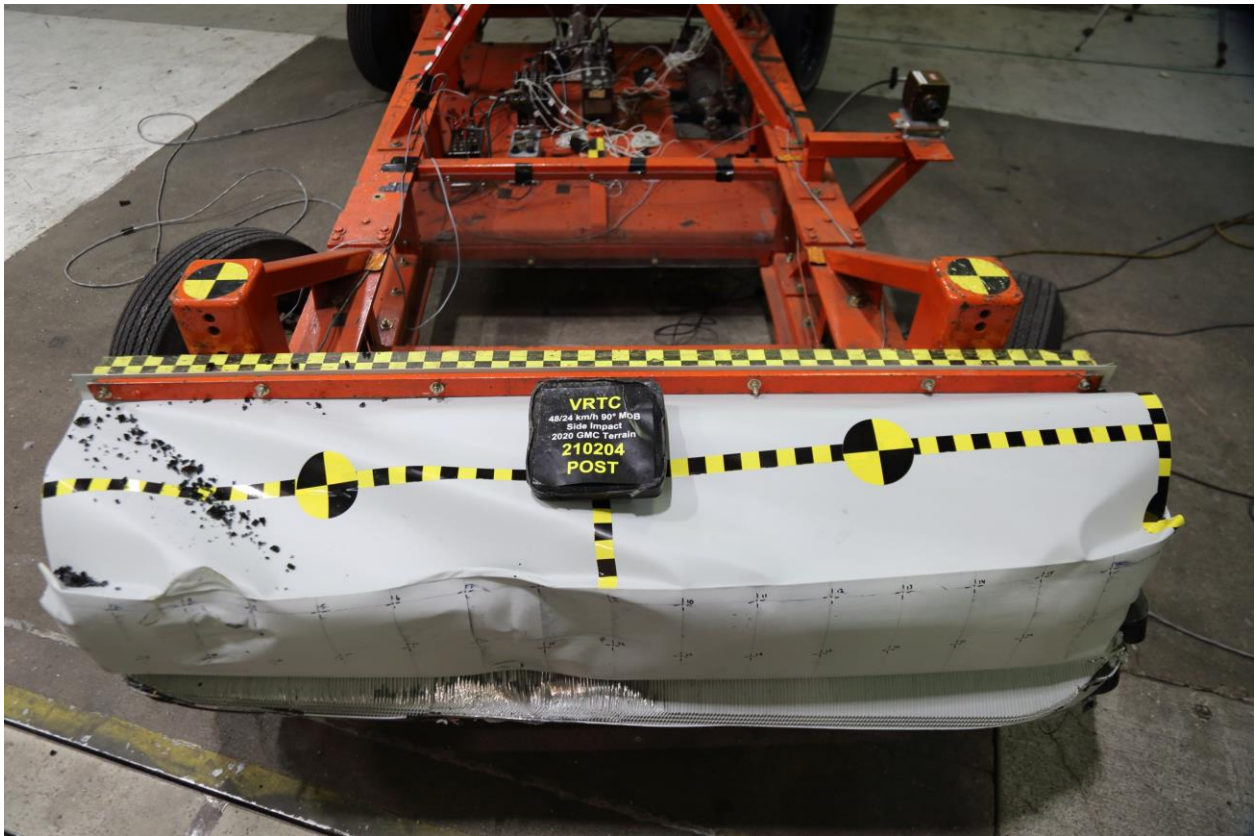
087 Post-Test Top View of MDB Impactor Face
