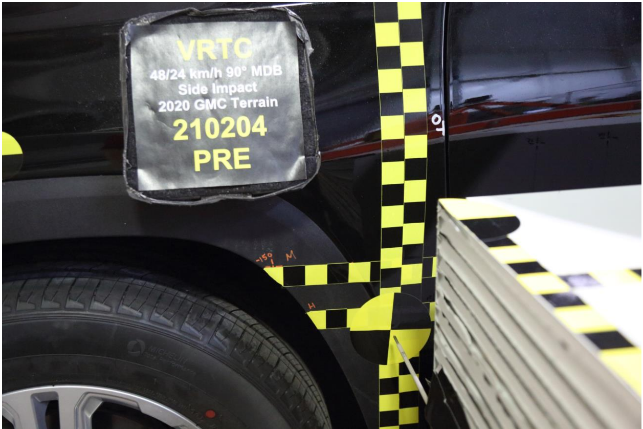
019 Pre-Test Close-Up View of Impact Point Target
