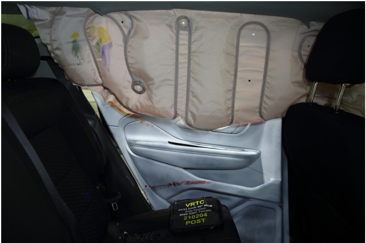
074 Post-Test Rear Passenger Inner Door Panel View
