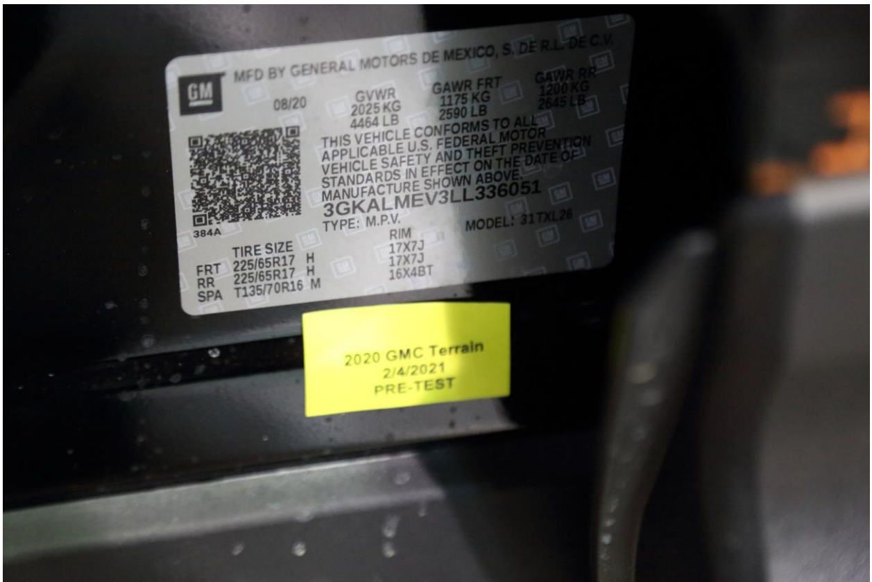
092 Close-Up View of Vehicle's Certification Label
