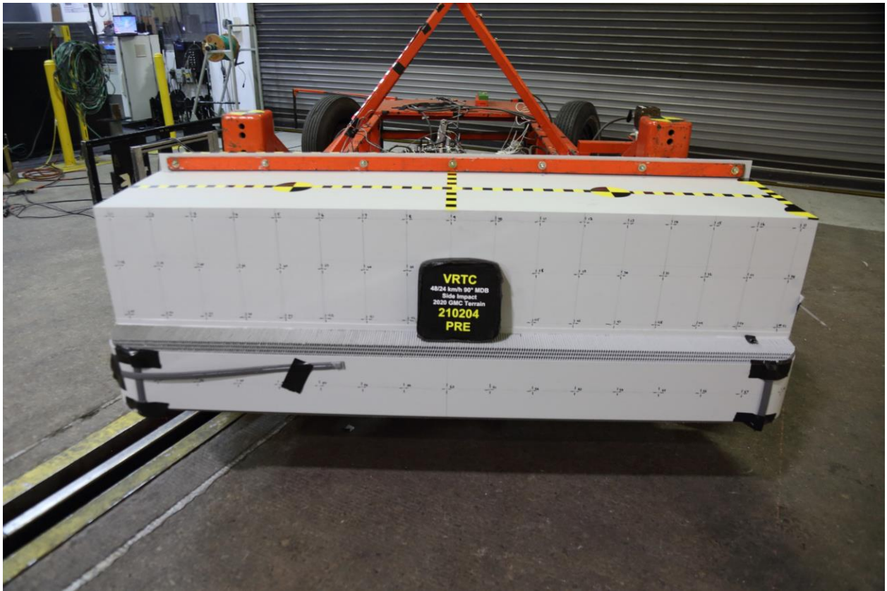
084 Pre-Test Front View of MDB Impactor Face
