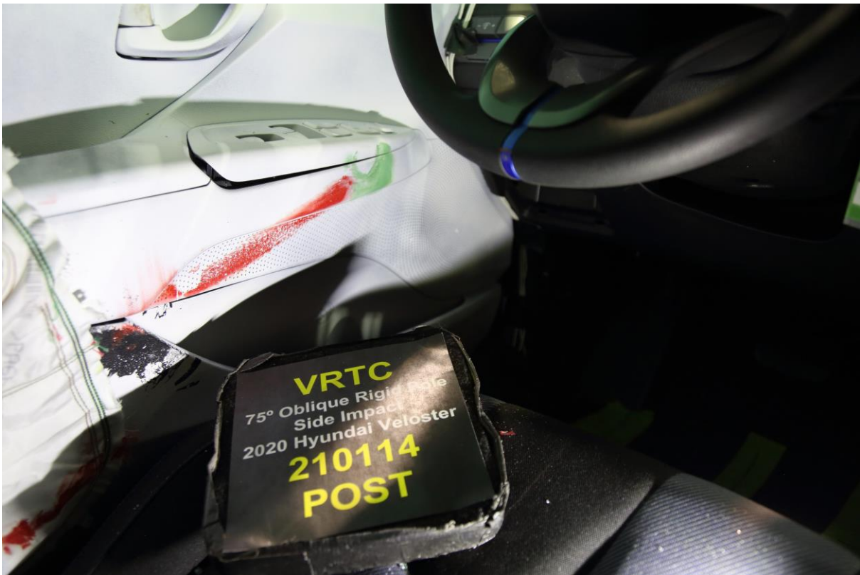
No. 050 Post-Test Dummy Close-Up Pelvis Contact with Vehicle Interior View
