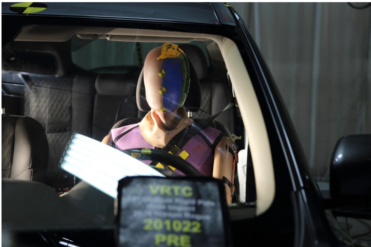
No. 027 Pre-Test Front Close-Up View of Dummy Head and Shoulders in Relation to Head Restraint
