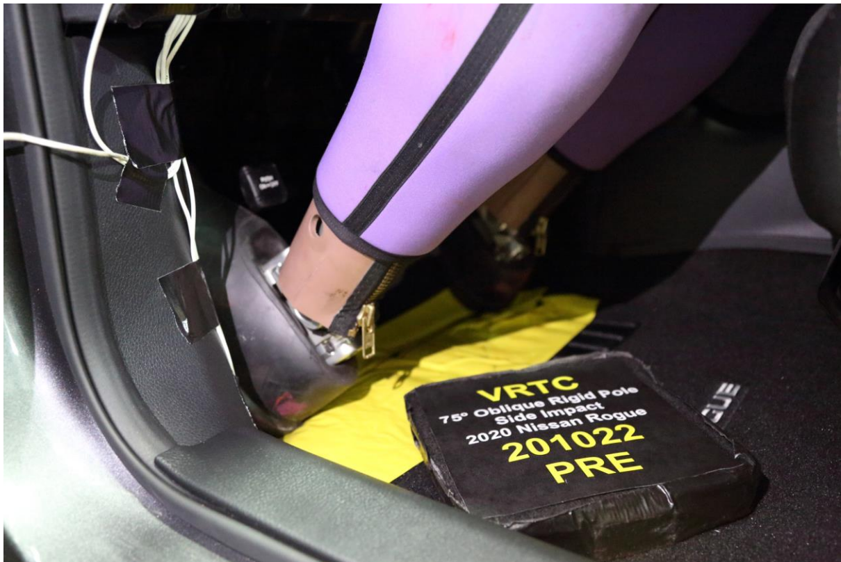
No. 032 Pre-Test Placement of Dummy Feet
