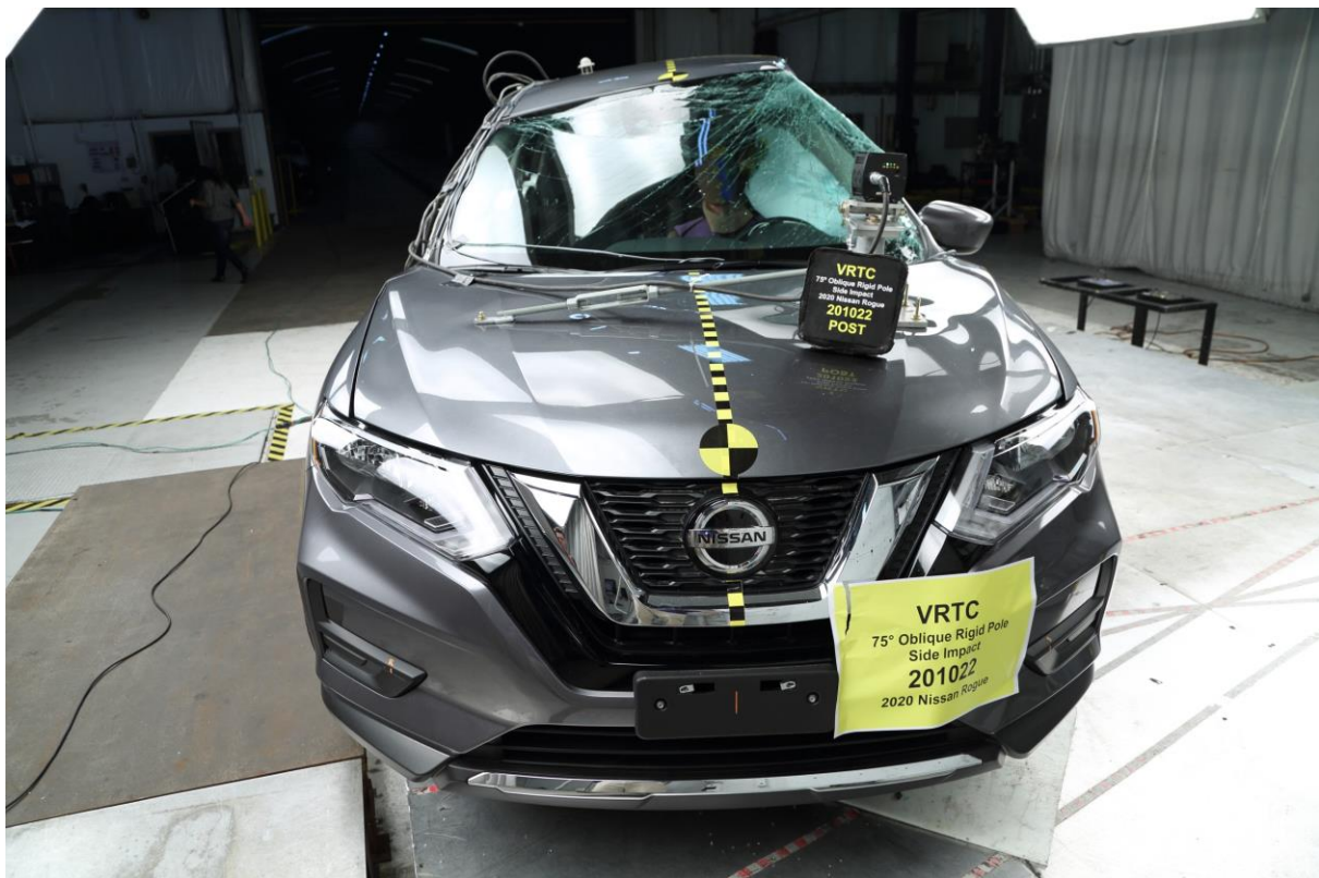
No. 004 Post-Test Frontal View of Test Vehicle
