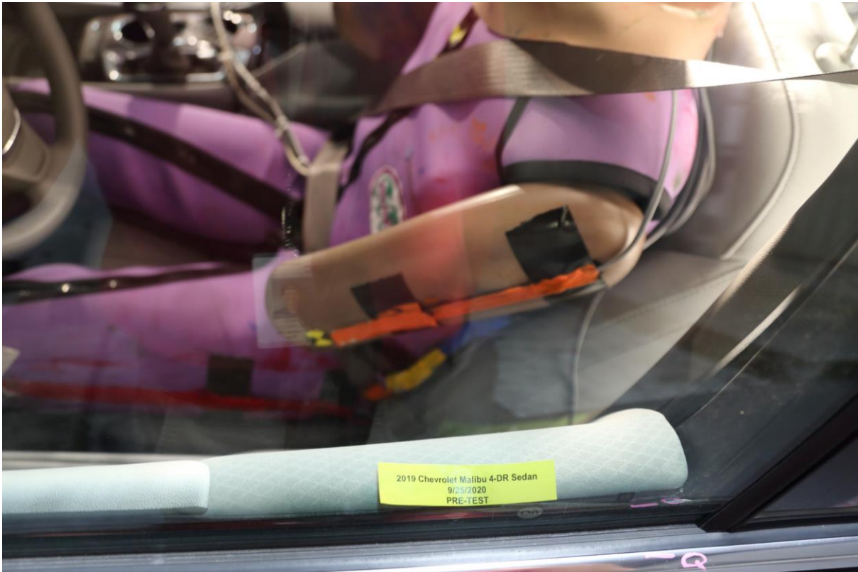
No. 040 Pre-Test Dummy and Door Clearance View
