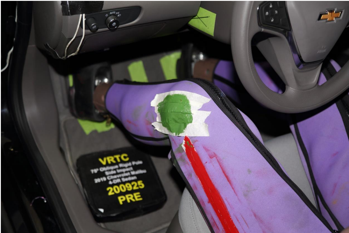
No. 032 Pre-Test Placement of Dummy Feet
