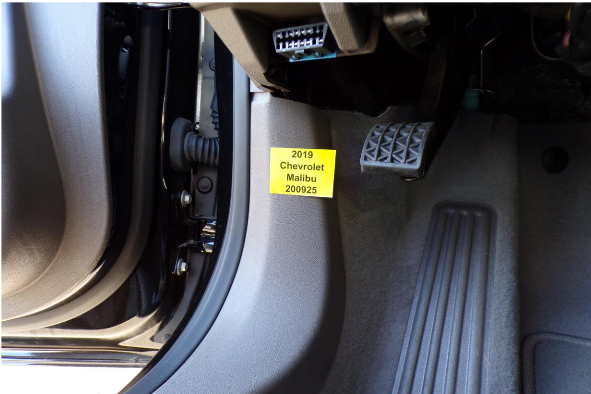
No. 035 Pre-Test View of Disengaged Parking Brake
