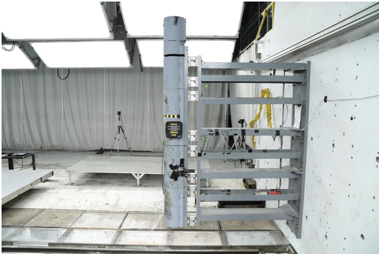
No. 060 Pre-Test Pole Barrier Side View
