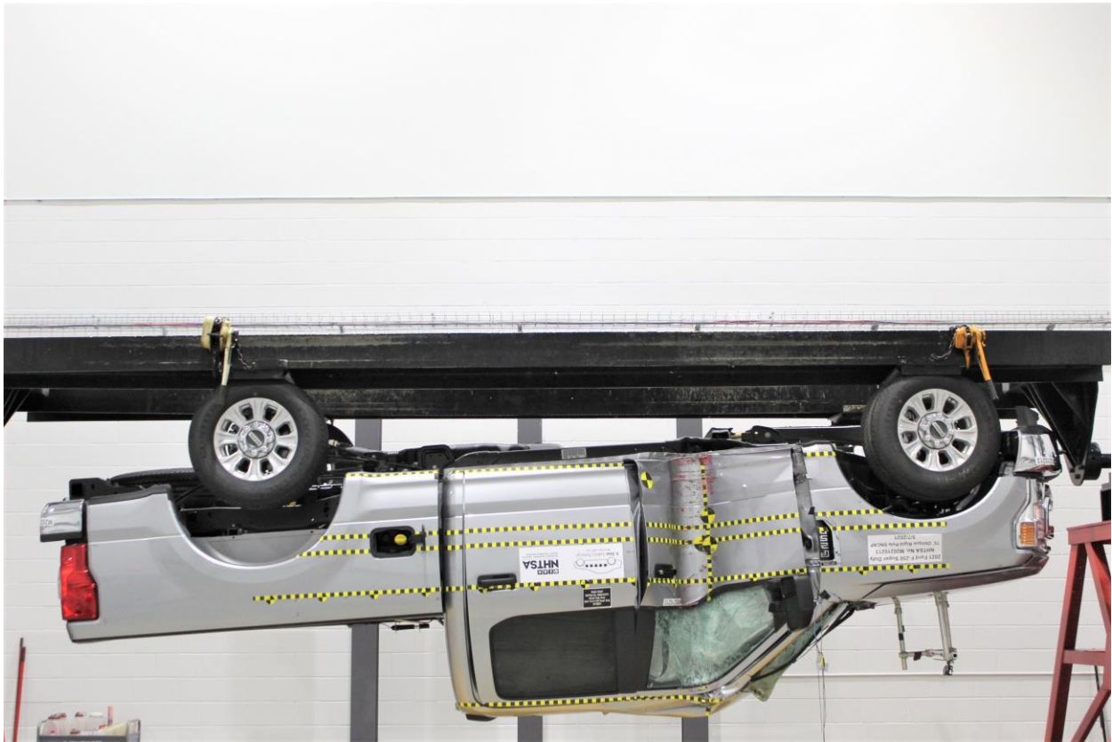
Figure A-67: FMVSS No. 301 Static Rollover 180 Degrees
