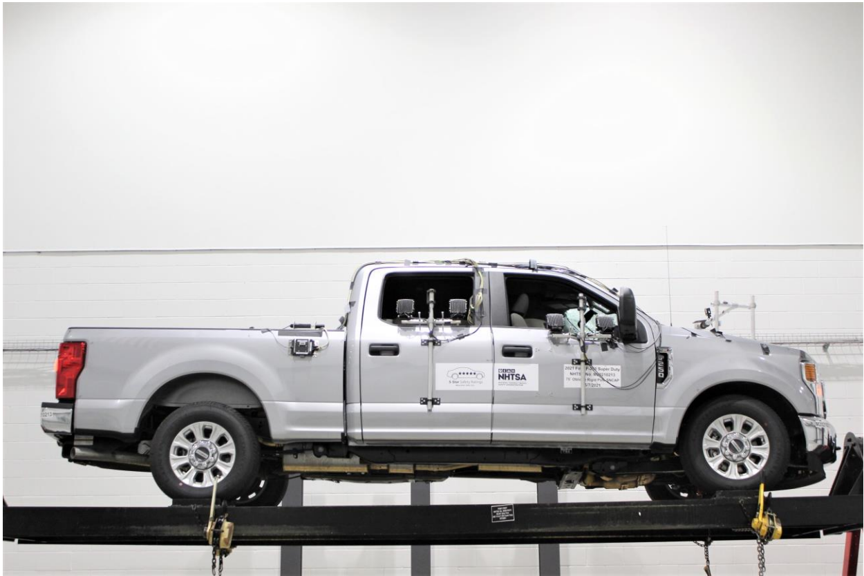
Figure A-69: FMVSS No. 301 Static Rollover 360 Degrees
