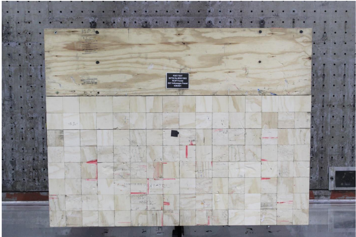
Figure A-3: Post-Test Load Cell Wall
