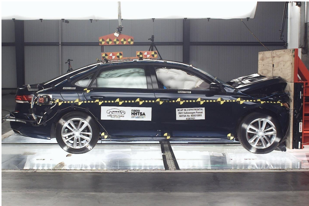
Figure A-82: 2021 Volkswagen Passat Frontal Impact Event
