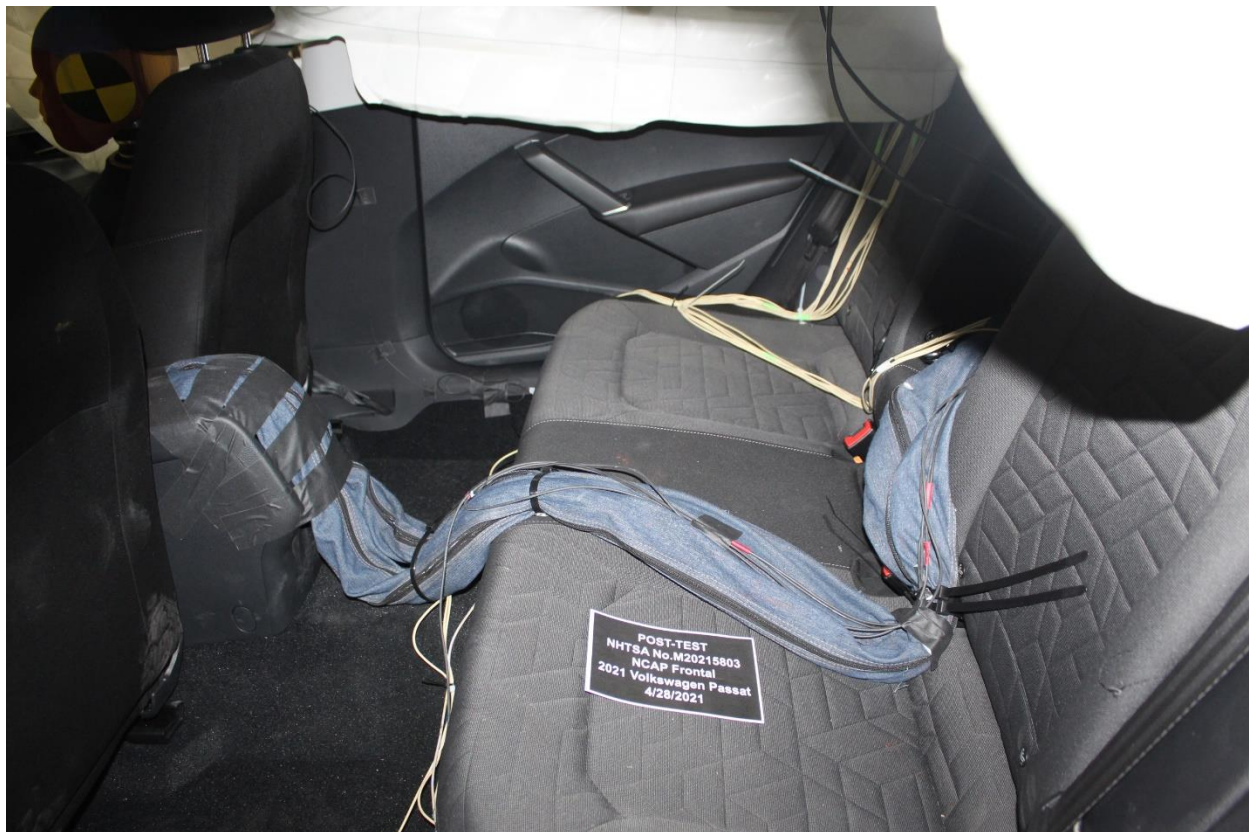
Figure A-29: Post-Test Dummy Cable Routing
