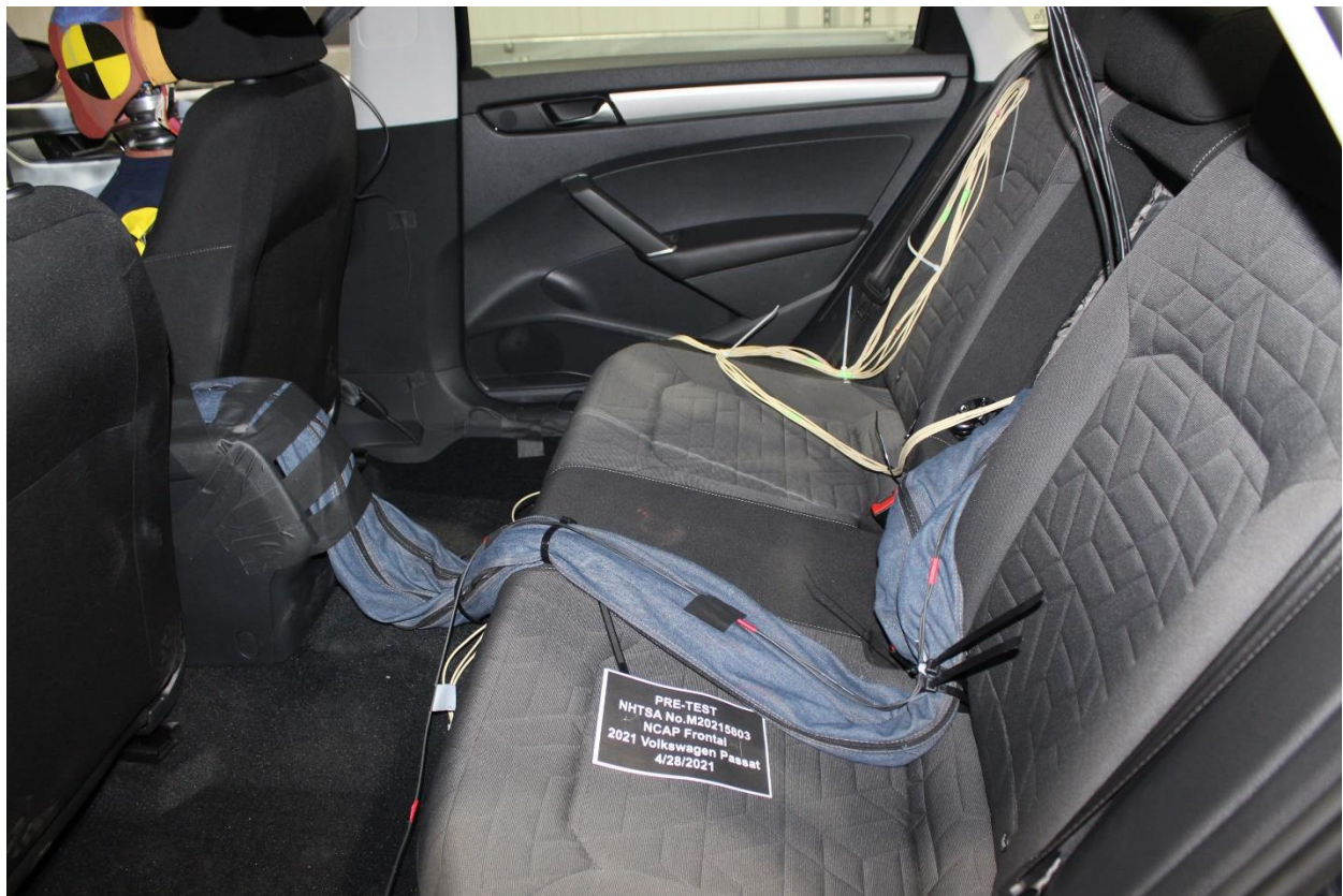
Figure A-28: Pre-Test Dummy Cable Routing
