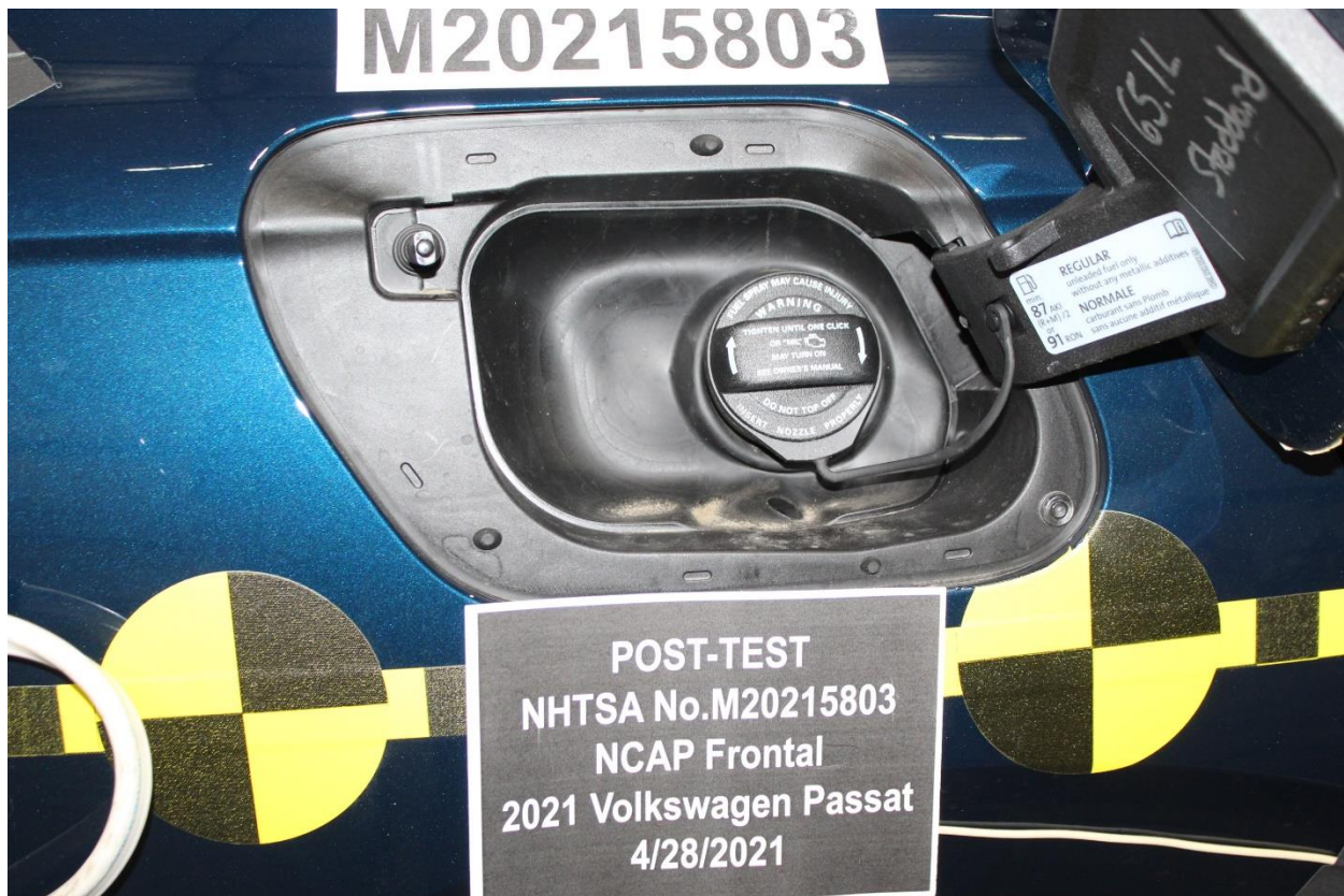
Figure A-23: Post-Test Fuel Filler Cap View
