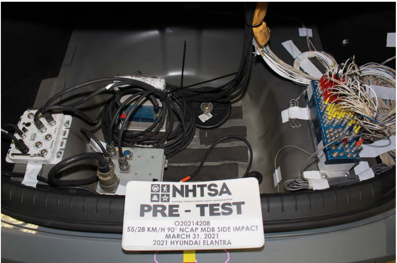
Photo No. 094 - Pre-Test Ballast View
