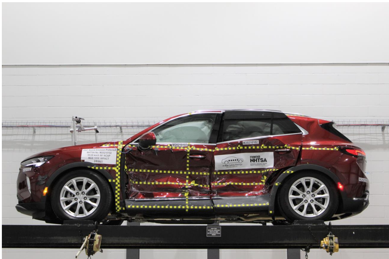
Figure A-96: FMVSS No. 301 Static Rollover 0 Degrees
