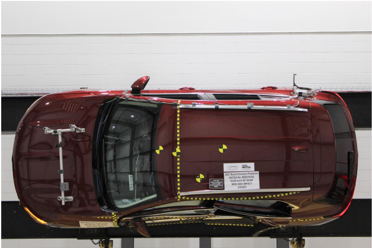
Figure A-99: FMVSS No. 301 Static Rollover 270 Degrees
