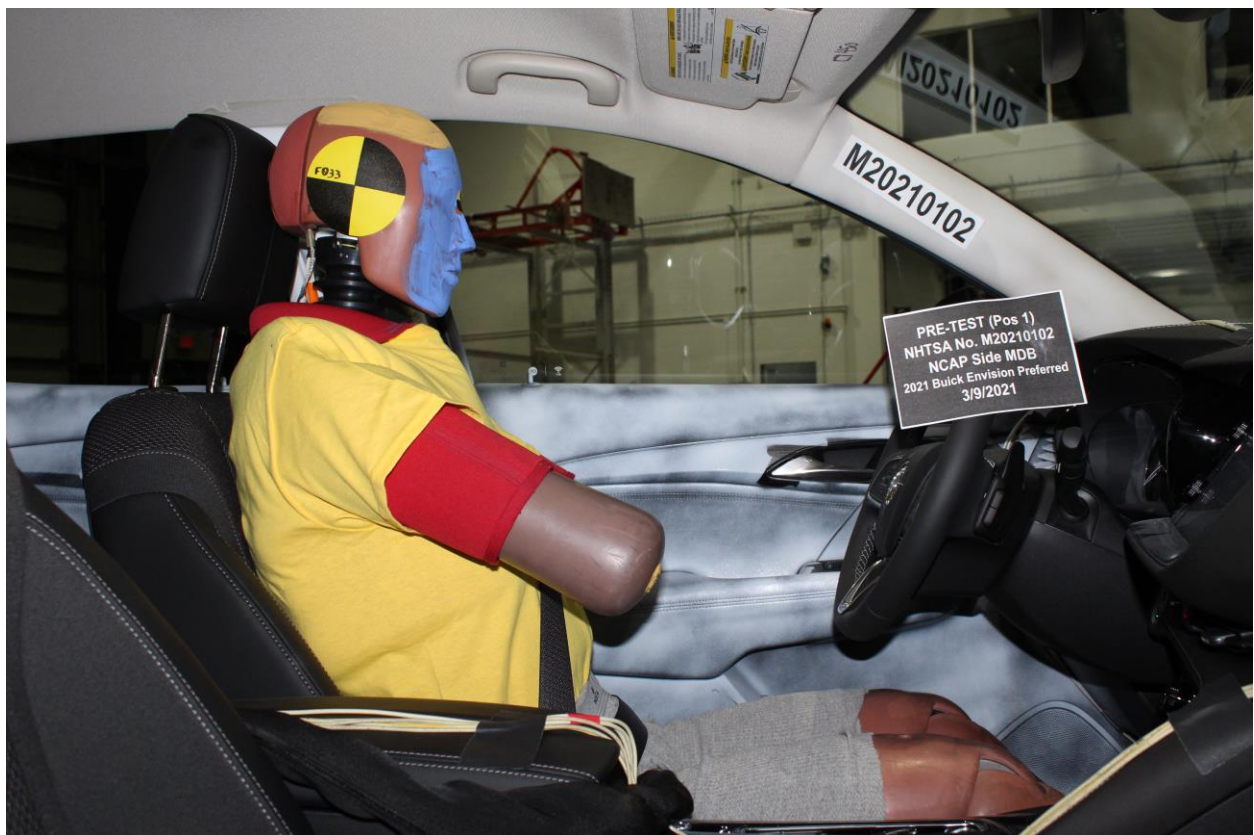
Figure A-44: Pre-Test Right Side View of Driver Dummy and Front Seat of Occupant Compartment
