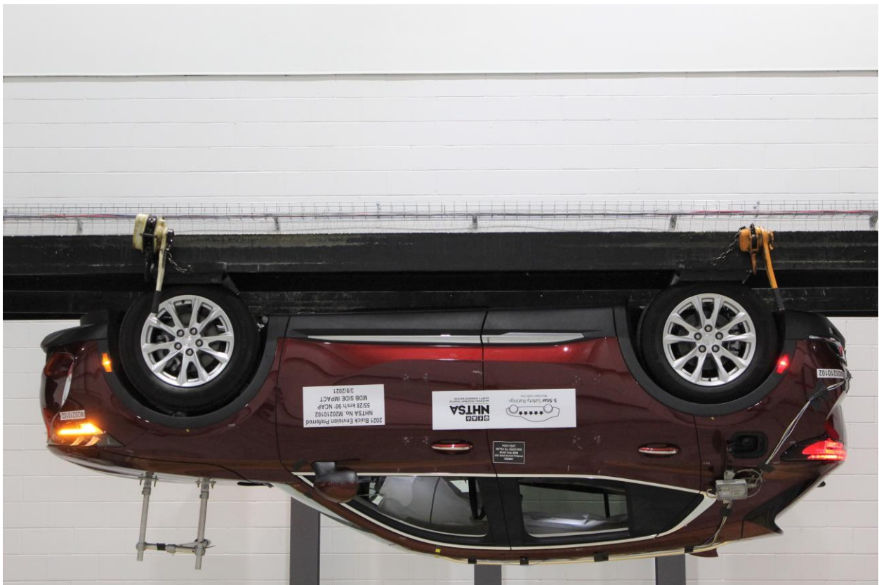
Figure A-98: FMVSS No. 301 Static Rollover 180 Degrees
