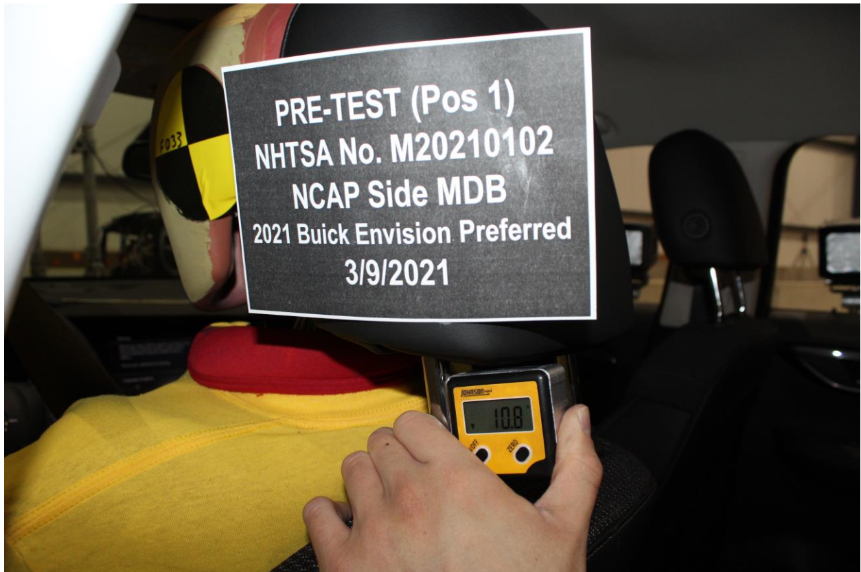
Figure A-41: Pre-Test Close-Up View of Driver Seat Back or Head Restraint
