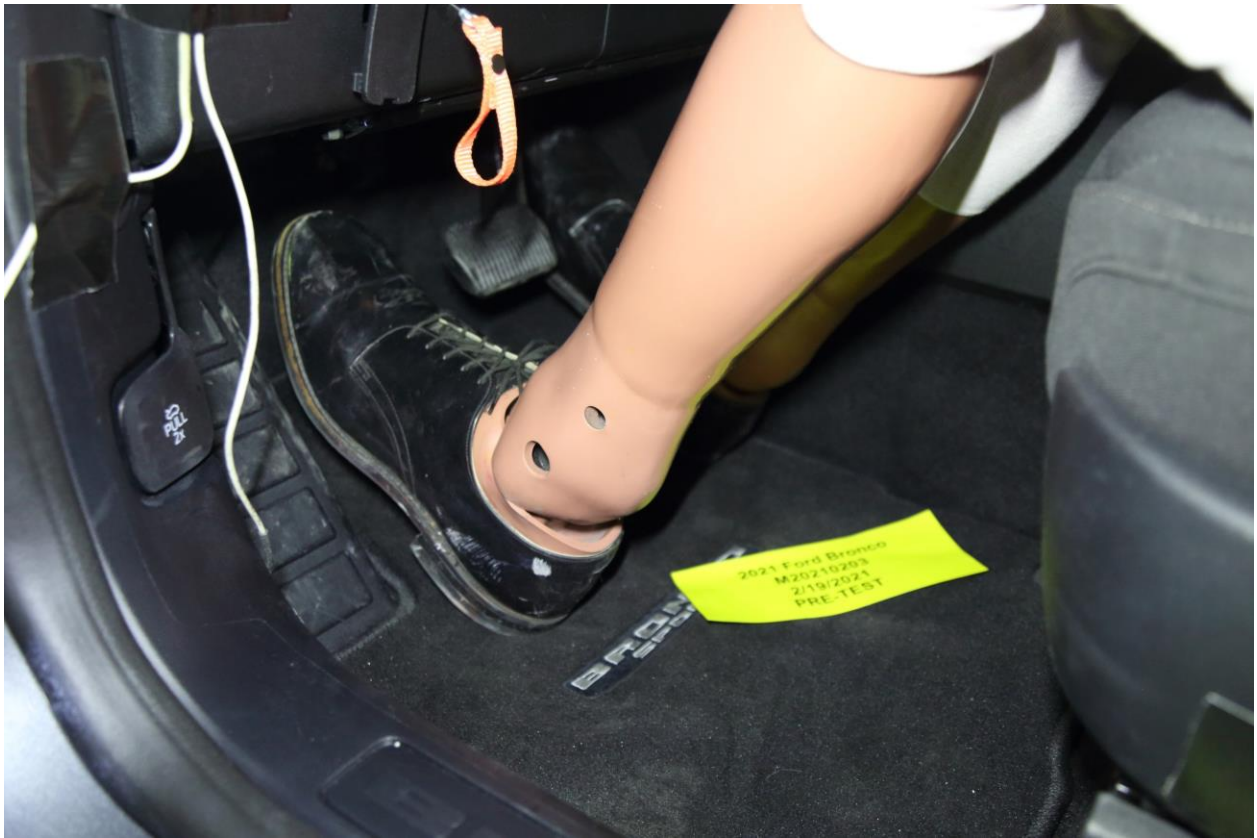
034 Pre-Test Placement of Driver's Dummy Feet
