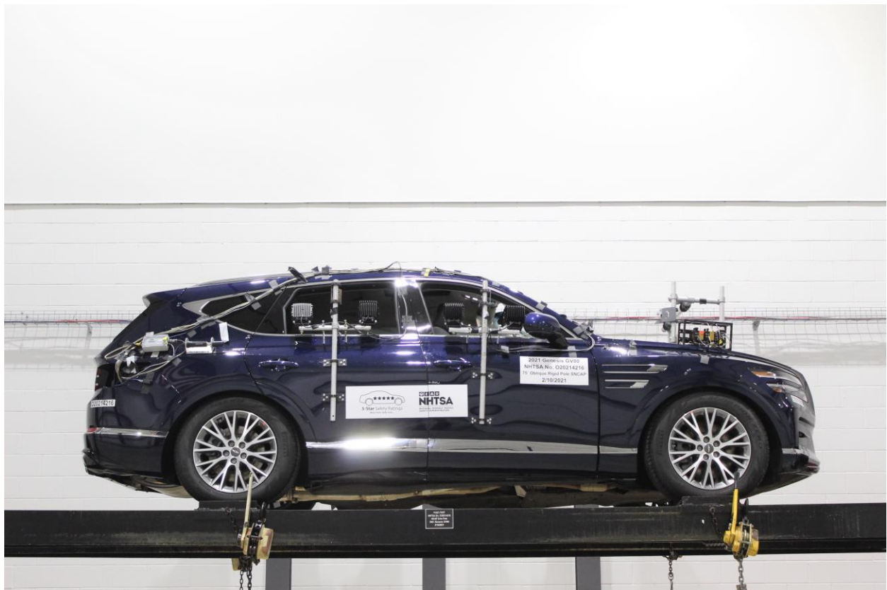
Figure A-69: FMVSS No. 301 Static Rollover 360 Degrees
