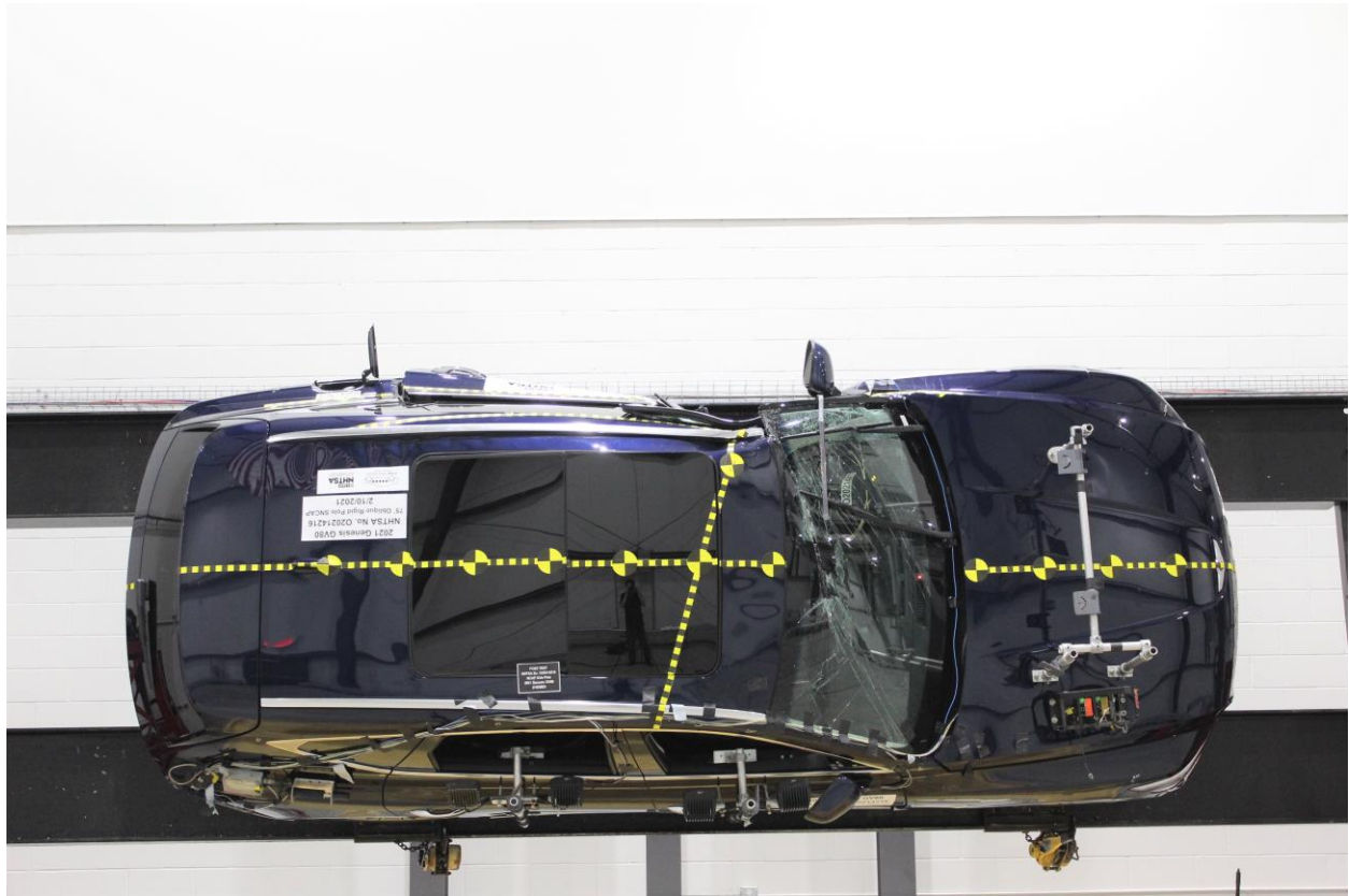
Figure A-68: FMVSS No. 301 Static Rollover 270 Degrees
