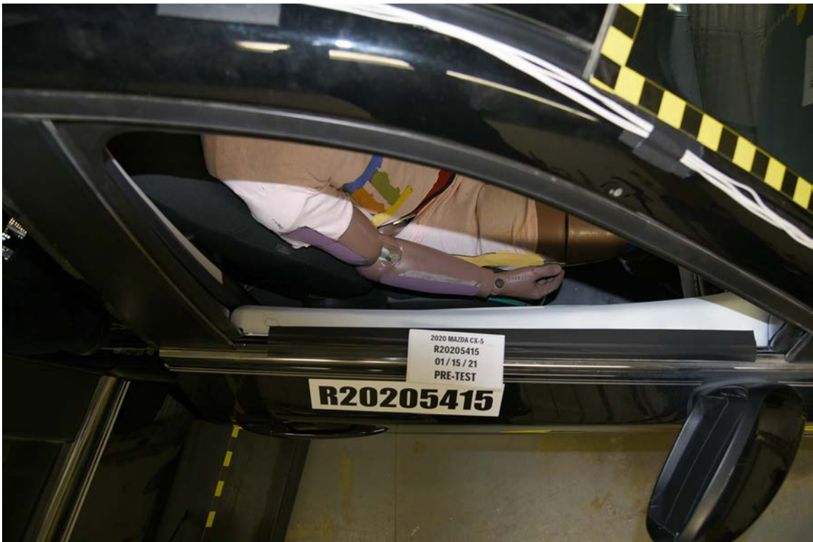
FIGURE 96. Pre-Test View of Passenger Door Clearance
