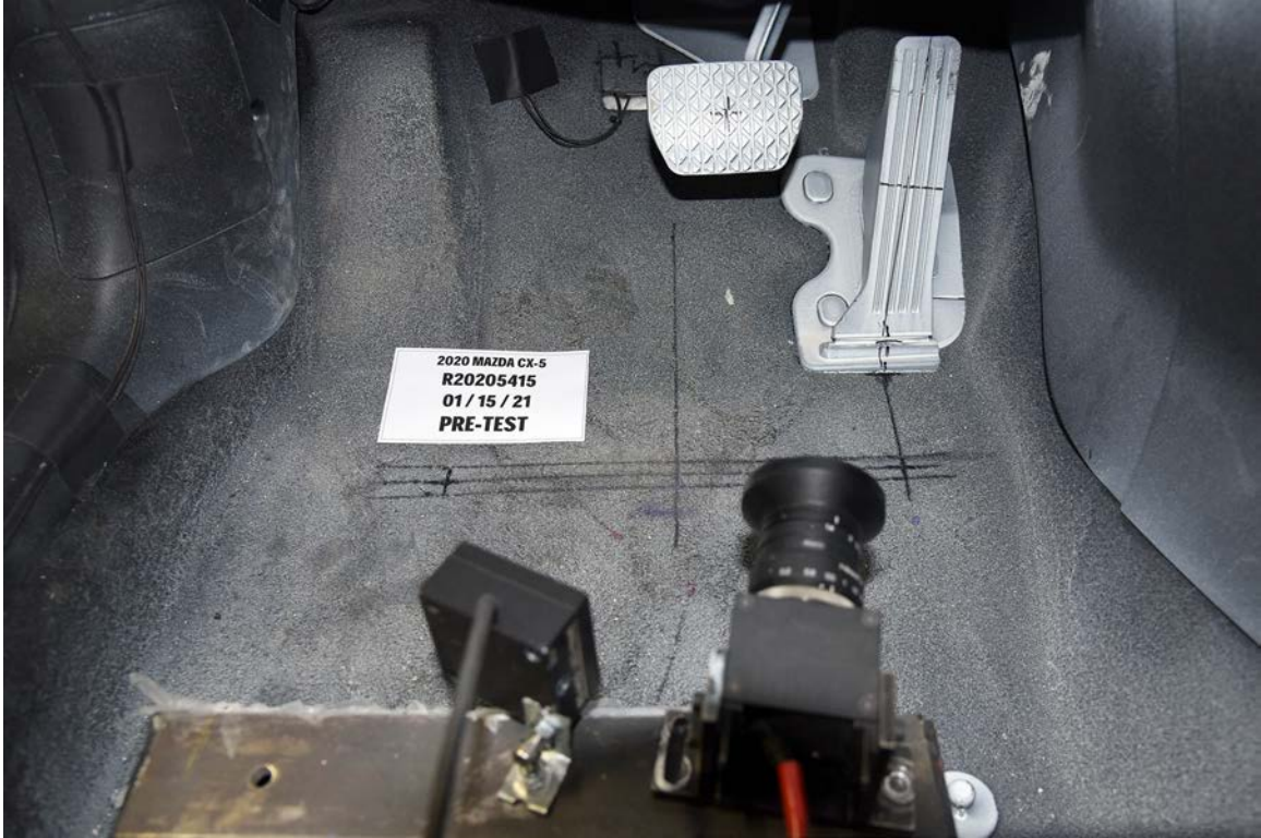
FIGURE 85. Pre-Test View of Driver Floor Pan from Top of Seat
