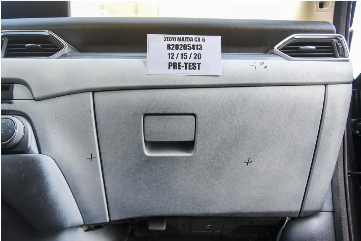
FIGURE 124. Pre-Test Center View of Passenger Knee Bolster
