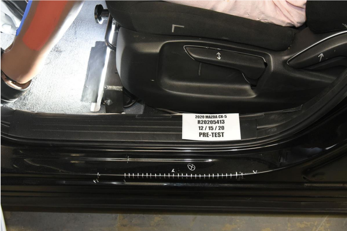
FIGURE 69. Pre-Test Driver Seat Fore-Aft Markings
