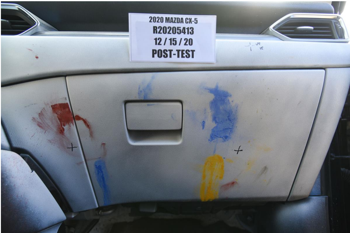
FIGURE 125. Post-Test Center View of Passenger Knee Bolster
