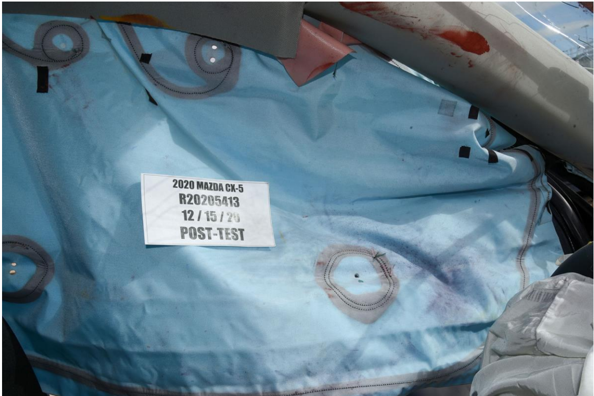
FIGURE 90. Post-Test Driver Dummy Contact with Side Airbag
