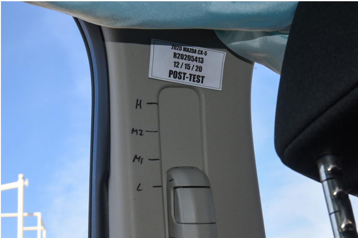
FIGURE 68. Post-Test Driver Adjustable D-Ring
