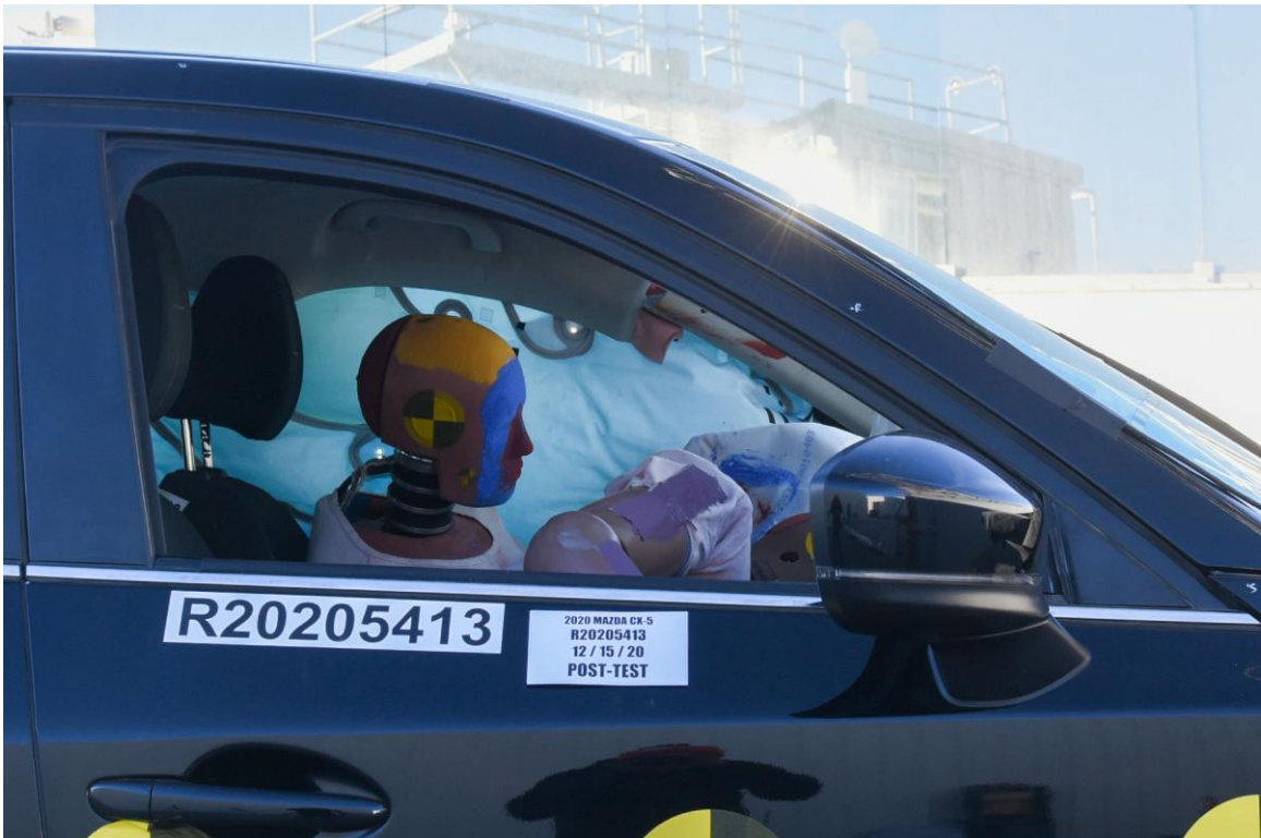
FIGURE 95. Post-Test Passenger Side Front Window View
