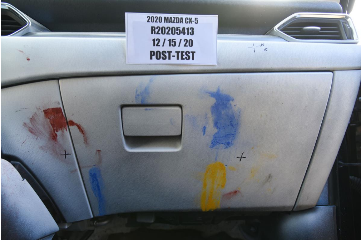
FIGURE 136b. Post-Test Passenger Dummy Contact with Knee Bolster
