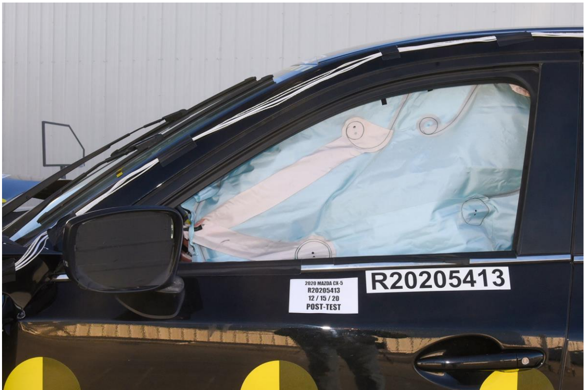
FIGURE 46. Post-Test Driver Side Front Window View
