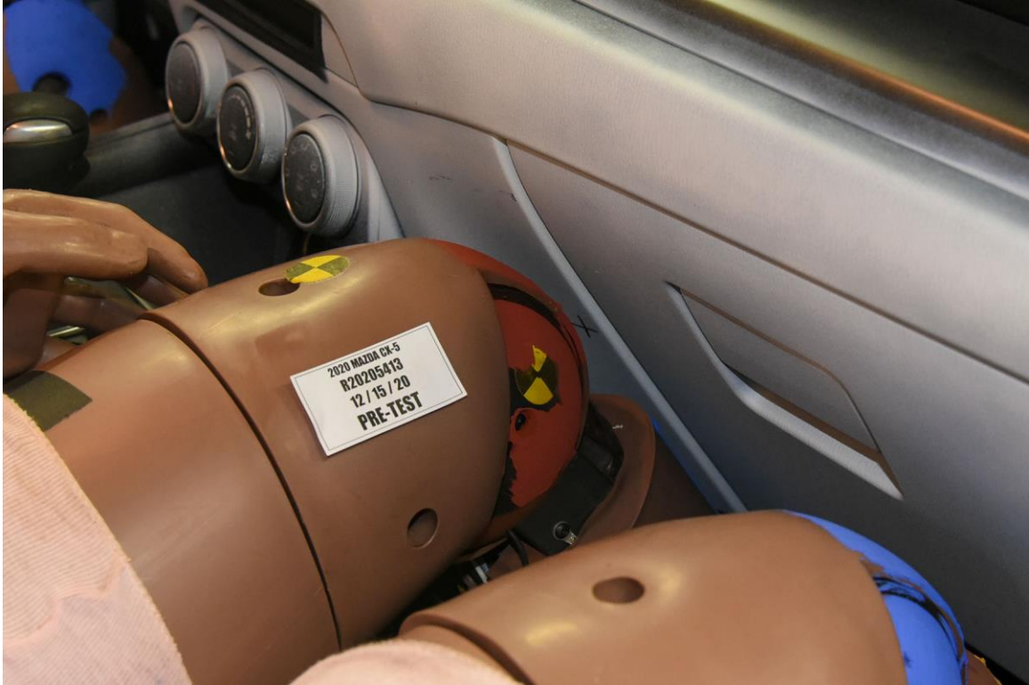
FIGURE 108. Pre-Test View of Passenger Left Knee and Bolster
