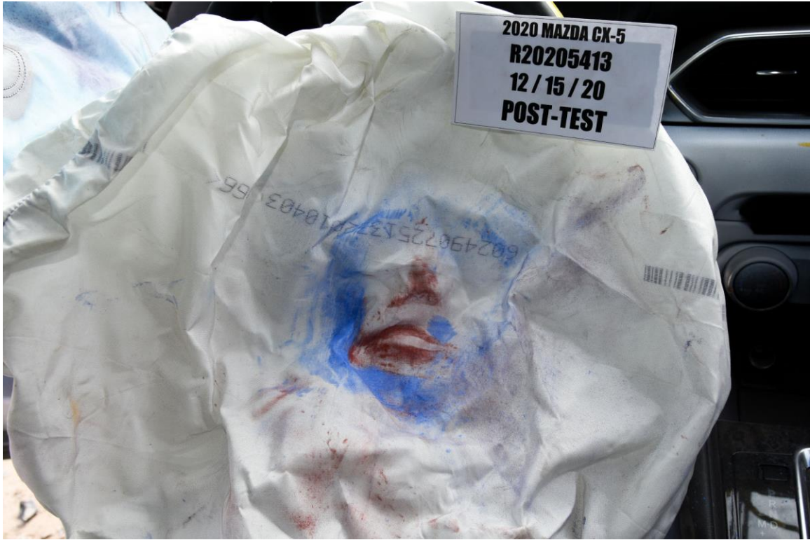
FIGURE 89. Post-Test Driver Dummy Contact with Front Airbag
