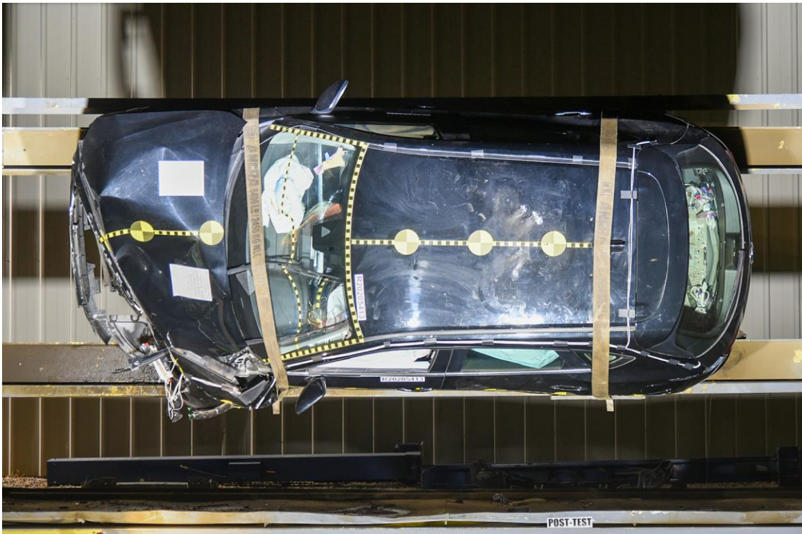
FIGURE 141. Vehicle at 90° on Static Rollover Device
