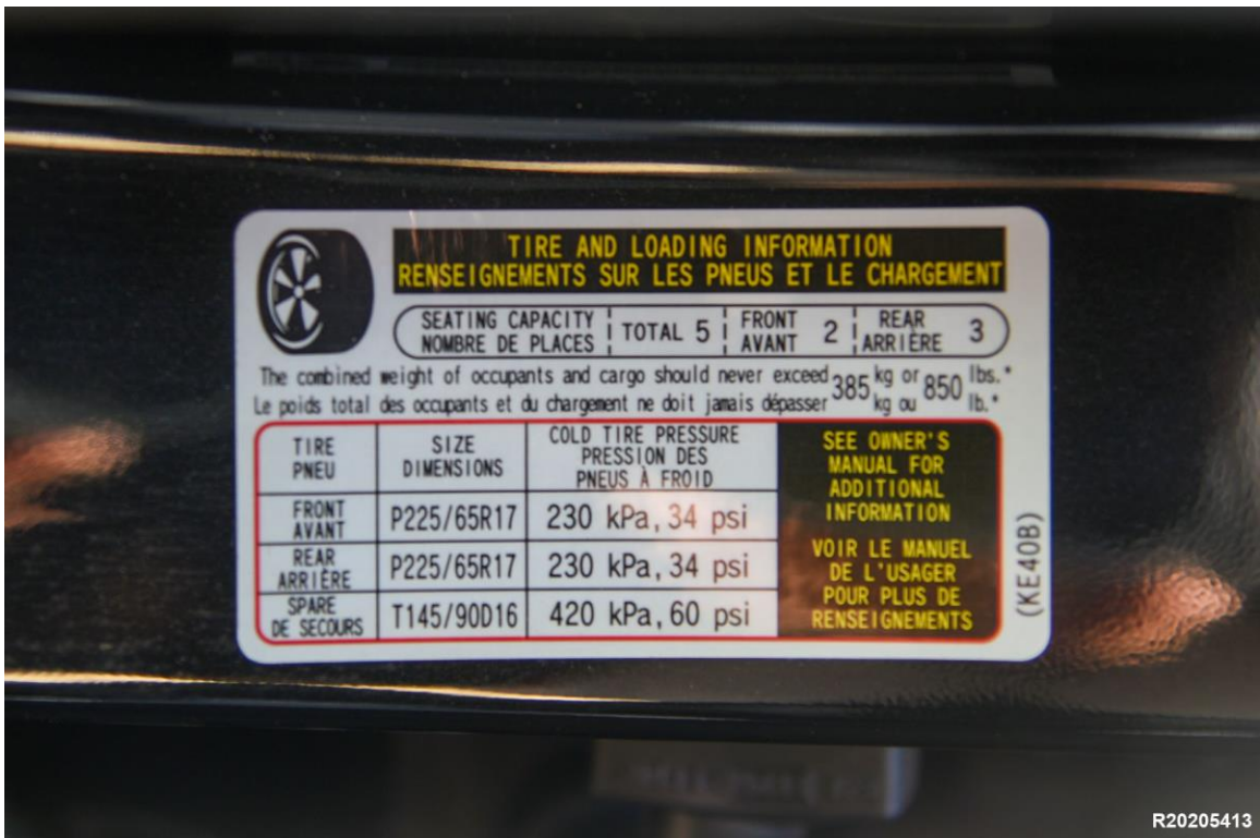
FIGURE 2. Test Vehicle Tire Placard
