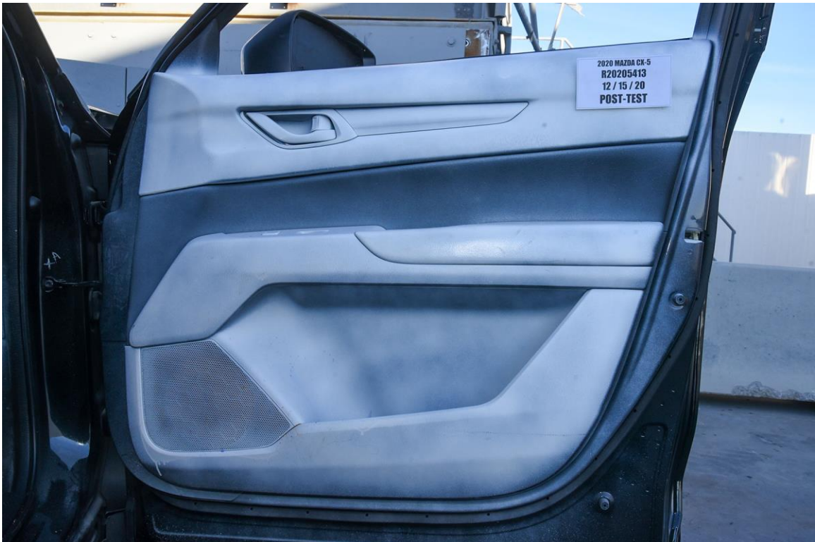
FIGURE 121. Post-Test Passenger Inner Door Panel
