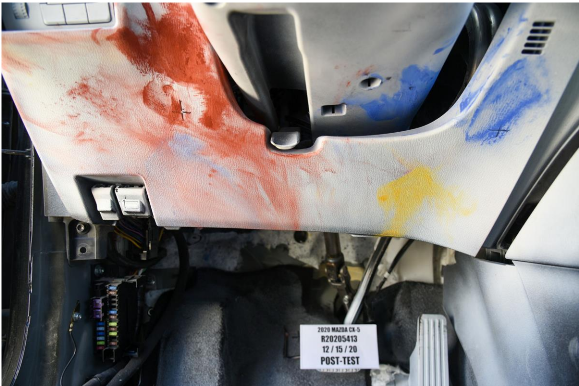
FIGURE 80. Post-Test Overall View of Driver Knee Bolster
