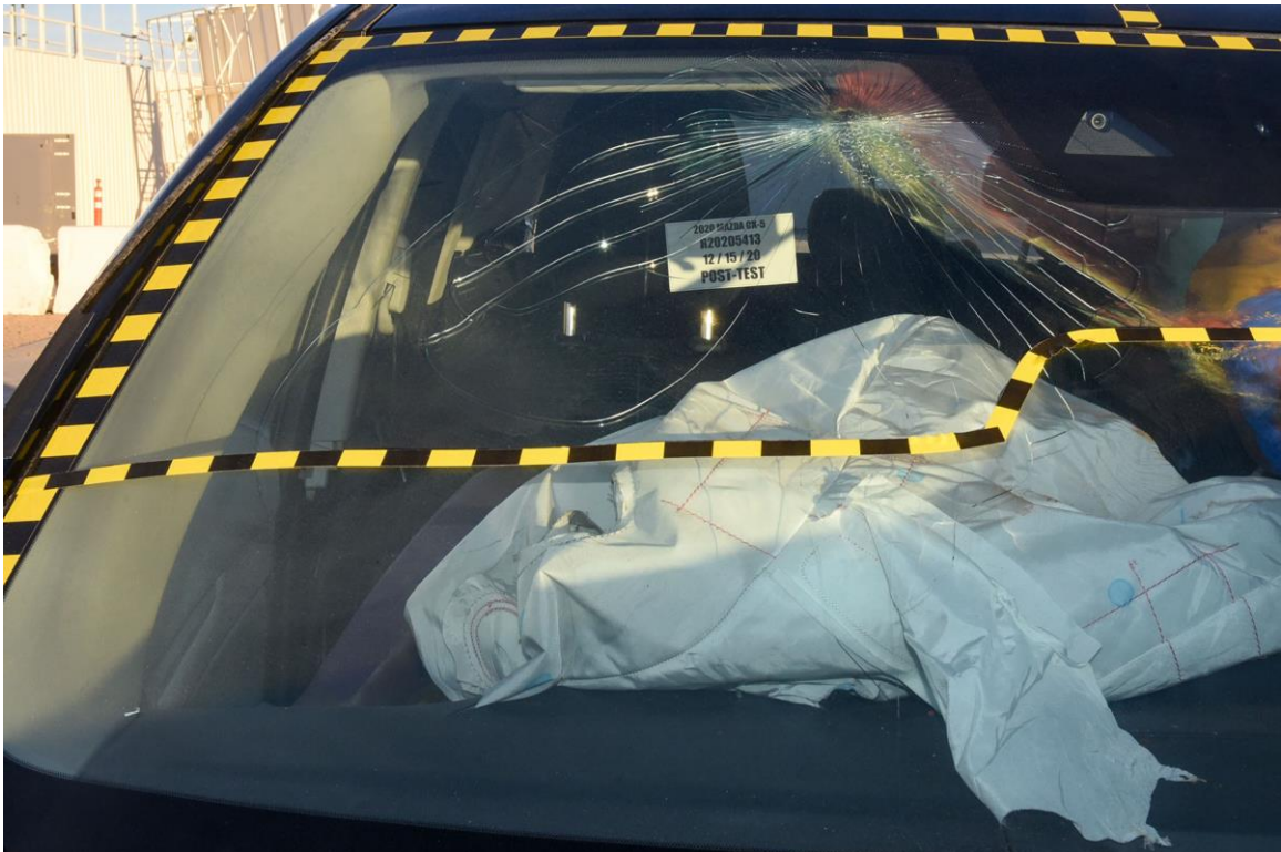
FIGURE 93. Post-Test Passenger Front Windshield View
