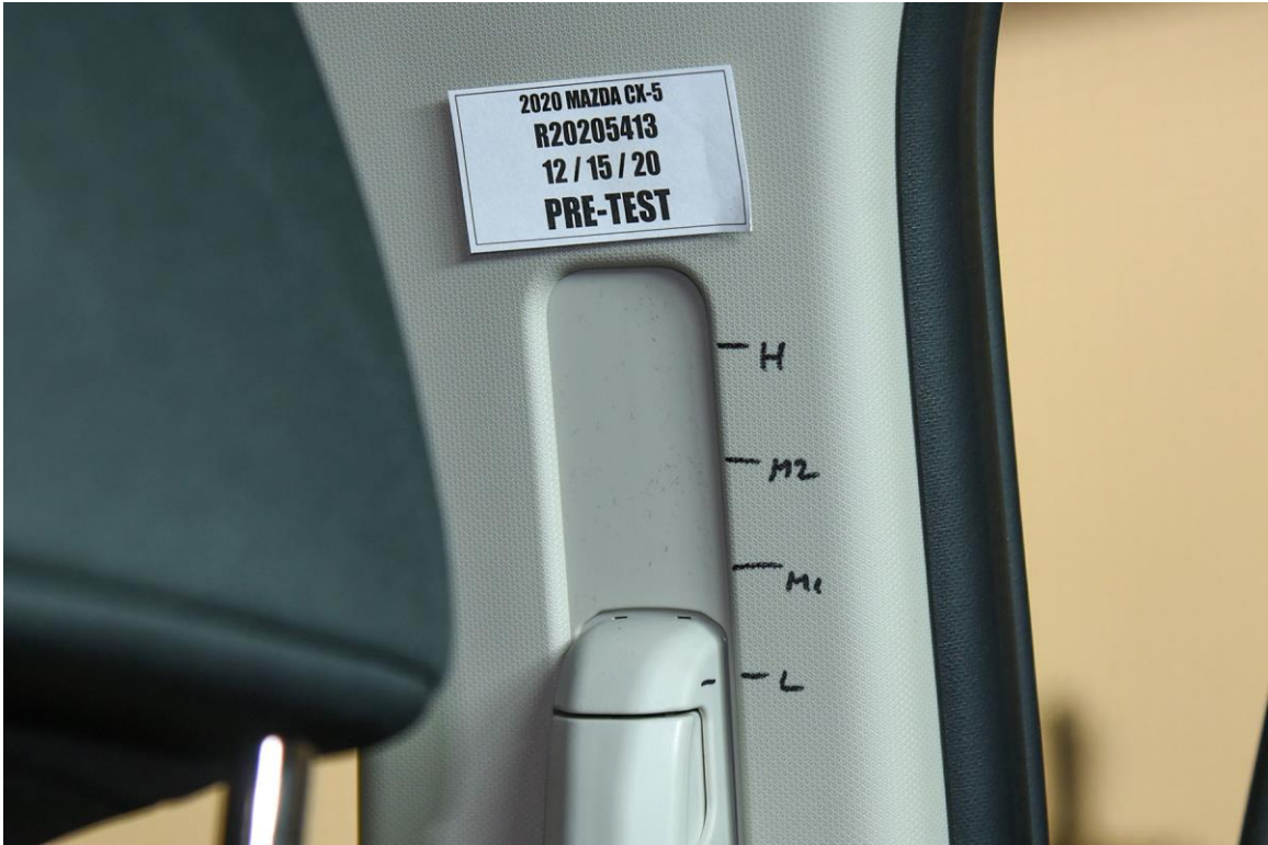
FIGURE 112. Pre-Test Passenger Adjustable D-Ring
