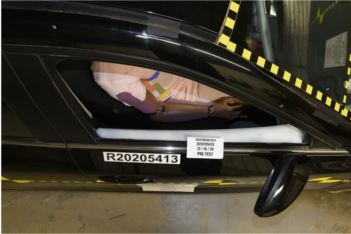
FIGURE 96. Pre-Test View of Passenger Door Clearance
