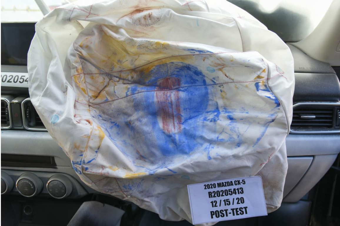
FIGURE 134. Post-Test Passenger Dummy Contact with Front Airbag
