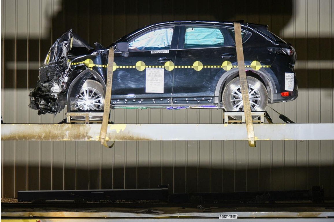
FIGURE 140. Vehicle at 0° on Static Rollover Device
