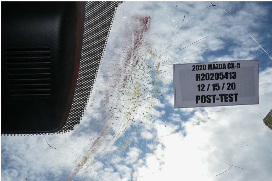
FIGURE 136a. Post-Test Passenger Dummy Contact with Windshield
