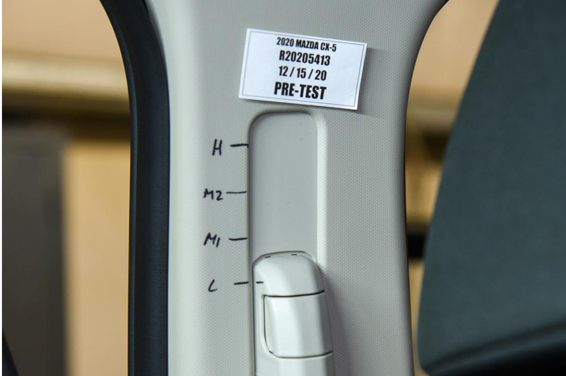
FIGURE 67. Pre-Test Driver Adjustable D-Ring
