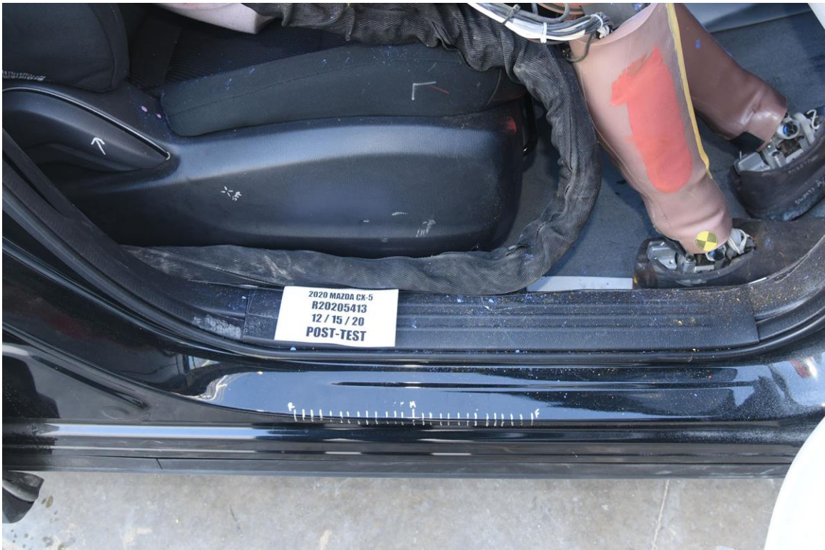
FIGURE 115. Post-Test Right Front Passenger Seat Fore-Aft Markings
