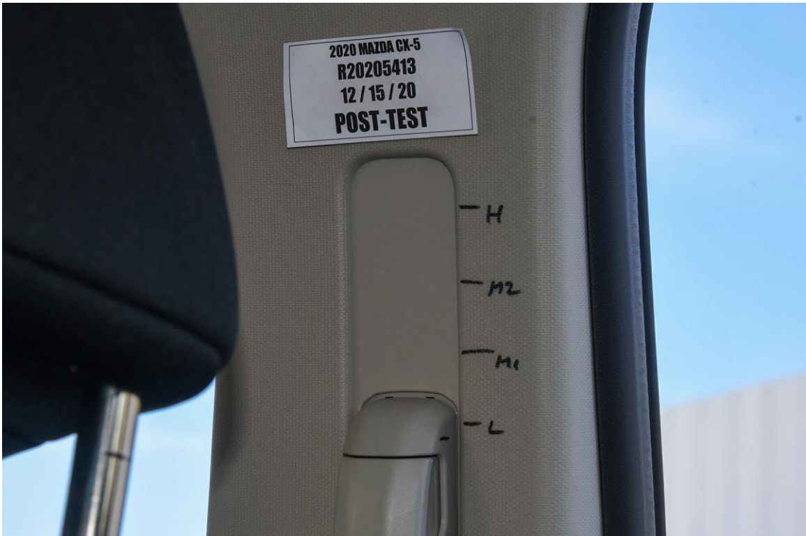
FIGURE 113. Post-Test Passenger Adjustable D-Ring
