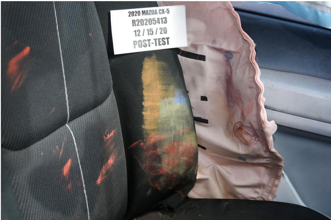
FIGURE 91e. Post-Test Driver Dummy Contact with Seat
