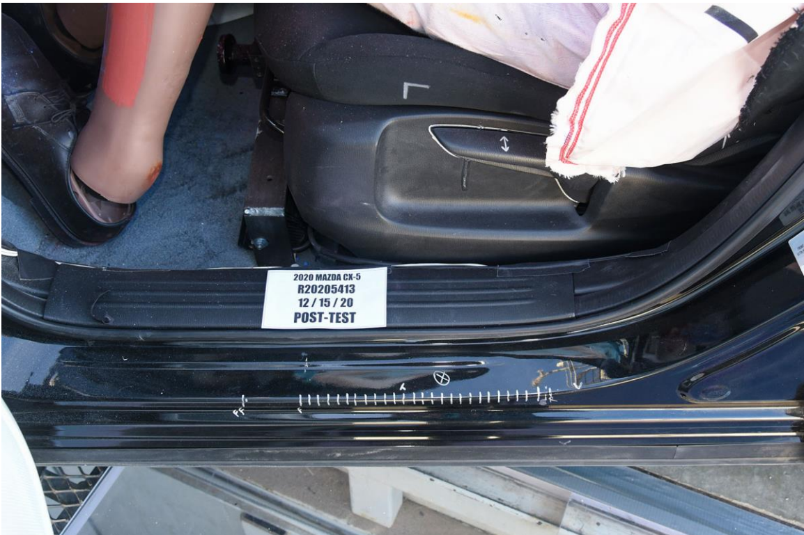
FIGURE 70. Post-Test Driver Seat Fore-Aft Markings
