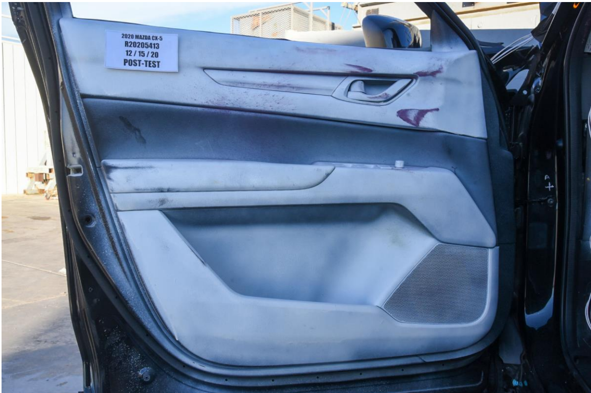
FIGURE 91c. Post-Test Driver Dummy Contact with Door Panel
