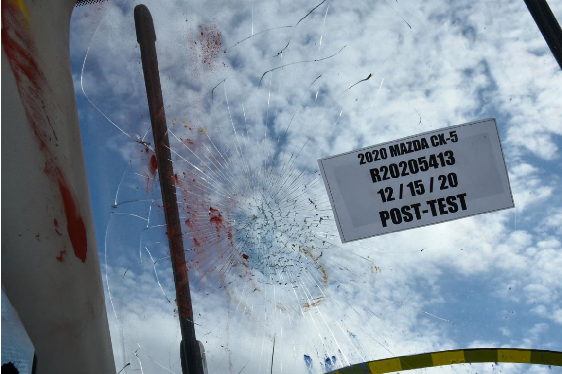
FIGURE 91b. Post-Test Driver Dummy Contact with Windshield
