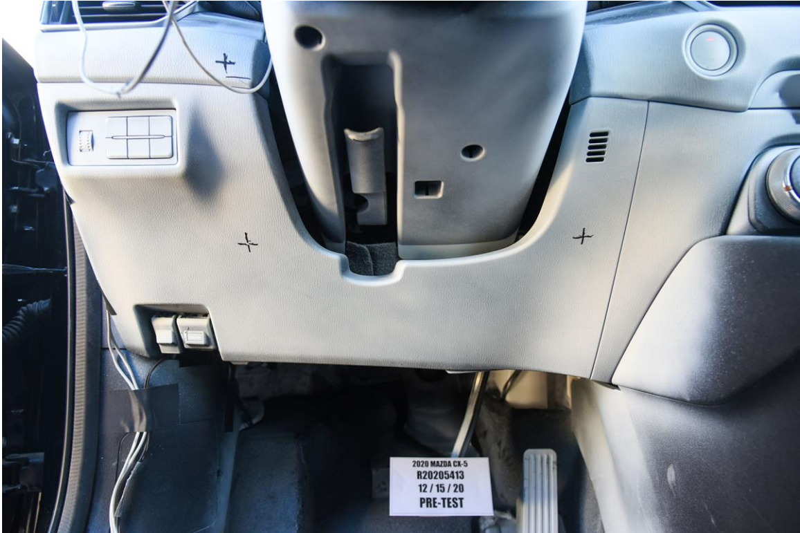
FIGURE 79. Pre-Test Overall View of Driver Knee Bolster
