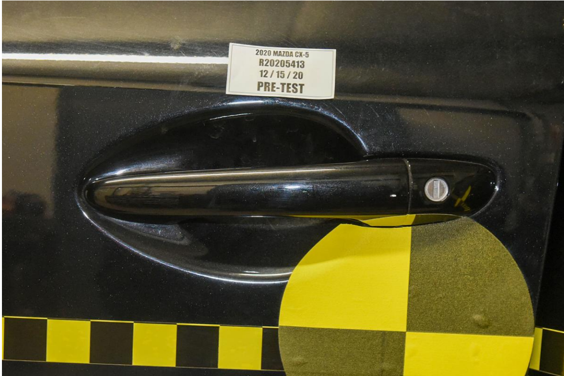
FIGURE 73. Pre-Test Close-Up View of Driver Door Latch
