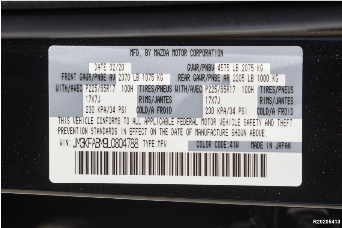
FIGURE 1. Test Vehicle Certification Label
