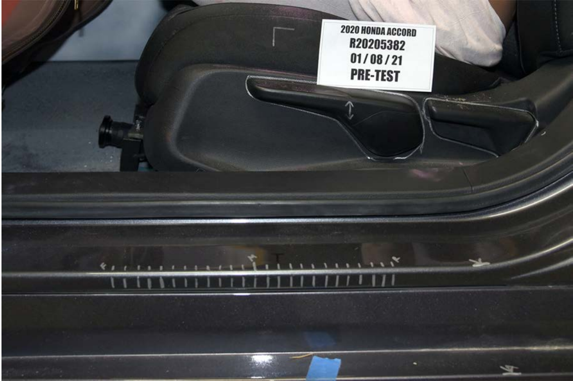
FIGURE 69. Pre-Test Driver Seat Fore-Aft Markings
