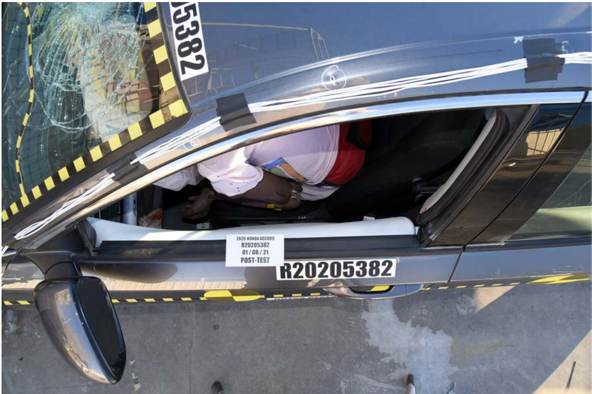
FIGURE 48. Post-Test View of Driver Door Clearance
