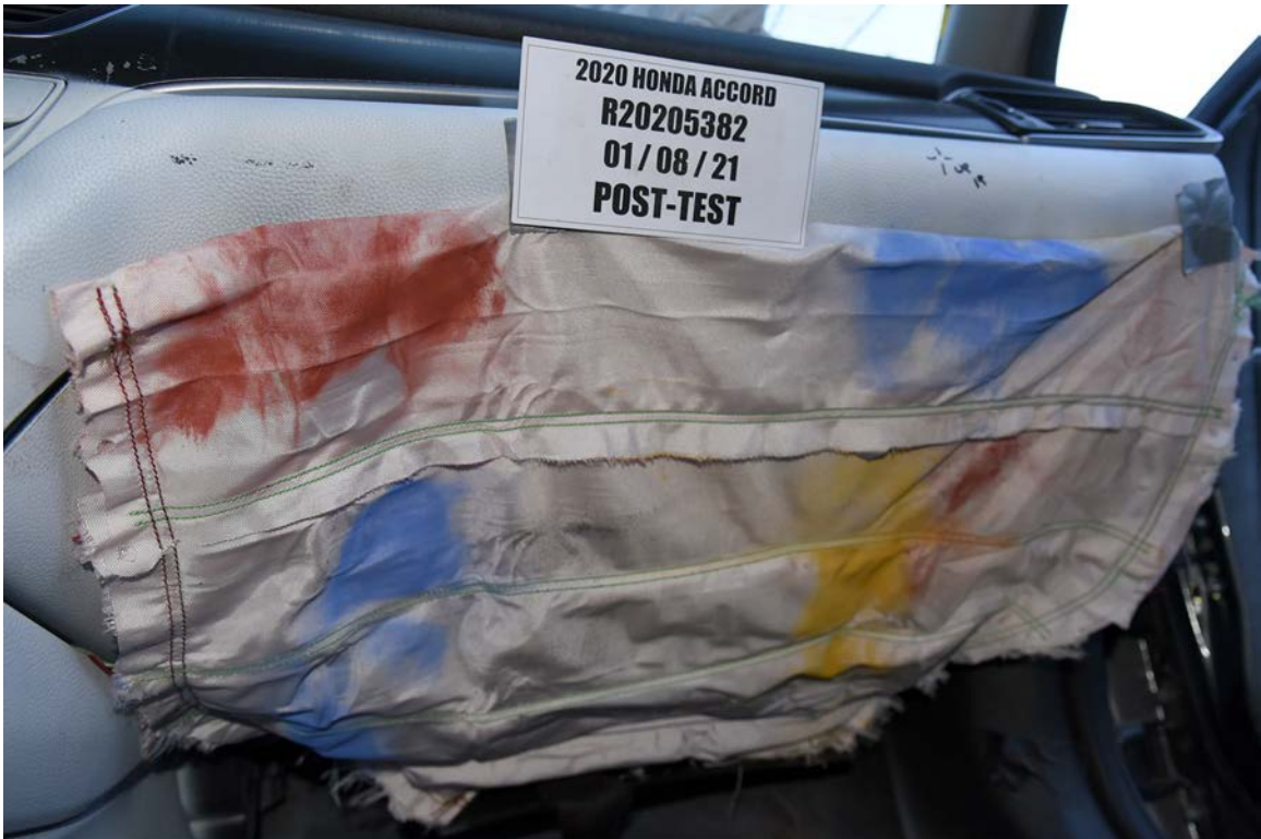
FIGURE 136f. Post-Test Passenger Dummy Contact with Knee Airbag
