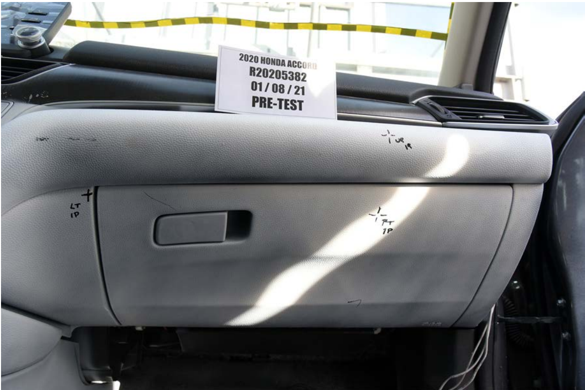
FIGURE 124. Pre-Test Center View of Passenger Knee Bolster
