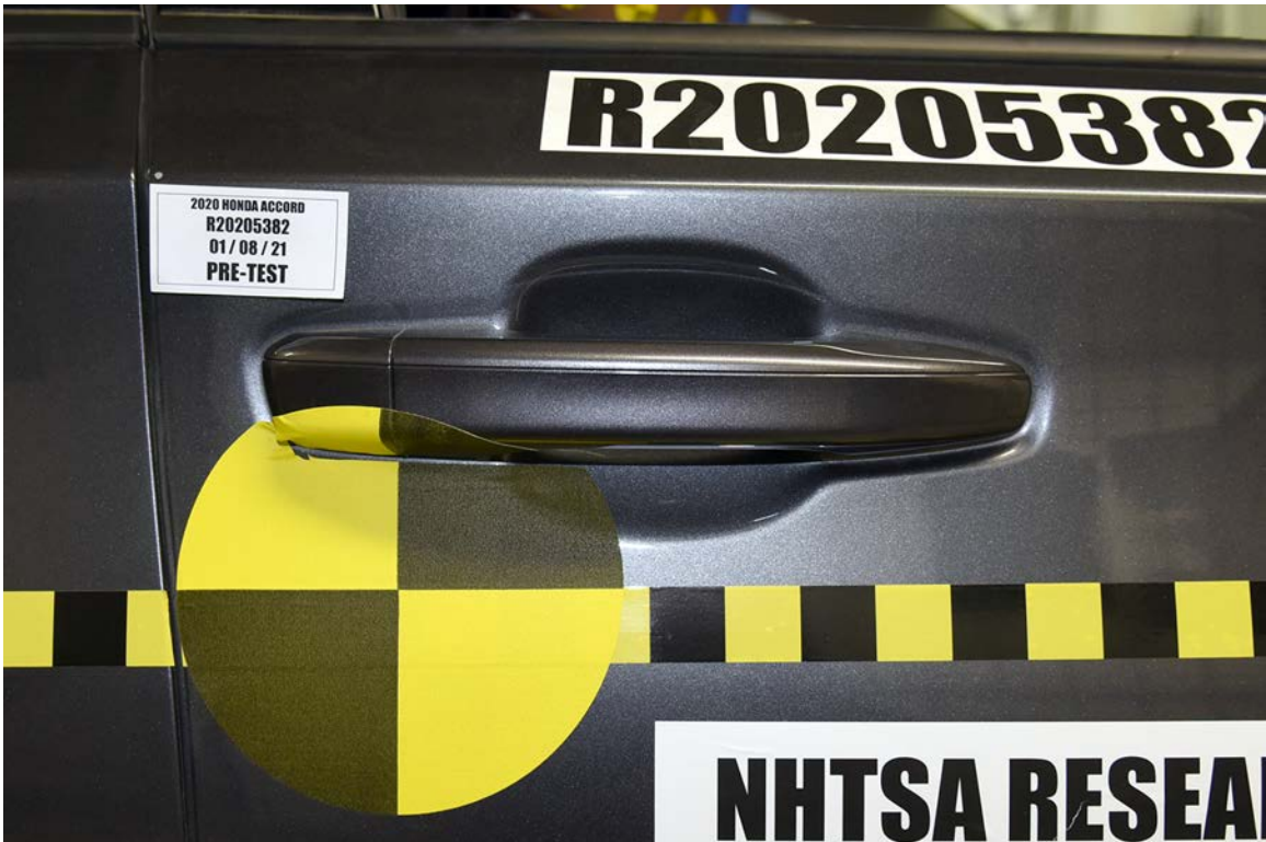
FIGURE 118. Pre-Test Close-up View of Passenger Door Latch
