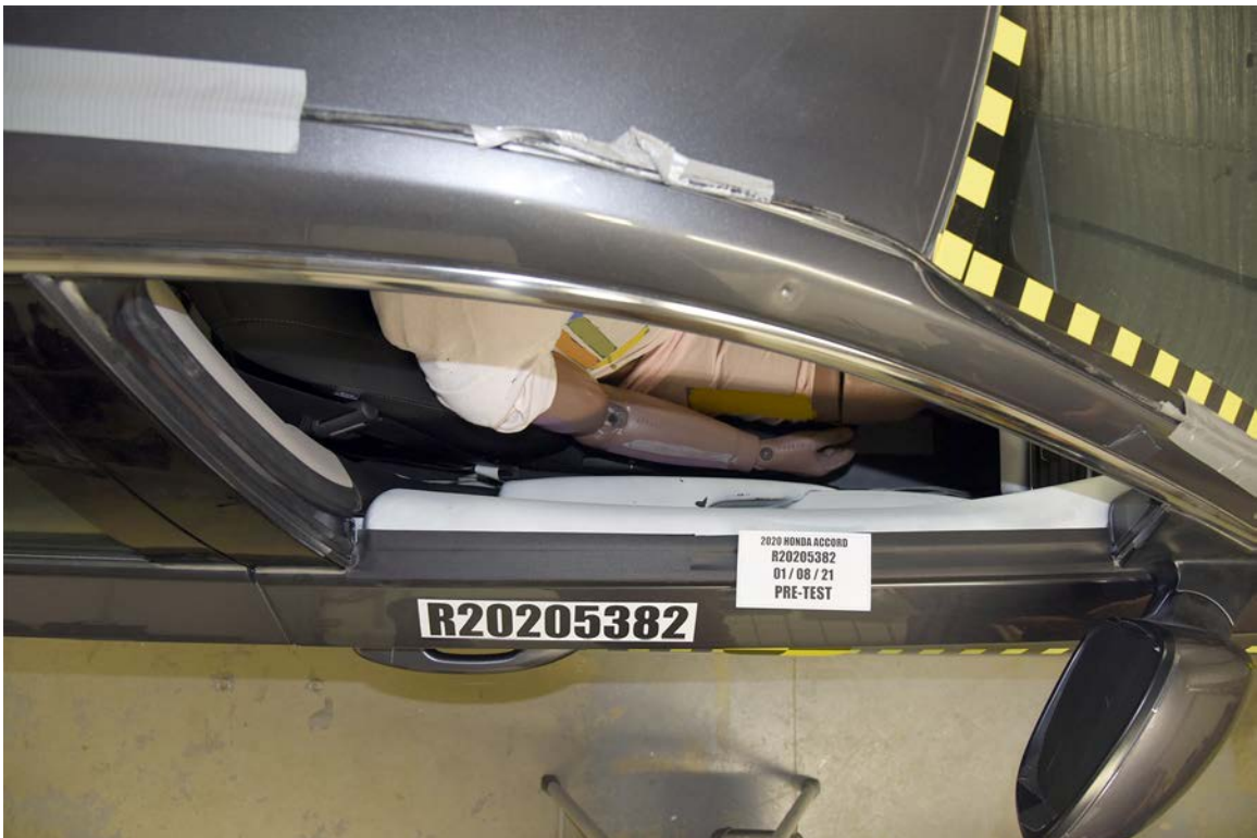
FIGURE 96. Pre-Test View of Passenger Door Clearance
