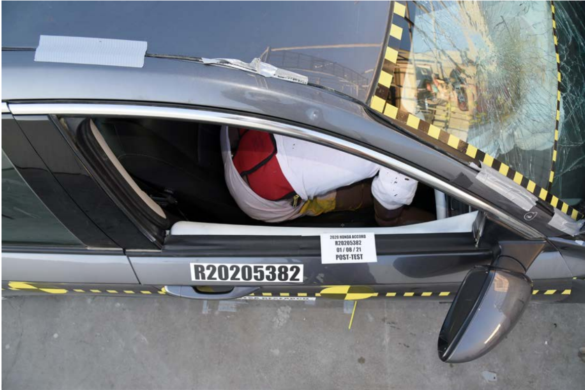
FIGURE 97. Post-Test View of Passenger Door Clearance
