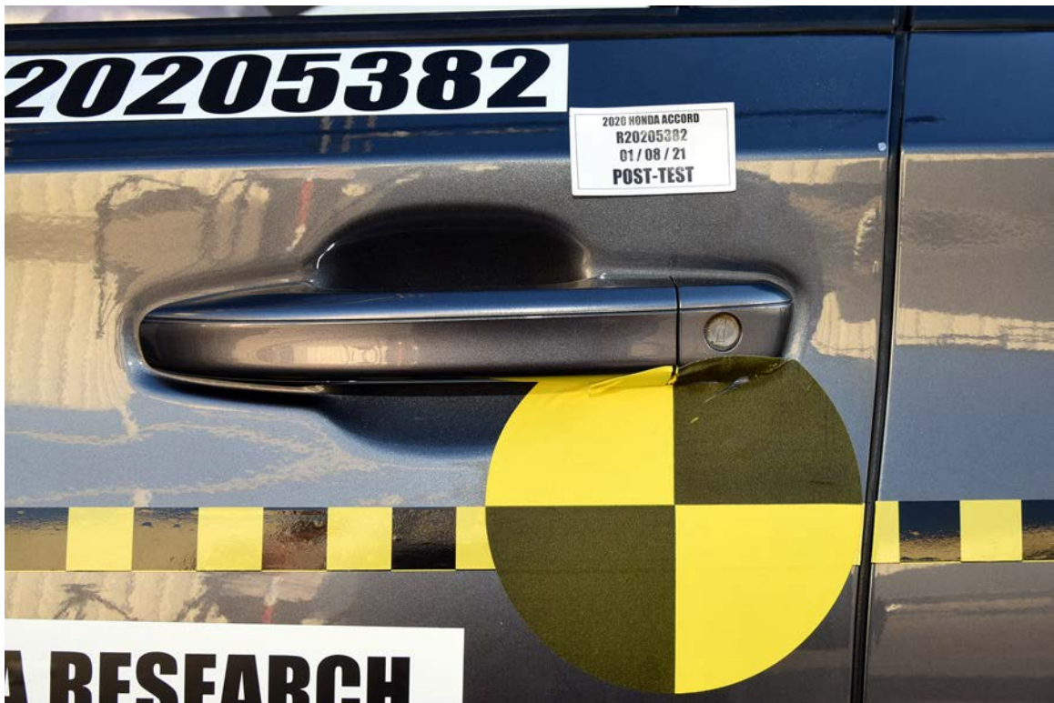
FIGURE 74. Post-Test Close-Up View of Driver Door Latch
