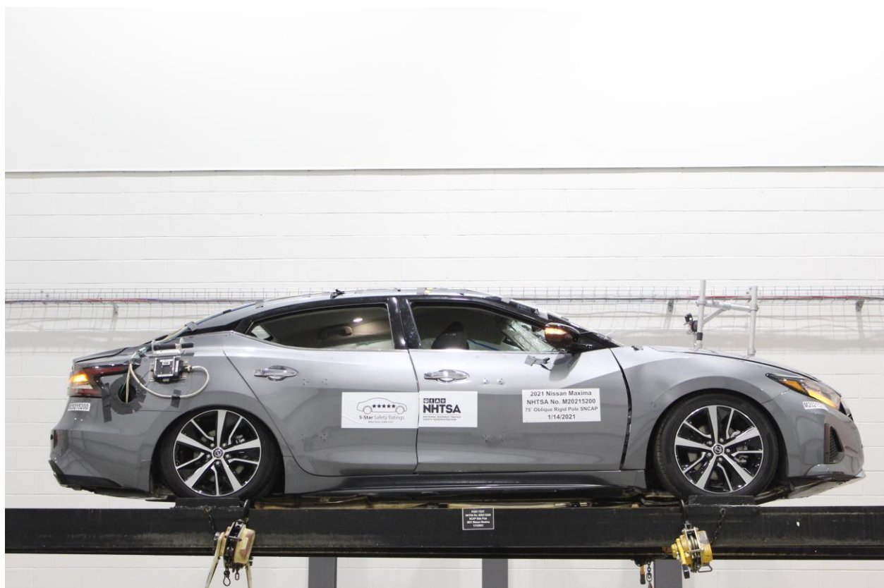
Figure A-63: FMVSS No. 301 Static Rollover 0 Degrees
