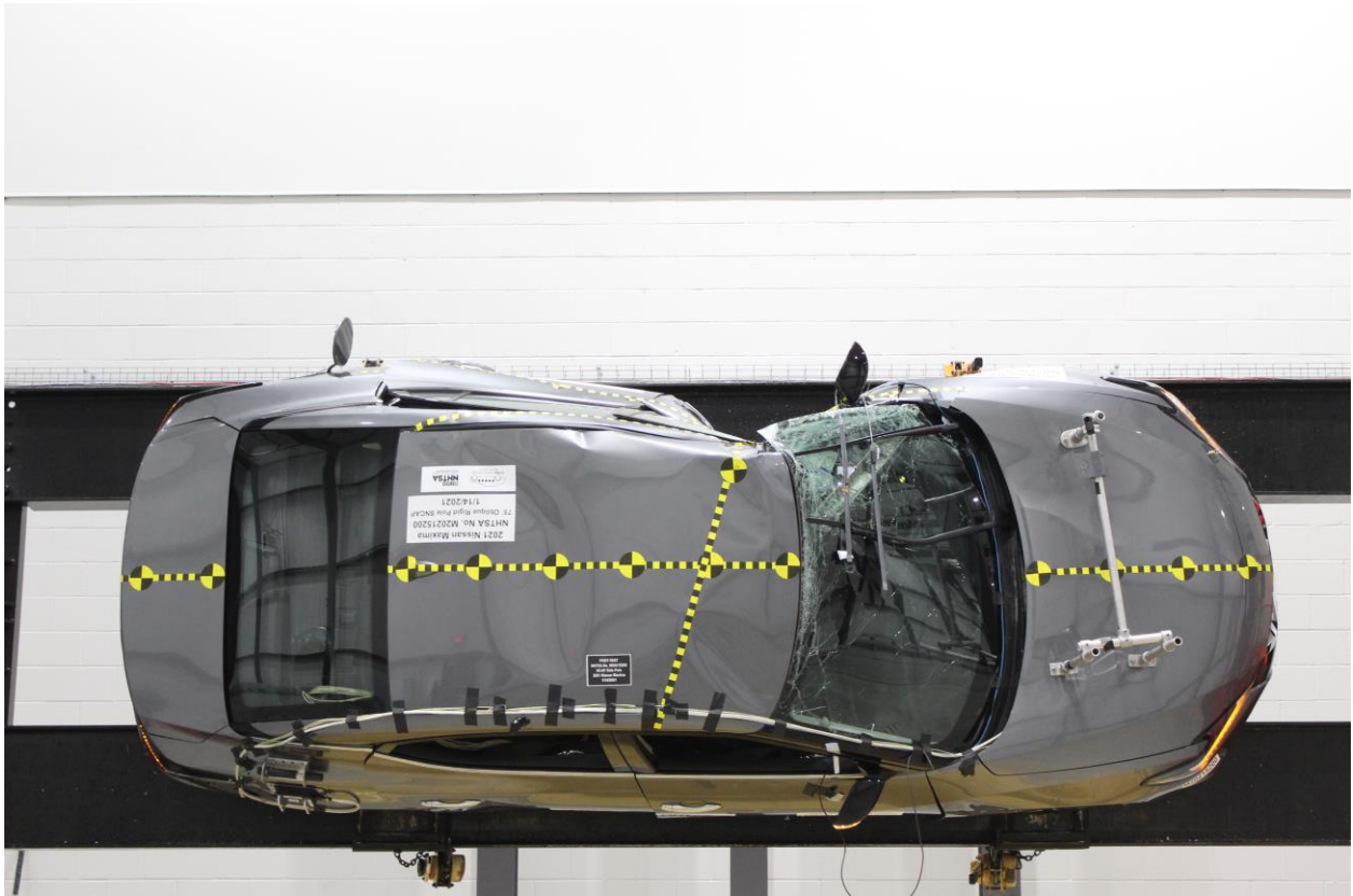
Figure A-66: FMVSS No. 301 Static Rollover 270 Degrees
