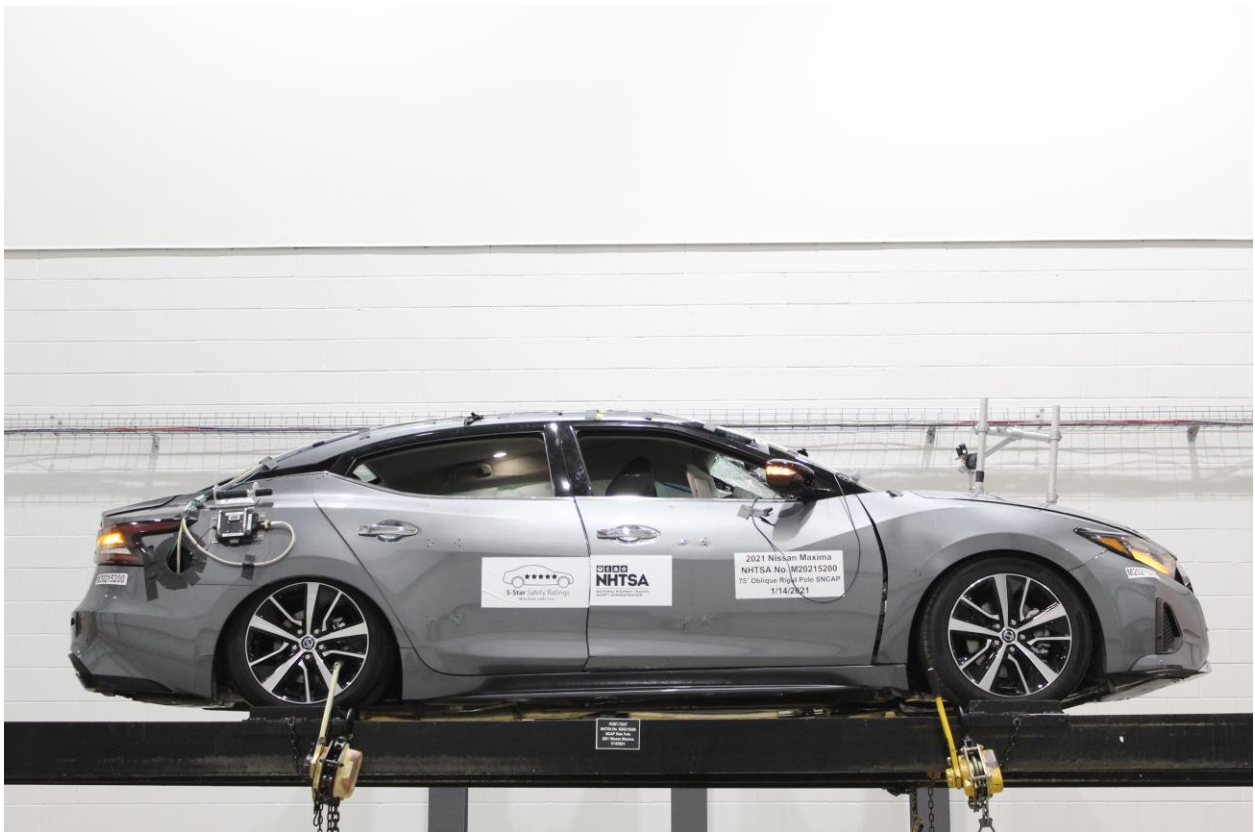
Figure A-67: FMVSS No. 301 Static Rollover 360 Degrees
