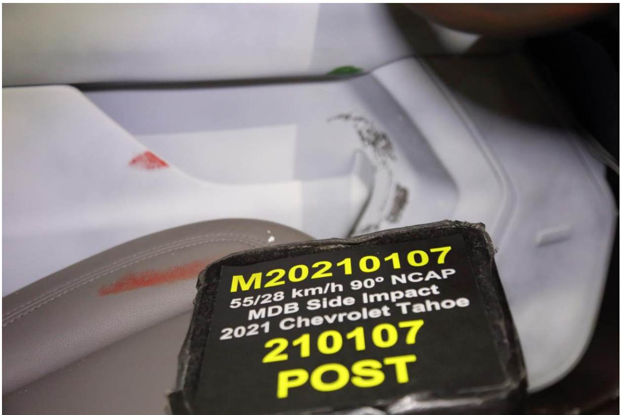
054 Post-Test Driver Dummy Close-Up Knee Contact View
